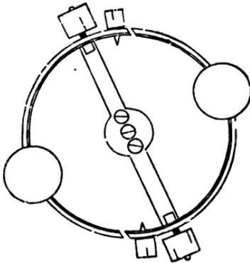
FIG. 131.—Marine chronometer balance.
