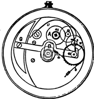
FIG. 149.—Pedometer winding.
