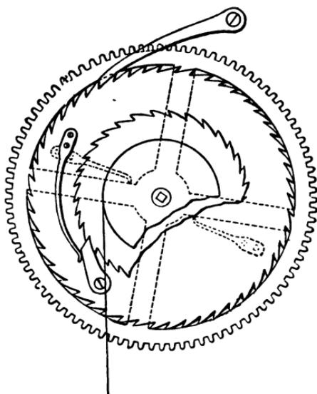
Fig. 181.—Maintaining power for weight clock.
