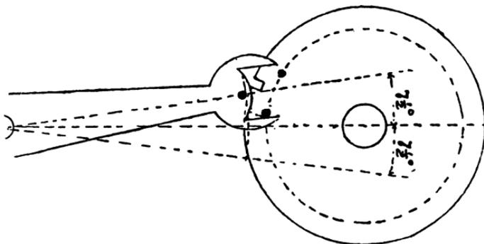
FIG. 166.—Savage's two-pin escapement.
