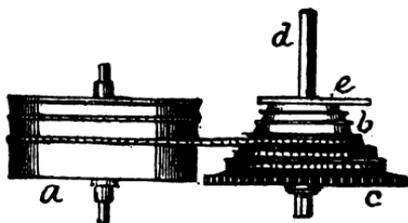
FIG. 22.—Mainspring barrel and fusee.
