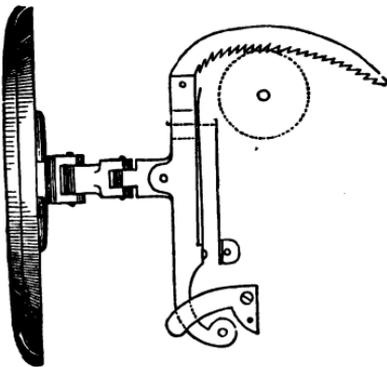
FIG. 148.—Self-winding watch mechanism to act on the closing of the hunting cover.
