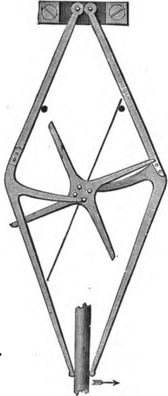
FIG. 159.—Four-legged gravity escapement.
