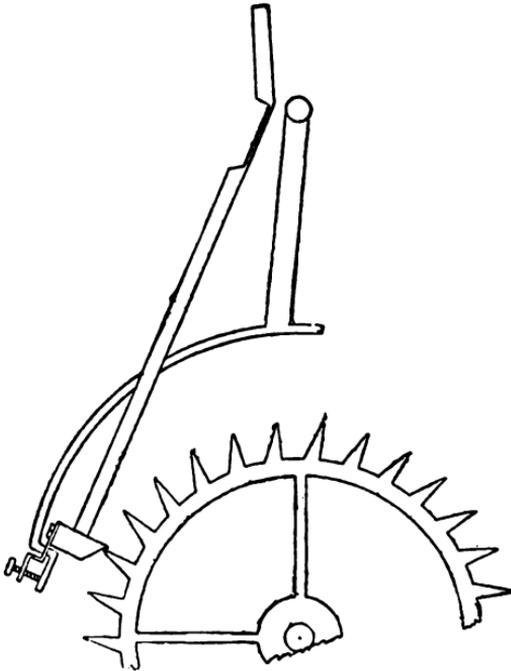
FIG. 158.—Reid's gravity escapement.
