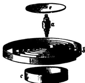
FIG. 20.—Mainspring and barrel.
