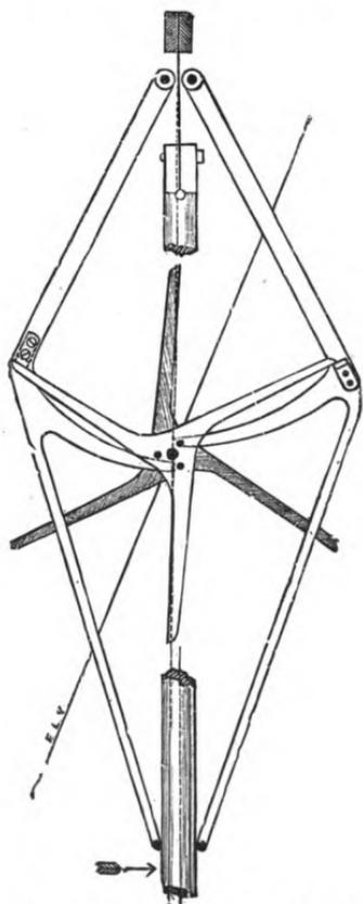
FIG. 156.—Double three-legged gravity escapement.
