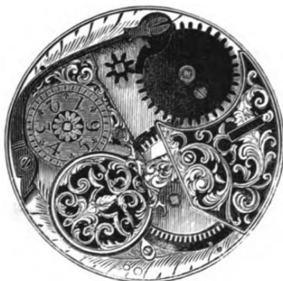
FIG. 21.—Watch movement with "stackreed."
