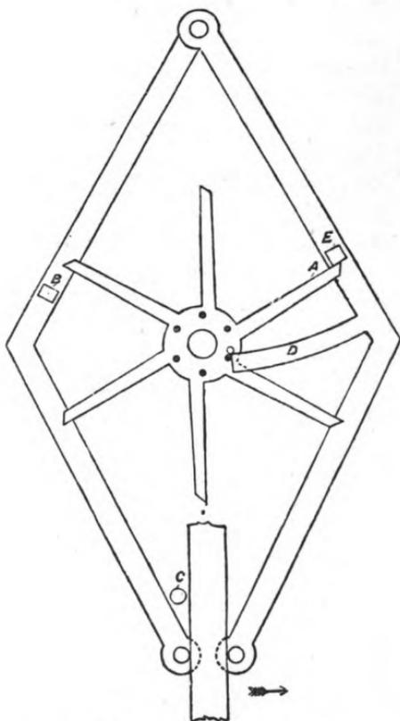
FIG. 157.—Thwaites and Reed's six-legged gravity escapement.
