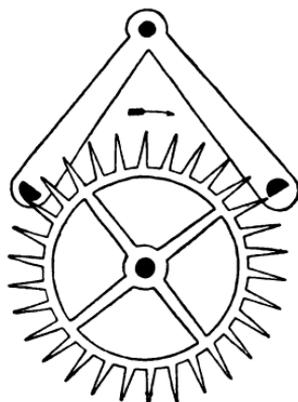
FIG. 155.—Pin pallet escapement.
