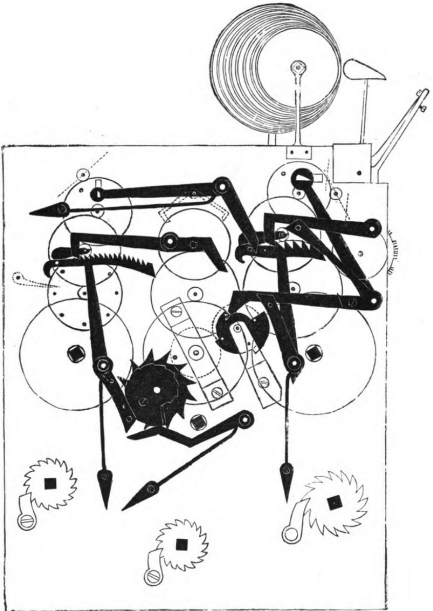
FIG. 126.—Striking mechanism of quarter-chime clock.
