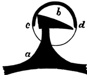
FIG. 162.—Plan of cylinder and one tooth of escape wheel therein.
