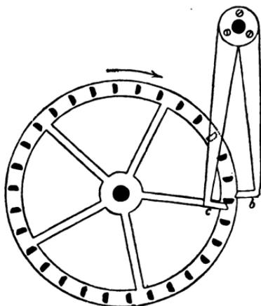
FIG. 154.—Pin wheel escapement.
