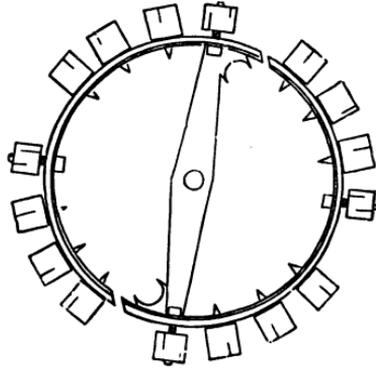
FIG. 132.—Compensation balance for watches.
