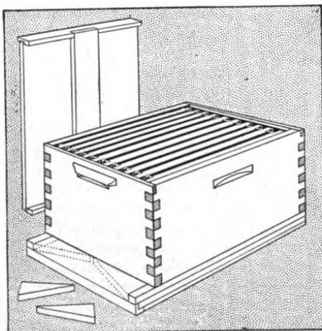
Fig. 52—"Dovetailed" or Lock-Cornered Hive
