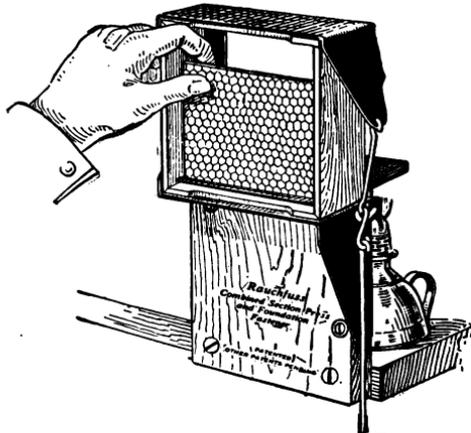
Fig. 94—The Rauchfuss Combined Section Press and Foundation Fastener.
