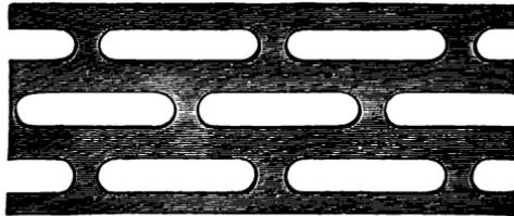
Fig. 110—Shows the Exact Size of Zinc Perforations.
