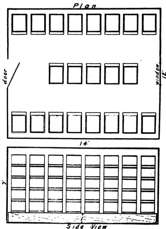
Fig. 127--Plan of Bee Cellar. 100 hives in a space 12 x 14.
