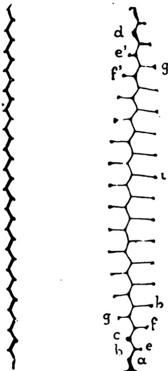
Fig. 87—Cross-Section of a sheet of Foundation—Natural size.
