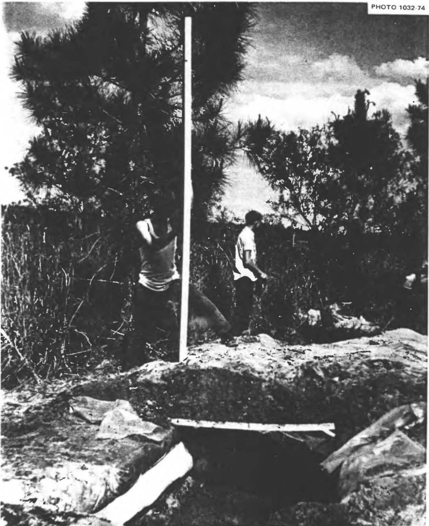
Fig. 5.60. The painted hollow-core door previously pictured, soon after it had been uncovered and removed from the walls made of rolls. Note how slight was its permanent warp or bow.
