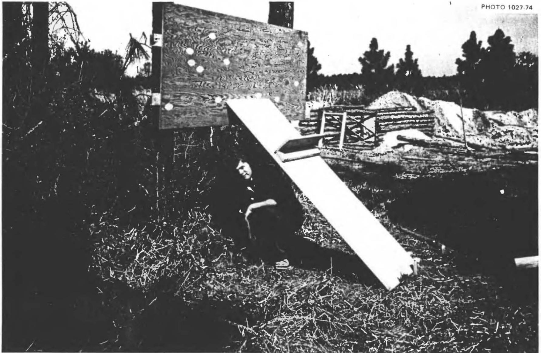
Fig. 5.63. Preparing to test a hollow-core interior door used as a roof door of an expedient Tilt-Up Shelter, built following instructions received from Donald A. Bettge, DCPA. The plywood (that was nailed to the horizontal 2 × 4s connecting the two pine trees) represented the side of a house. The door slopes 45° and is secured at its base by stakes.
