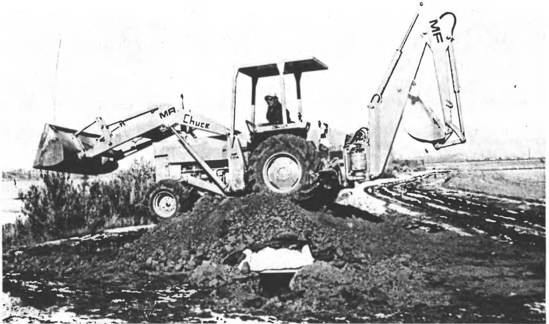
Fig. 3.3. An 8-ton backhoe on top of what was originally the  $6\frac{1}{2}$ -ft-deep pile of earth over the shelter. Before this picture was taken, this machine had been driven back and forth several times over the mounded earth. The roofing doors remained undamaged, and were not observed to be bowed downward any more than when only the  $6\frac{1}{2}$ -ft mound of earth was over them.
