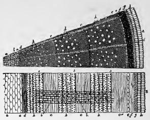
Fig. 1.—Diagram of a stem with a cambium layer. A, section cut across the bundles; B, section in the direction of the bundles; 1, 2, 3, first, second, and third annual rings; a, a, pith; b, b, pitted vessels; c, c, wood-cells; d, spiral vessels, found only in the first annual ring; e, cambium-cells; f, g, h, layers of bark; i, i, medullary ray. (After Carpenter.)
