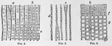
Fig. 4.—Section of pine-wood cut parallel with the medullary plates. a, spring growth, with large bordered pits: b, summer growth, with smaller bordered pits; c, medullary tissue.
