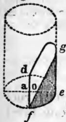
$$\text{Or, } \frac{2s^3}{3} - a c \times \frac{h}{vs} = V, \text{ vs representing the versed sine.}$$
