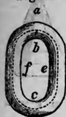
When the Ring is Elliptical.—Square the diameters of the axes of the ring, and multiply the square root of half their sum by 3.1416.
