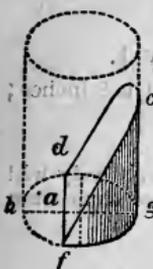
RULE.—4. When the Section passes through the Base of the Cylinder, and the Versed Sine,  $a g$ , exceeds the Sine. Fig. 37, Multiply the sine of half the arc of the base by the diameter of the cylinder, and to this product add the product of the arc and the excess of the versed sine over the sine of the base.
