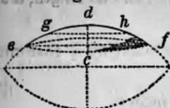
EXAMPLE.—The segment of a parabolic spindle, Fig. 102, has diameters,  $e f$  and  $g h$ , of 15 and 8.75 inches, and the length,  $c d$ , is 2.5 inches; what is its volume?
