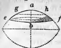
EXAMPLE.—The segment of a hyperbolic spindle, Fig. 105, has diameters,  $ef$  and  $gh$ , of 110 and 65 inches, and its length,  $ab$ , 25; what is its volume?
