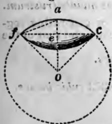
**EXAMPLE.**—What is the volume of a circular spindle, Fig. 93, when the central distance, *o e*, is 7.071067 inches, the length, *f c*, 14.14213, and the radius, *o c*, 10 inches?
