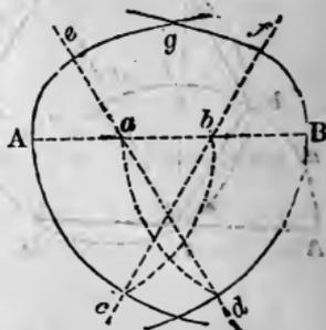
To draw from or to the Circumference of a Circle, Lines leading to the Centre, When the Centre is inaccessible --Fig. 22.
