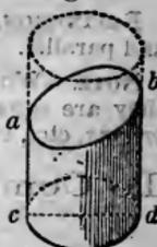
EXAMPLE.—The diameter of a cylindrical unguula is 10 inches, and the greater and less heights,  $bd$  and  $ac$ , are 25 and 15 inches; what is its curved surface?
