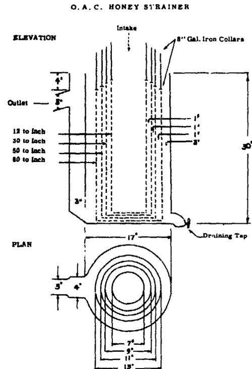
Each screen is equipped with a gate at the bottom to facilitate drainage. These gates may be opened from the top.
