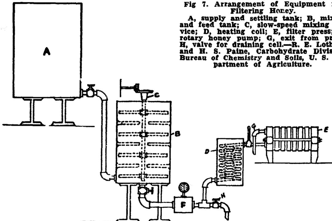
Fig 7. Arrangement of Equipment for Filtering Honey.
