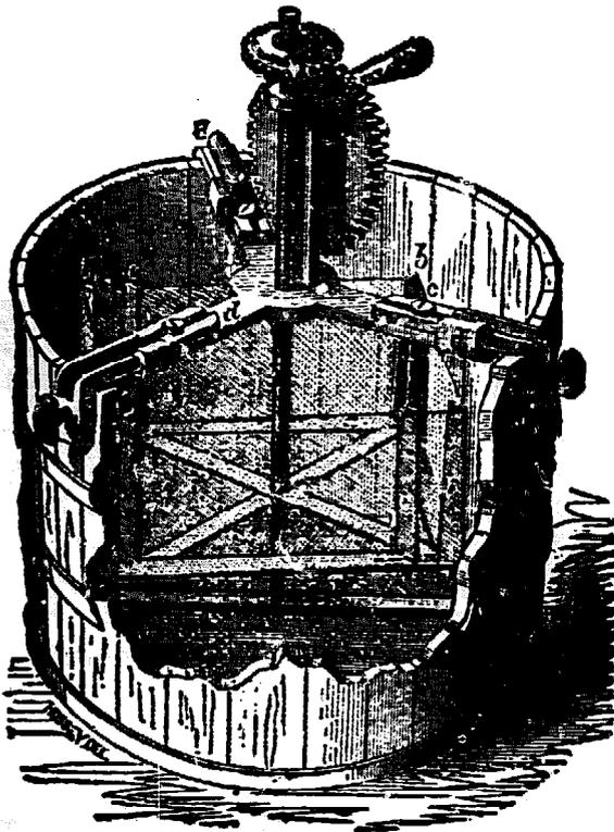
The first extractor built in the United States. Langstroth, the inventor of the hive and frame bearing his name, was the first to build a honey extractor in the United States. With his quick genius for the practical he early saw the necessity for gearing to increase the speed of the reel. —Illustration from American Bee Journal for 1868, page 189.
