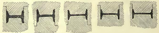
FIG. 8.—Reduction of Girder Section in Finishing Rolls.
