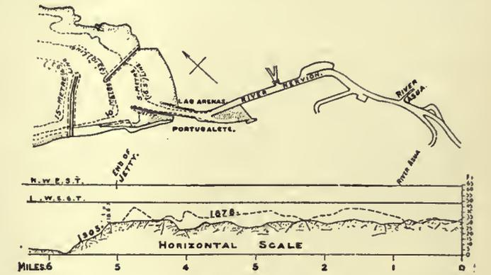
FIGS. 19 and 20.—Training Tidal River and protection of Outlet: River Nervion.
