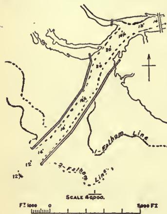
FIG. 9.—Jetty Outlet into Baltic: River Pernau.
