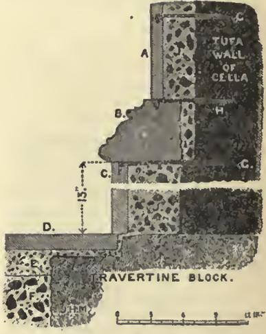
FIG. 4.—Example of Marble Lining, from the Cella of the Temple of Concord. A. Slabs of Phrygian marble. B. Plinth moulding of Numidian "giallo." C. Slab of cipollino (Carystian marble). D. Paving of porta santa. E and F. "nucleus" and "rudus" of concrete bedding. G, G. Iron clamps run with lead to fix marble lining. H. Bronze clamp. J. Cement backing.
