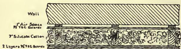
FIG. 5.—Insulation of a Cold Store.
