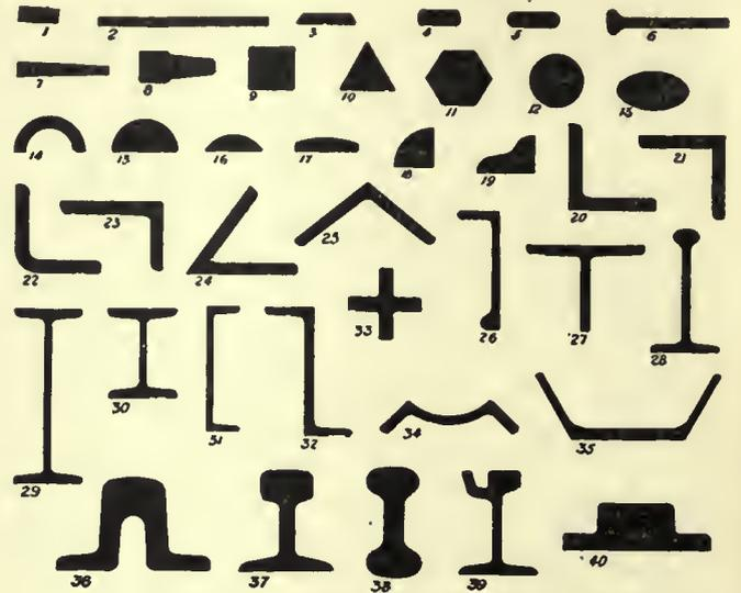
FIG. 1.—Forms of the Principal Rolled Sections.
