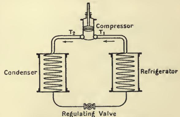
FIG. 2.—Vapour Compression Machine.
