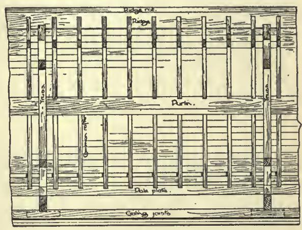
Half elevation; 25' 0" span.
