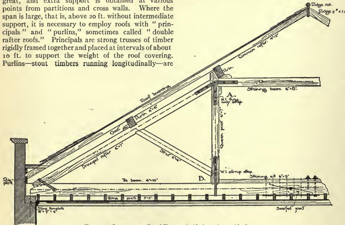
FIG. 3.—Queen-post Roof Truss; half elevation, 38' 0" span.
