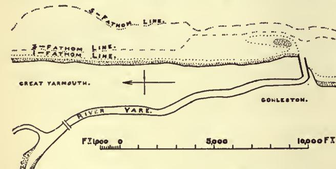
FIG. 10.—Shifting Outlet, fixed by Jetties: River Yare.
