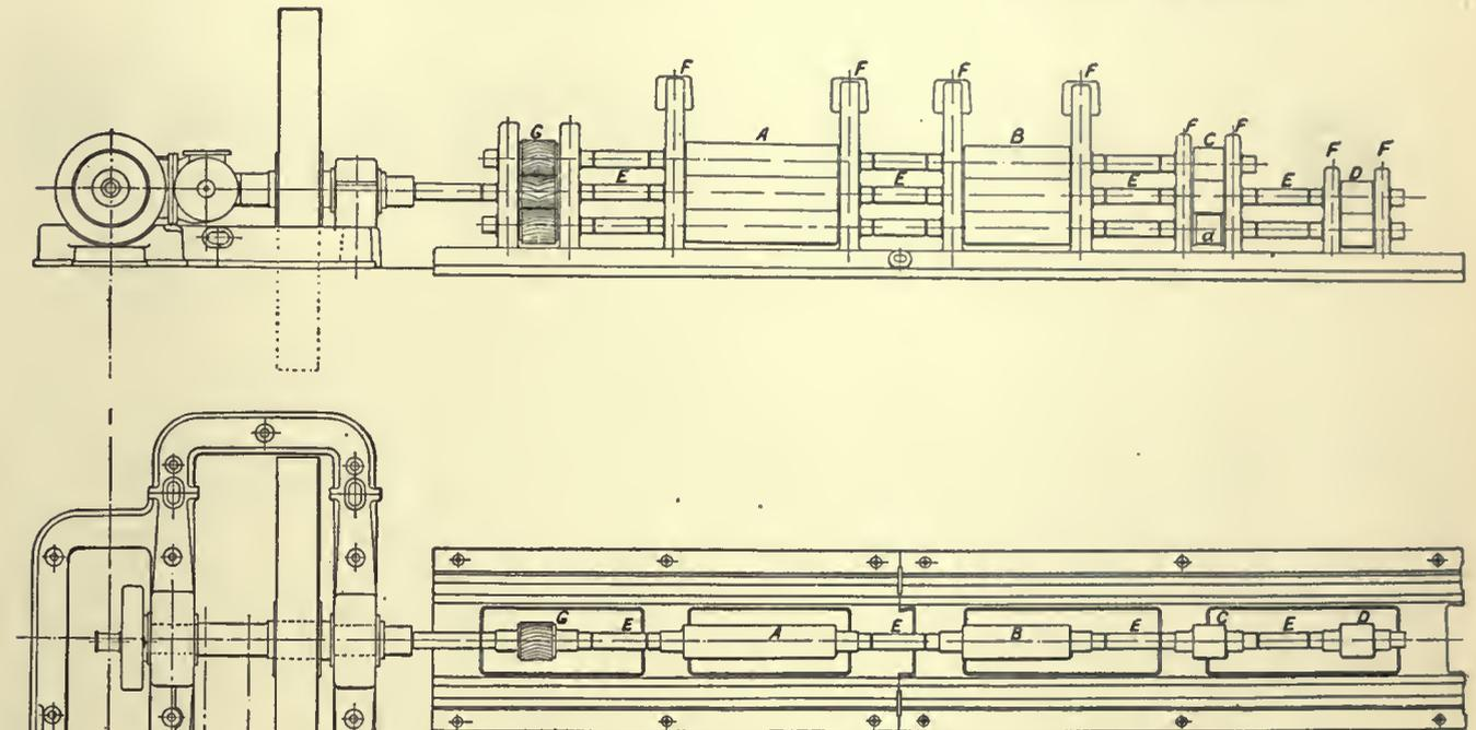
FIG. 3.—12-in. Merchant Guide-Mill and Engine. Four-set mill.
