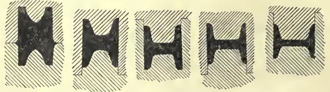
FIG. 7.—Reduction of Girder Section in Roughing Rolls.
