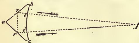
FIG. 36.—Vertical Section. Prism of Dioptric Spherical Mirror.
