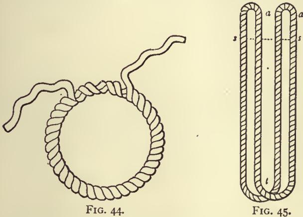
the space between the block and the thimble and hove taut by a Spanish windlass to cramp the parts together ready for the reception of a small round seizing. The cramping or pinching into shape is sometimes done by machinery invented by a rigger in Portsmouth dockyard. The strop may be made the required length by a long splice, but it would not possess any advantage.
