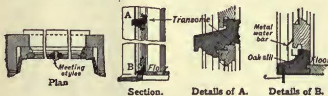
FIG. 9.—Details of French Casement to open inwards.
