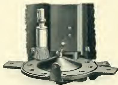
Corn Hopper, Inside View, Showing Seed Plate and Brush Cut-Off.
