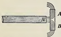
FIG. 464.—Lines of force pass through iron more easily than through air.
