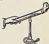
FIG. 299.—Water is a poor conductor of heat.
