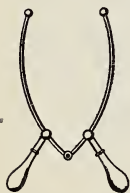
FIG. 500. — Discharging tongs. The handles are of glass or of ebonite.
