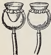
FIG. 110.—Rubber membrane forced inwards by pressure of the air.
