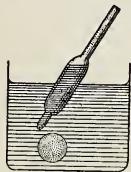
FIG. 169.—A sphere of olive oil in a mixture of water and alcohol.
