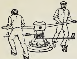
FIG. 76.—Raising the ship's anchor by a capstan.
