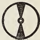
FIG. 417.—Disc to put over Newton's disc to cut out any desired colour.
