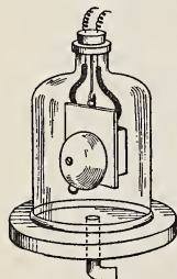
FIG. 187.—Electric bell in a jar connected to an air-pump. On exhausting the air from the jar the sound becomes weaker.
