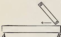
FIG. 471.—Magnetizing the steel bar AB .
