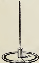
FIG. 186.—Illustrating torsional vibrations.
