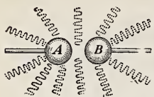
FIG. 613.—Diagram illustrating how the electric waves spread out from a spark gap.
