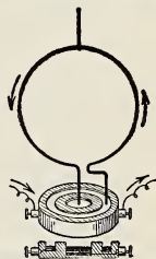
FIG. 536.—Experiment to show that a circular loop carrying a current behaves as a disc magnet.
