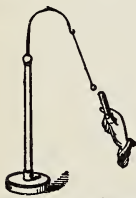
FIG. 477.—A pith ball on the end of a silk thread drawn towards the electrified rod.
