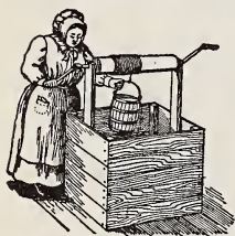
FIG. 75.—Windlass used in drawing water from a well.
