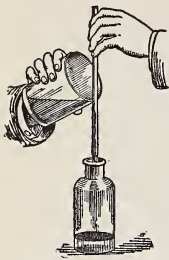
FIG. 178.—How to utilize surface tension in pouring a liquid.
