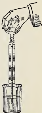
FIG. 247. — Expansion of a gas by heat.
