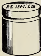
FIG. 5.—Imperial Standard Pound. Avoirdupois. Made of platinum. Height, 1.35 inches; diameter 1.15 inches. "P.S." stands for parliamentary standard .
