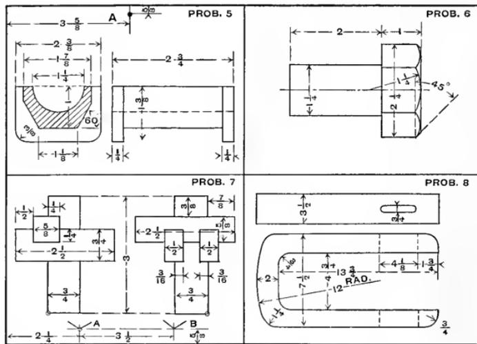
PROB. 5. Make the isometric drawing of the bearing illustrated, locating the upper corner at point A.
