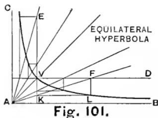
**92. The Equilateral Hyperbola.** Fig. 101. If the hyperbola is derived from a cone, the elements of which make angles of  $45^\circ$  with the axis, the curve is called an equilateral hyperbola. A knowledge of the construction of this curve is important, as it is the best approximation to the expansion curve of steam and is much used in connection with indicator diagrams.
