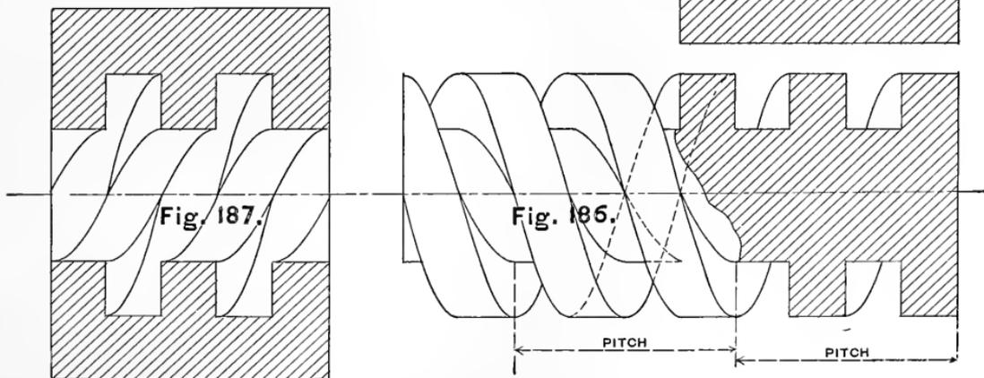
may be found and the side view likewise determined. Points in the curve may also be obtained by revolving the plane  $XY$  parallel to  $H$ , thus obtaining the height of any point, as  $N$ , which may then be projected into the other views.
