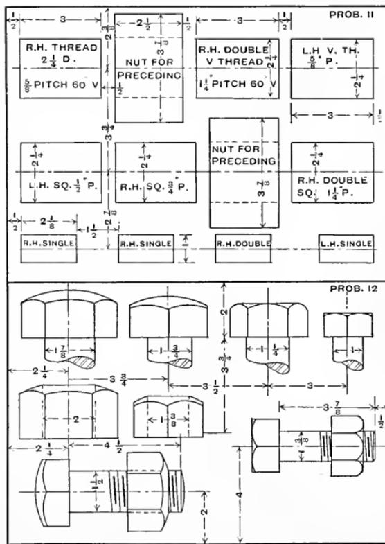
PROB. 11. The first four examples are of conventional V threads, Art. 133, page 108. The second four are conventional square threads. Art. 136, page 110. The last four are to be drawn by the methods illustrated by Figs. 177 to 180, page 109. Make the pitches about the same as those in the illustrations, estimating the spaces by the eye. Distinguish clearly between the single and double threads.
