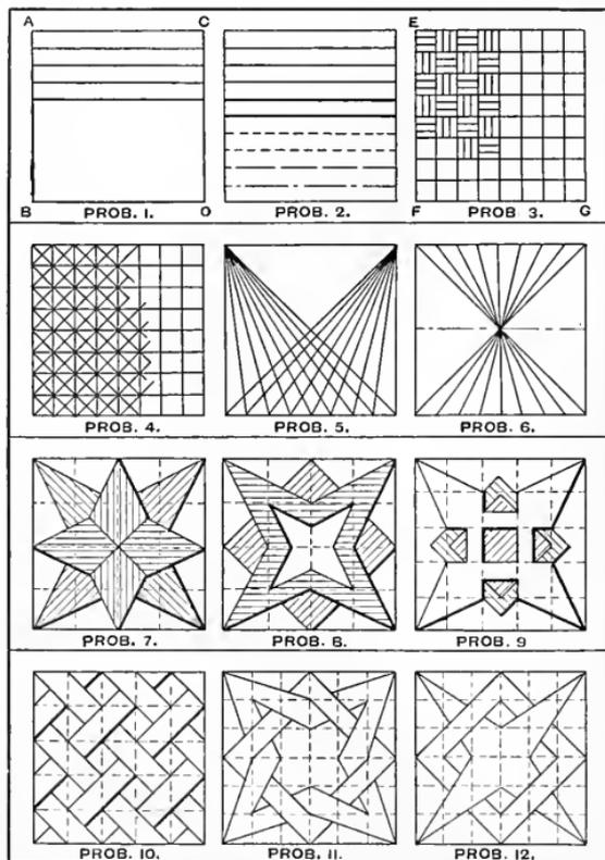
**PROB. 1.** By means of a triangle and T square draw AB and CD, and divide them into quarter-inches by the scale. Art. 13, page 8. Through these points draw parallel lines by the aid of a straight-edge or triangle, but do not use the T square. Their parallelism may be tested by sliding one triangle on another.
