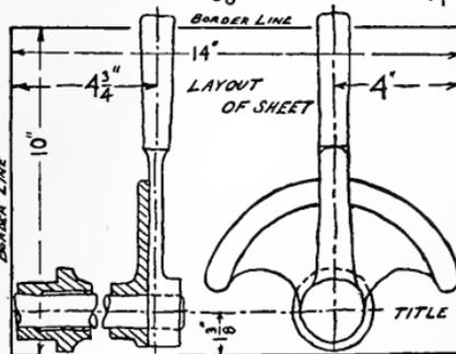
HAND LEVER FOR CONTROLLING CYLINDER VALVES U.S. COAST DEFENSE VESSEL MONTEREY
