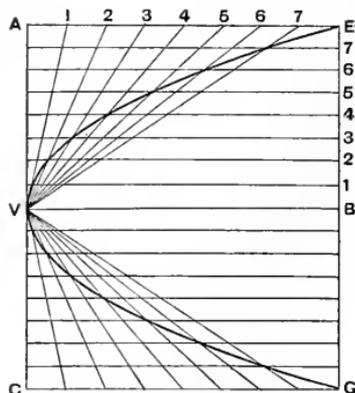
Fig. 97. PARABOLA SECOND METHOD
