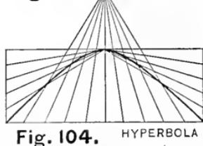
**93.** Figs. 102, 103, 104, illustrate the relation between the ellipse, parabola, and hyperbola, when constructed by the method which is common to all. In each case the height of the curve is the same and they have equal chords.
