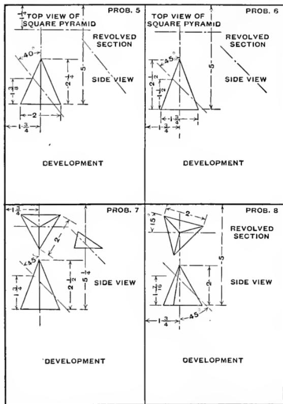
PROB. 5. This is a square prism, the diagonal of the base being 2". Observe that the base is cut by the plane, and one of the inclined edges will not appear on the completed development. In developing the surface open it on this line.
