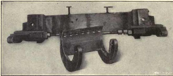
Fig. 6. Same Casting repaired with the Carbon Arc
