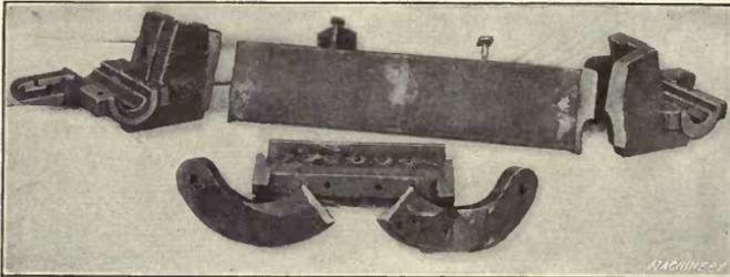
Fig. 5. Broken Casting from a Wood-working Machine
