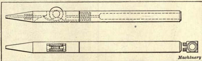
Fig. 6. Holder for Applying the Solder by Hand
