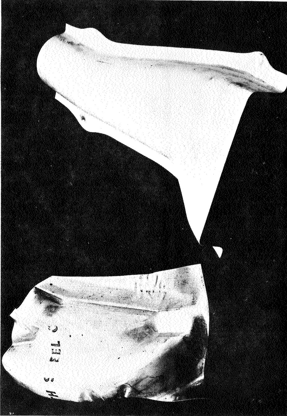
FIGURE 81. DC8 OUTLET HALF AND DUCT ASSEMBLY 0.025 AND 0.032 THICK
