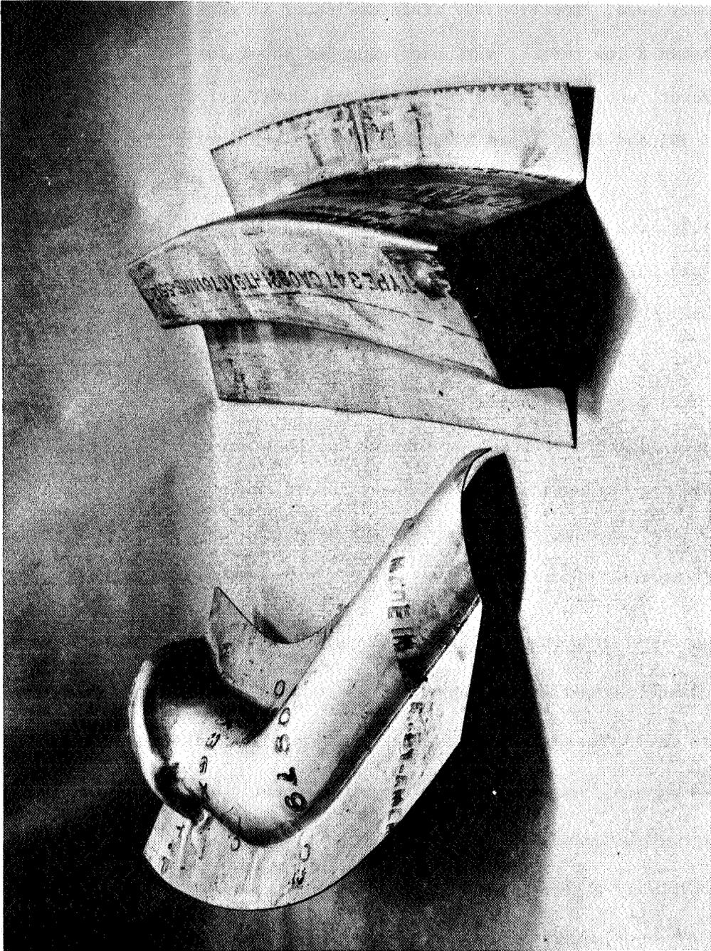
FIGURE 80. DC8 DUCT HALF AND CHANNEL, DROP-HAMMER FORMED FROM 0 032 THICK TYPE 347 STAINLESS STEEL
