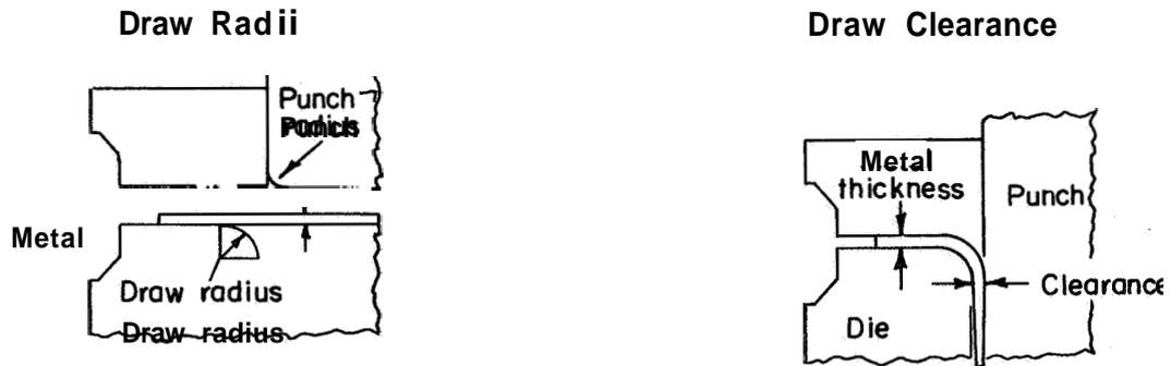
FIGURE 32. DRAW RADIUS AND DRAW CLEARANCES FOR STAINLESS STEELS (Ref. 77)
