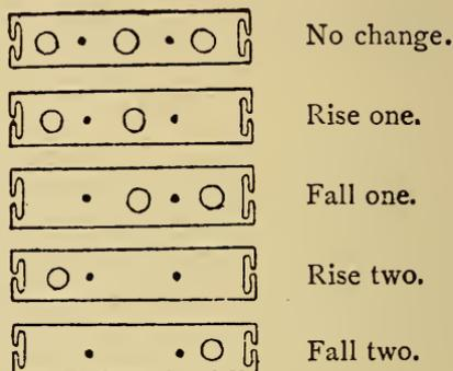
Rising one means that the box is risen to the next shelf; rising two is risen to the next shelf but one, skipping one. This style of drop box can be driven at the speed of 170 picks per minute. Generally, a weaver attends to three of these looms, and an overlooker to from 50 to 60. For the check shirting trade looms to weave from 30-inch to 37-inch cloth are used.
