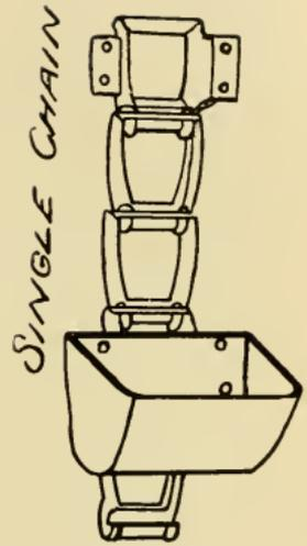
FIG. 71. Sprocket Chain Elevators.
