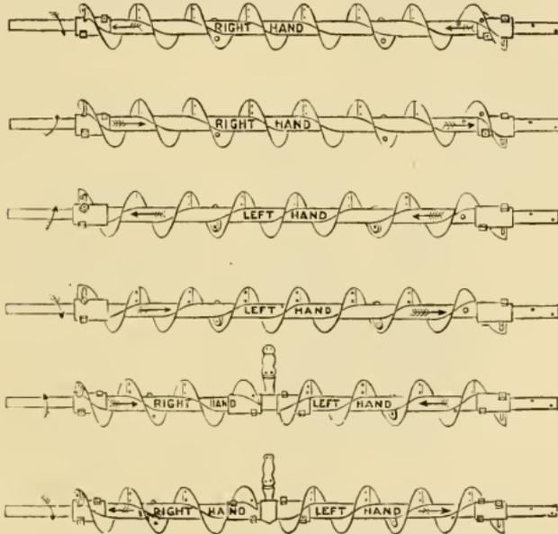
FIG. 68. Right and Left Hand Conveyors.
