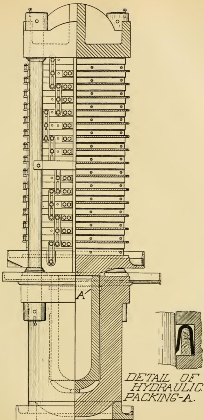
FIG. 101. Oil Press, Showing Hydraulic Packing.
