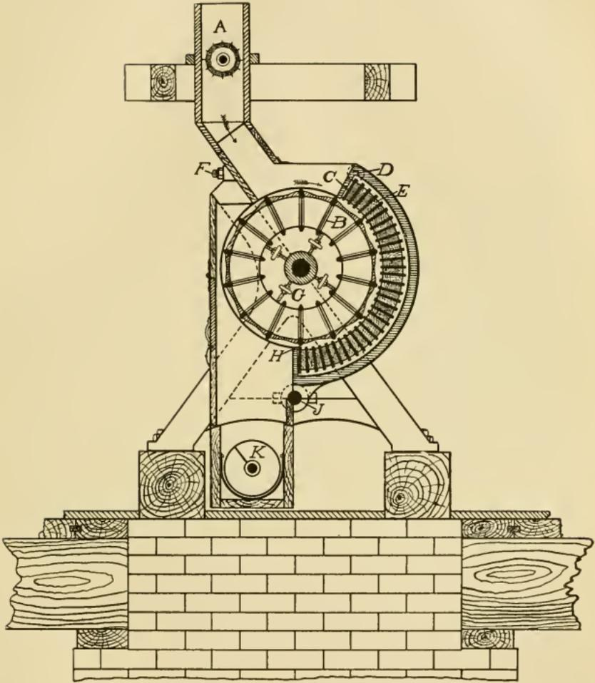
FIG. 80. Section Through Huller.
