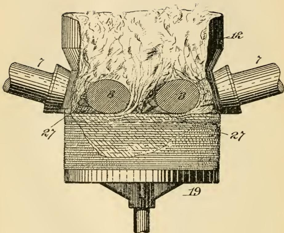
FIG. 38. Ginnery Compress, End Packed Cylindrical Bale.
