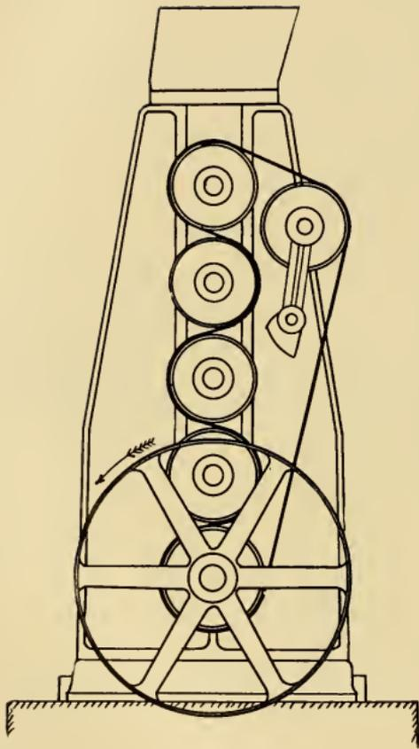
FIG. 83. Diagram Serpentine Drive for Rolls.
