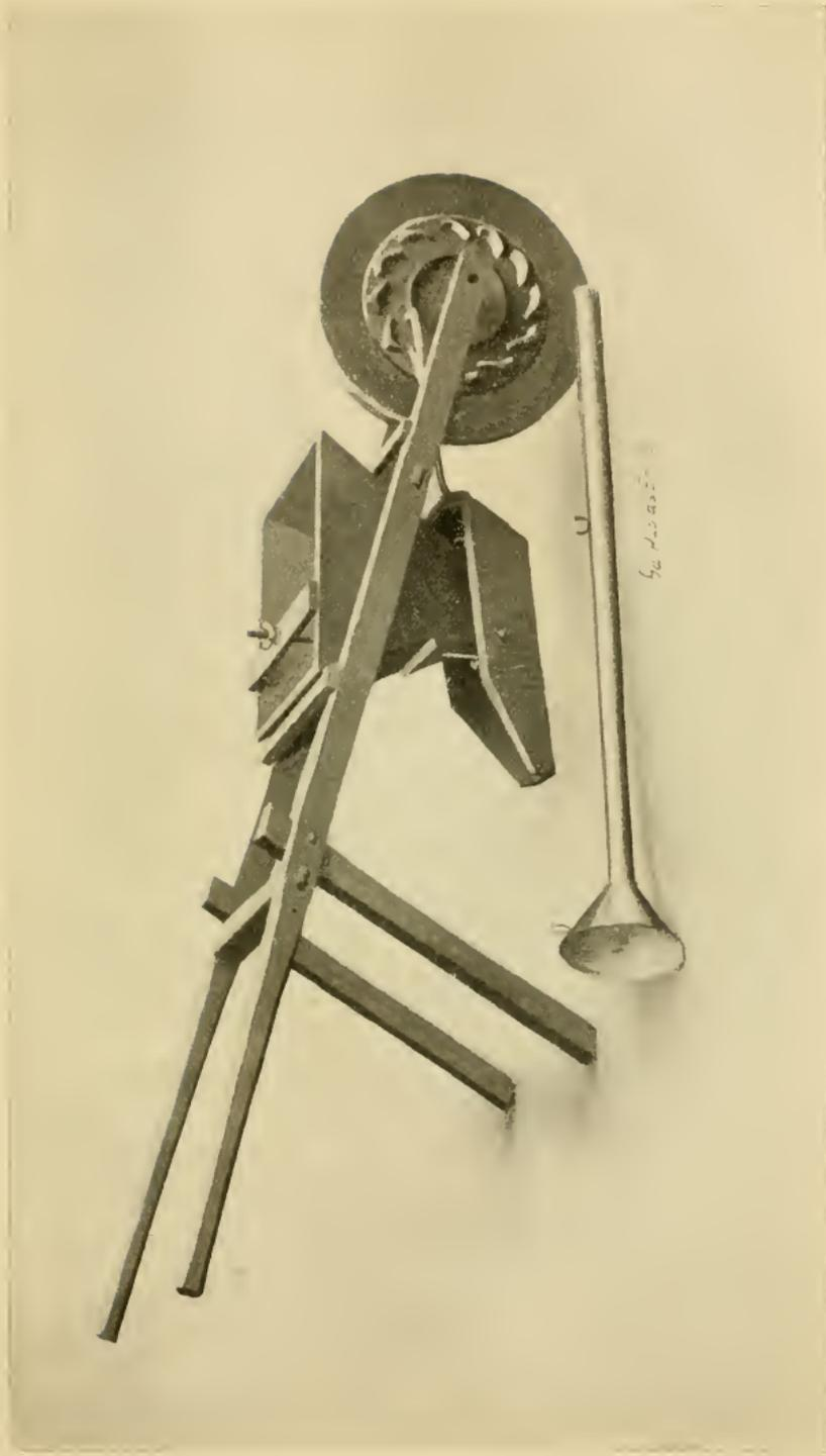
FIG. 47. Fertilizer Distributor and Guano Horn.
