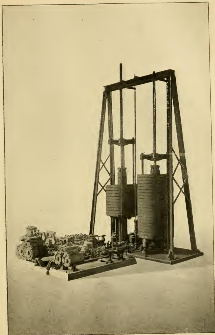
FIG. 104. Hydraulic Accumulators.
