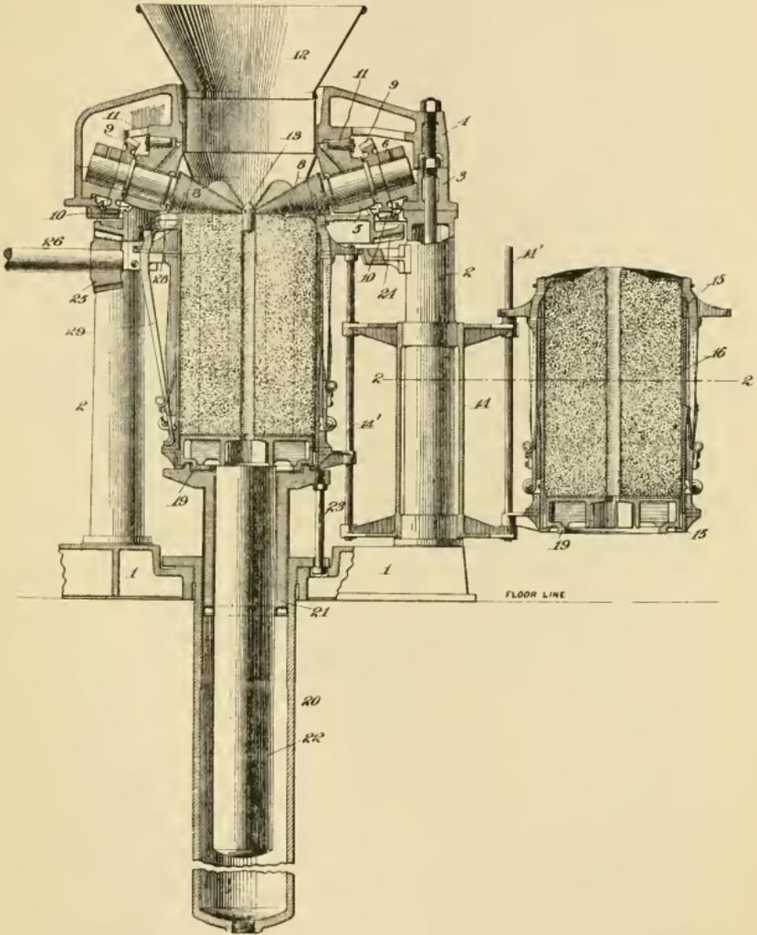
FIG. 37. Ginnery Compress, End Packed Cylindrical Bale.
