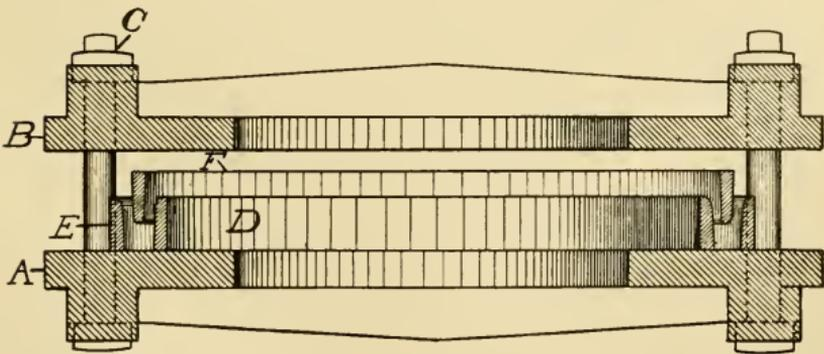
FIG. 102. Mold for Making Hydraulic Packing.
