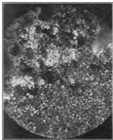
FIG. 5.—Internal structure of limestone. (Magnified 20 diams.)
