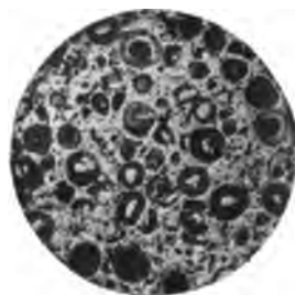
FIG. 10.—Fossil-bearing limestone. (Magnified 20 diams.)
