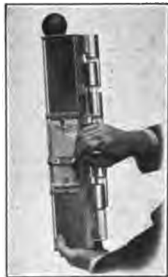
FIG. 2.—Universal Sand Tester—portable instrument for making mechanical analyses of sands. 2
