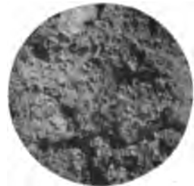
FIG. 1.—Rough fracture through porous floor slab. (Magnified 2 diams.)
