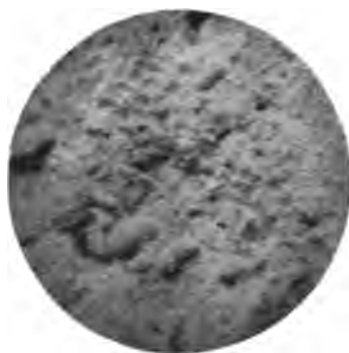
FIG. 6.—Enlarged surface of piece of gravel, showing roughness. (Magnified 5 diams.)
