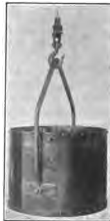
FIG. 29.—Round self-tilting bucket.
