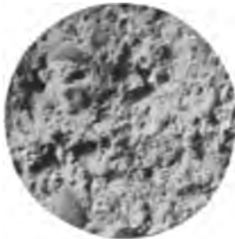
FIG. 2.—Dusting surface of concrete floor. (Magnified 5 diams.)
