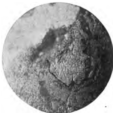
FIG. 1.—Iron pyrites ( \text{FeS}_2 ) in concrete aggregate oxidizing and destroying adjacent matrix. (Magnified 40 diams.)
