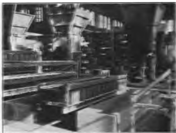
FIG. 109.—Block machines with hoppers above are shown in the background and block cars in the foreground. Note the two floor levels. The cars run on tracks into pits so that four decks can be loaded without too high a reach. The empty "decks" from the car at the left are placed on the car at the right as it is piled.
