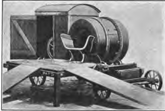
FIG. 18.—Low charging drum mixer.
