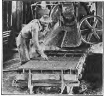
FIG. 105.—Metal gang molds mounted on car.
