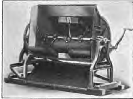
FIG. 20.—Batch mixer of the shoveling type.
