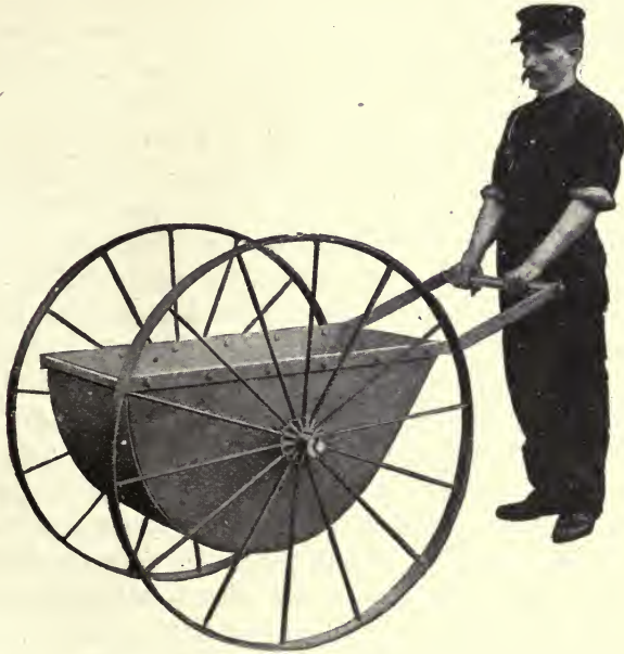
Fig. 12.—Two-Wheeled Ransome Cart for Hauling Concrete.
