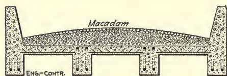
Fig. 154.—Cross-Section of Concrete Girder Bridge.
