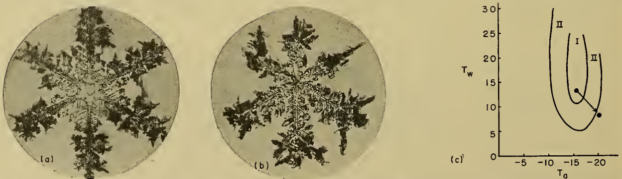
FIG. 28.—(a) Natural, and (b) artificial crystals of dendritic type with small plates attached; (c) physical conditions during course of formation.
