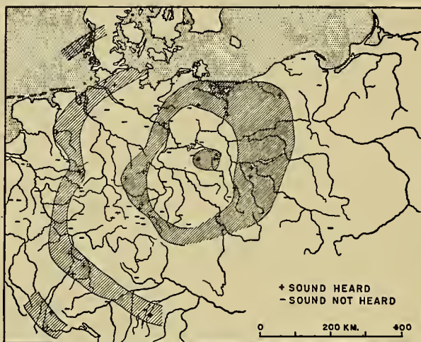
FIG. 8.—Observations of sound waves through the stratosphere after explosion of 5000 kg of ammunition, December 18, 1925. (After Hergesell and Duckert [16].)
