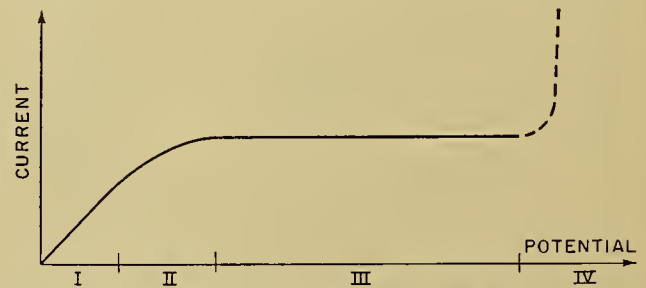
FIG. 5.—Schematic curve of the current-potential relationship (characteristic) in an ionized gas at rest.
