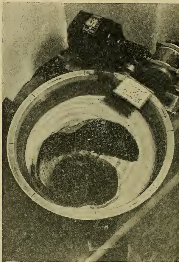
FIG. 12.—Ink initially of slightly greater density, a couple of minutes after being poured into a pan of water in solid rotation at 15 rpm. Note the vertical walls. As in Taylor [63] the walls remain vertical for many minutes and gradually draw out into surfaces which are sharply divided by clear areas when viewed end-on. The same effect is very marked to at least as low as 5 rpm and occurs under the heating conditions of Fig. 11 when the pan bottom is insulated by a layer of plaster.
