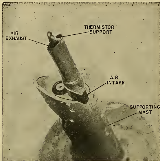
FIG. 1.—Photograph of a "vortex thermometer" as designed by P. J. Harney for measuring true air temperature from an airplane. (Courtesy of Signal Corps Weather Radar Research at M.I.T.)
