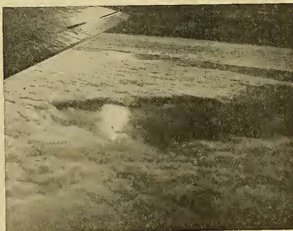
FIG. 1.—Reflection of sunlight on aluminum aircraft wing, ice-crystal cloud, and supercooled water-droplet cloud. Note that the reflection from the ice-crystal cloud is nearly as bright as that from the wing.
