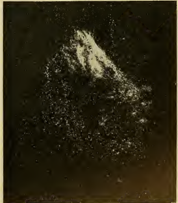
FIG. 8.—Snow crystals forming in a cold chamber with air supersaturated with respect to ice.
