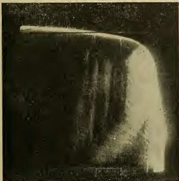
FIG. 8.—Photograph of RHI scope showing tall (snow) shower with abrupt shear below the altitude of 9000 ft. Lack of shear in showers more distant from the radar can best be explained by nonuniformity of the wind field. Storms are approaching the radar; shear therefore indicates decreasing wind velocity with altitude (in the plane of the picture) up to the point where echo signal edges become nearly vertical. Actual slope of shower in shear zone about 80^\circ from the vertical (X-band radar). ( M.I.T. Weather Radar Research. )
