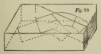
known as the bevel cut. The top portion of the wreath is the same as the bottom. To make the joint at the shank end, it may be necessary to use the short piece of falling mould as at Fig. 34.
