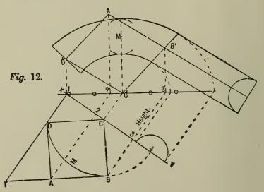
Fig. 12 is the face mould, the square, ABCD, being drawn the same as Fig. 11. Having drawn the center line the next step is to determine the horizontal trace or directing ordinate, for all ordinates must be parallel to this line.
