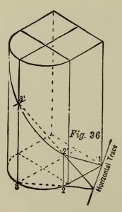
the major axis from the mould to the stuff. Square over the minor axis line on both edges and mark the distance from M to the dotted line at Fig. 35, on one side of the minor axis line at the top and on the other at the bottom.
