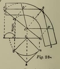
Fig. 28: The pitches of the wreath being equal, the face mould is drawn same as those in previous plates.
