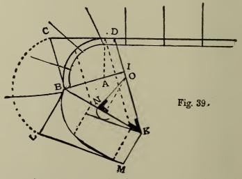
struct Fig. 39 draw radius from center A to joint of rail at newel B. At right angles to AB draw BC. This will give the angle of tangents on ground plan. In wreaths of this shape the tangent BC is always level so as to give a plumb joint at the newel.
