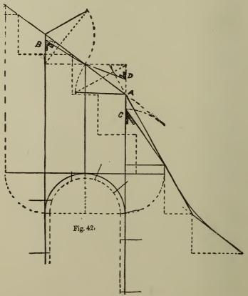
In Fig. 42 we represent a flight of stairs with four winders, quarter landing, and return flyers.
