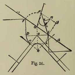
Fig. 26 shows the development of the angle of tangents for the face mould and the bevel for springing the wreath. Draw the angle ABC on center line of rail as shown; draw dotted line from center O to B; draw DE at right angles to OB; from center B swing around A and C to D and E; set up one riser from D to F, and one down from E; mark one step above and below the pitch-board; draw pitch-line XX.
