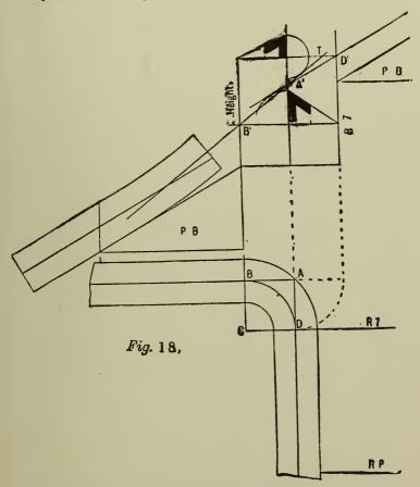
A'D' is produced past A', which is the point where the center line of the lower portions must meet it. It will be seen that if the center line of the lower portion had been produced, it would cut the perpendicular below
