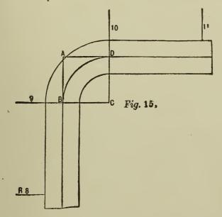
Fig. 15 is the plan of a rail for a quarter-space land ing, the risers' landing and starting being placed in the springing of the well. The radius of the center line of rail being equal to half a tread, the pitch-board gives the inclination of both tangents. If a square block be cut with two of its adjacent sides to the same pitch, it will be seen that a line joining the two opposite corners is horizontal. This being known, it is unnecessary to unfold the tangents.
