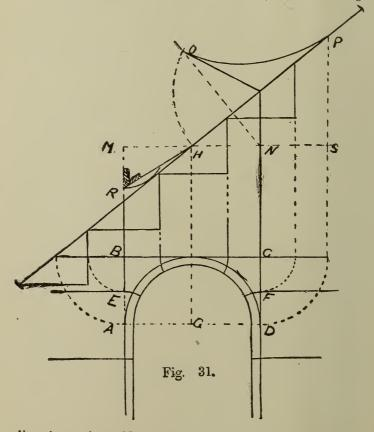
line drawn from N at O; connect LO, and the triangle OLP gives the tangents for the face mould.
