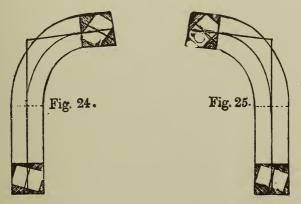
Figs. 24 and 25 show the sections and application of bevels on rails. Fig. 24 is the lower and Fig. 25 the upper wreath; the same face would serve for both, as the upper and lower pitches are the same.
