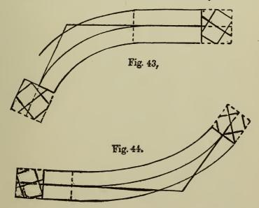
Fig. 43 shows the face mould for the lower wreath, and Fig. 44 for the upper, also sections of rail and applications of the bevels.
