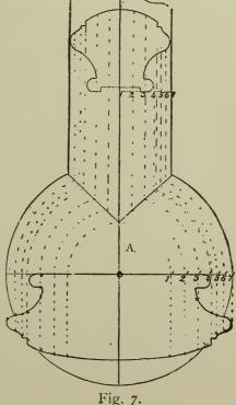
upper section shows the rail, which is supposed to be the full size; the lower section shows the cap, which may be of any reasonable diameter. Draw the plan of the cap as shown, then a section of the rail, then draw
