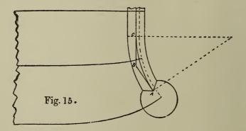
Fig. 15 shows the plan of turnout steps, with rail mitering into cap. The dotted curved line shows face of string. The black line shows center of rail with tangent ABC at right angles to dotted radius.
