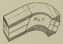
shown by the dotted lines. The joints are made square to these lines. Mark the center of the piece at each end. With a bevel set to the long edge and riser side of the pitch-board, draw the line through
