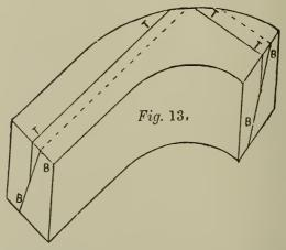
lines, then with the bevel for each end, draw the lines BB through the center of the stuff. Square over these lines on the face on both sides as seen by the dotted lines on the top side.
