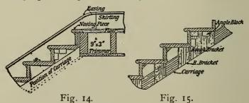
risers on the underside, and having pieces of rough boards—ends up—nailed to the rough carriage pieces and made to fit snugly against the underside of the tread and the inside of the riser. This method is not a commendable one, though much employed, as the nails may get loosened by the continual jar that a flight of stairs is subject to—a solid carriage piece is much better for the purpose.
