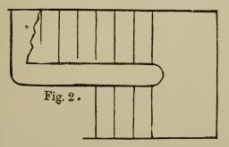
Fig. 2 shows a plan of a stair with a landing and return steps.
