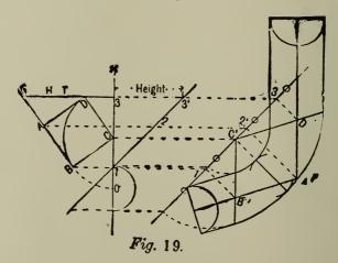
Fig. 19 shows the face mould for Fig. 18, obtained in the same way as those for Fig. 1 on the last page.
