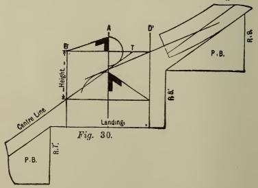
are taken from them. For the extra thickness required for this wreath the distance ST, Fig. 27, would be quite sufficient over what is usually allowed. Fig. 30 is the development for the wreath to be in one piece with the easing on the straight rail at the top. The face mould is not drawn, being similar to those already explained.
