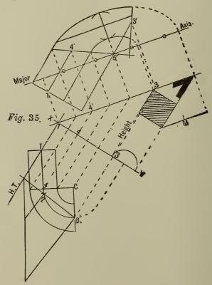
Fig. 35: Redraw the plan with the points as shown. Join 3 and 2, and produce the line to the left and on this line erect perpendiculars from 3 and 2. Make the one from 3 the height of I'-3' at Fig. 34, and the one from 2 the height of I'-2', Fig. 34. Draw
