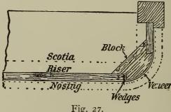
whole length of curve and return, but is cut out where the curve occurs and thinned down to a quarter of an inch. A solid block, as shown, is fastened to the floor in the proper place, being curved to the right shape. The newel is put in position, but is rebated out the depth of the riser, as shown. The thin portion of the riser is then steamed, glue is put on the block, and on
