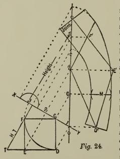
Fig. 24 is the face mould for the top portion. To find the height where the pitch cuts the springing line F'F", Fig. 22, draw the line F'F" at right angles to D"; then to the lineatright angles to D'D", through the joint is the height. Where the line through the joint cuts E'F' at O, with O as center, draw a circle tangent to the pitch and cutting
