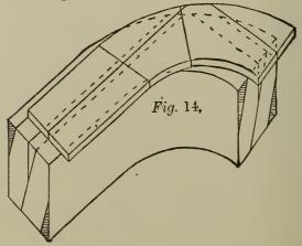
Fig. 14 shows the face mould in position with the tangent lines held to the corresponding line on the wreath. The etched part shows the amount to be taken off.
