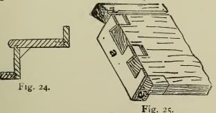
method of building a step is shown at Fig. 24. Here the riser is tongued into the tread above and runs down below the lower tread, but fits close to its edge to which it is nailed as shown in the upper portion.
