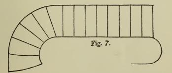
Fig. 7 is the plan of a stair similar to Fig. 6, but having seven winders.
