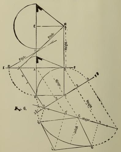
can be readily obtained. At right angles to HT draw X2, Y2 through the center C; by doing this the line that shows the true inclination will also contain the major axis of the elliptical section. Parallel to HT
