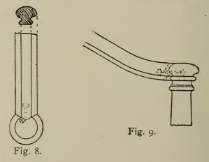
the joint or miter lines as shown, and from the outside points of these lines draw parallel lines with the central line A. Divide into spaces as shown by the dotted lines, then at the junction with the miter lines describe semi-circles as shown, until they cut the line of diameter. Square down these lines and from them prick off the points as figured, and through these prick points describe the curves and squares; then, when mitered
