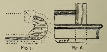
The sketches shown at Figs. 5 and 6 exhibit the end of the bottom step, which is semi-circular or "bullnosed," also an end view of the lower tread and riser with the shank of the newel passing through. The position of the newel, with regard to the step, is shown by the dotted lines in Fig. 5.
