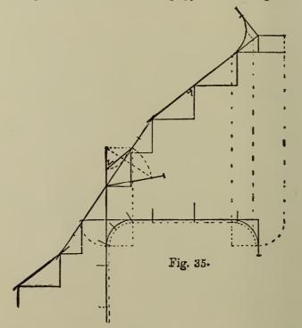
plan and elevations of treads and risers. The explanations given for the solution of previous examples will apply to this one if the figure be properly studied, as the method of proceeding to lay down the rail is exactly the same.
