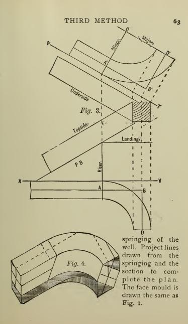
Fig. 4 shows the wreath piece cut out and worked into cylindrical form ready for squaring, the face mould being applied the same as in Fig. 2. The face mould gives the line for squaring the top off, and a better curve is obtained. It will be seen at Fig. 3 that
