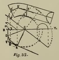
Fig. 32 is the face mould. Redraw the center line with its tangents AB and BD; produce AB to T, making BT same as B'T, Fig. 6. Draw the ordinate TD; draw XY at right angles to TD through the center C and draw projections from A and B, and on TD produced. Set up the height H, taken
