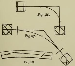
By carefully studying Fig. 12, the landing wreath, Fig. 36, will be easily understood. Care must be taken to locate the last riser as near half a step from the level tangent as possible.
