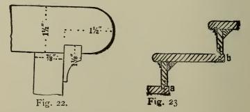
where the cove is glued into a groove made in the tread. When the work is put together the cove is braded to the riser, which ties the tread down solid to
