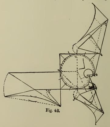
the width of treads to correspond with the points where the risers cut the tangents in Fig. 48. These elevations also give the exact height as shown; the first wreath in Fig. 49 is lifted for the newel, and the landing wreath in Fig. 48 runs half a rise above the floor.
