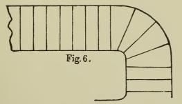
Fig. 6 shows a plar. of a quarter-space stair with four winders.
