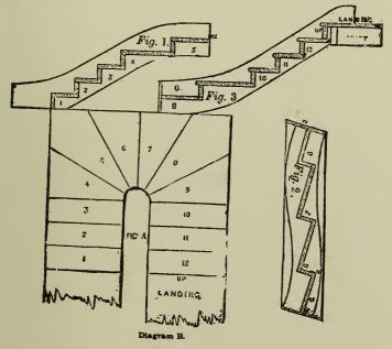
out the winder. You will see that a piece must be glued on the under side of string. I have shown easing at top, and also shown ramp at bottom to receive base, etc.
