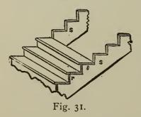
each side. The tread is shown at t and the riser at p. These are a cheap kind of stair and are nailed together. This class of stair is generally intended to fit in between walls or parti tions, the strings being spiked to studding or to board timbers or
