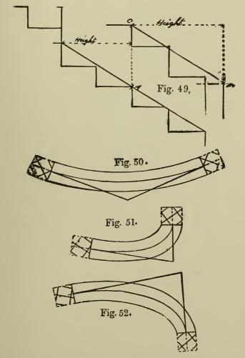
and are drawn as shown in Fig. 48. Figs. 50, 51 and 52 show the face moulds and application of the bevels, in the same manner as explained in previous illustrations.
