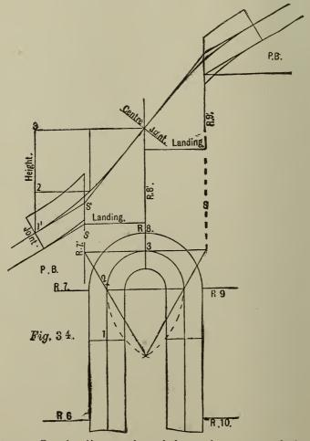
line. On the line projected from the center of the well, mark off the height of a riser and draw the second
