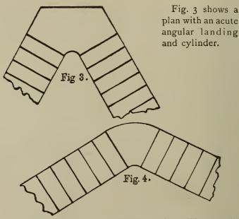
Fig. 4 shows the same kind of stair as Fig. 3, only being at an obtuse angle.
