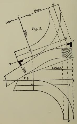
the shank is not in the center of the stuff. The shaded portion shows the slab to come off one side.
