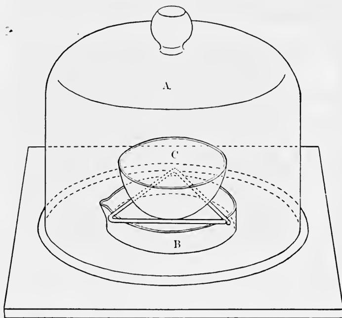
FIG. 22.—Ammonia determination, Schlösing method. A, bell-jar; B, dish containing urine; C, dish containing acid.
