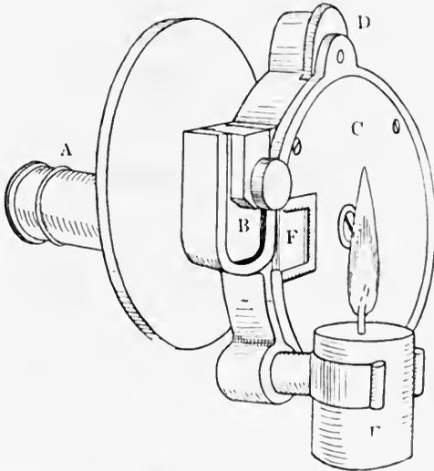
FIG. 111.—Dare's haemoglobinometer. A, telescope; B, pipette in place; C, case inclosing color-prism; D, milled head moving prism; E, candle; F, window admitting light to color-prism.
