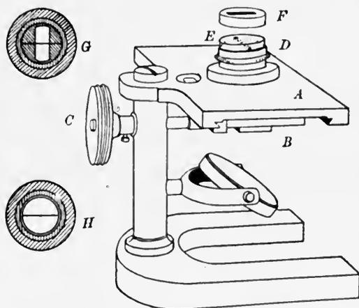
FIG. 105.—Miescher's modification of Fleischl's hæmoglobinometer. *A*, stage; *B*, color-prism rack; *C*, milled head; *D*, cell; *E*, cover-glass; *F*, cap; *G*, cell seen from above; *H*, cell of Fleischl's instrument.
