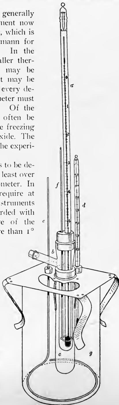
FIG. 62.—Apparatus for freezing-point determinations. *a*, thermometer graduated to  $0.01^{\circ}$  C.; *b*, tube for fluid to be investigated; *c*, air-chamber; *d*, thermometer for freezing mixture; *e*, stirrer for freezing mixture; *f*, stirrer for fluid; *g*, jar for freezing mixture.
