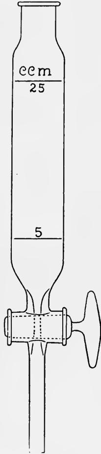
FIG. 63.—Strauss' separating funnel for lactic acid tests.
