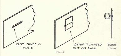
be filed smooth. The inside cutting is accomplished by first drilling a small hole, then inserting the saw and re-fastening it in the frame.
