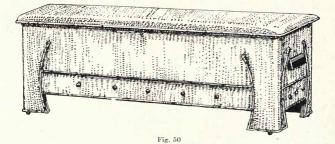
Cut the sides and ends to the desired shape, Figs. 50 and 51 offer excellent suggestions, and square the ends of all four pieces. Nail or screw the boards together, and glue in triangular corner strips on the inside.
