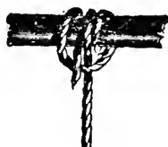
Fig. 14.—Magnus Hitch. (Not Apt to Slip Along a Pole)
