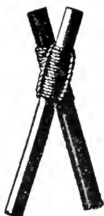
Fig. 13.—Shear Legs Spread
