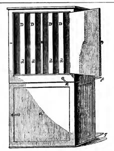
The box hive is thus made:—Plate ii. fig. i. and fig. ii., two boxes made to part in two, is eighteen and a half inches high, or nine and a quarter inches each high, and ten inches square.
