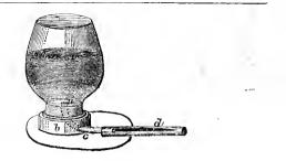
When the bottle is filled with syrup, the cork should be pressed in and the whole inverted, when the syrup will flow into the trough, until level with the top of the small tube, and will continue to do so as long as the supply in the bottle lasts.
