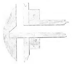
a. Frames 16 in the brood room and eight for the honey room, size inside  $105_8$  by  $85_8$ , wood used, fifteen-sixteenths by three-sixteenths distance pieces, q,  $1\frac{1}{2}$  by  $\frac{2}{3}$  by  $\frac{2}{3}$ , frames planed on edges and outsides.
