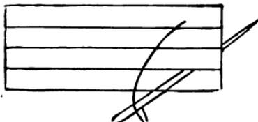
FIG. 41.—FIRST STAGE OF KETTLE-STITCH.
