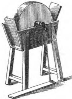
FIG. 10.—GRINDSTONE FOR PLOUGH-KNIVES.
