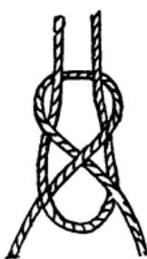
**COMMON BEND**—Make a bight with the end of one rope, and pass the end of the other through the bight from beneath, and round both parts with the end under its own standing part. The greater the strain, the faster will this bend jam.
