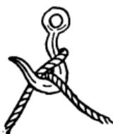
**BLACKWALL HITCH**—It is the simplest method known of making fast the end of a rope to the hook of a tackle. The figure is self-explanatory, the underneath part of the rope being jammed hard and fast by the strain on the hook.
