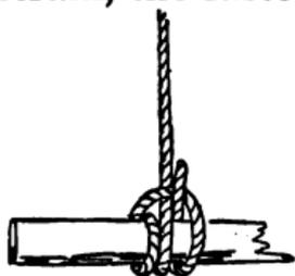
**MAGNUS HITCH**—Pass two round turns with the end of a rope over a spar, then take it before the standing part, pass it again under the spar and up through the bight.
