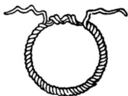
**GROMMET STROP**—It is made of a single strand of rope. To make it, lay one end over the other at the size required, and with the long end follow the lay round until a ring is formed with three parts of the strand all round. Finish by di-
