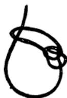
**RUNNING BOWLINE**—It is made by passing the end of a rope round its standing part and forming a bowline as in Fig. 8.
