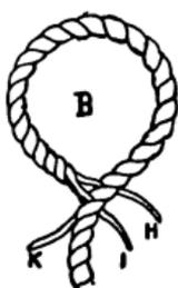
**EYE SPLICE**—Unlay the rope and lay the strands E, F, G at the proper distance upon the standing part, as shown at A. Now
