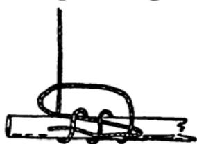
**GAFF TOPSAIL HALYARD BEND**—Pass two turns round the spar, then lead the end back round the standing part and underneath all the turns, bringing it round to its own part and back again over the two outer turns and underneath the inner turn.
