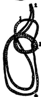
**BOWLINE ON A BIGHT**—To make it, double the rope and take the doubled end (1) in the right hand, the standing part (2) of the rope in the left hand. Lay the end over the standing part, and by turning the left wrist form a loop (3) having the end
