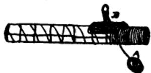
This illustration shows the process of parcelling and serving. After the worming is finished wrap narrow strips of canvas—tarred, if the rope is of hemp, and painted if it is of wire—round the rope with the lay, secure the parcelling to the rope by marling it with twine, the rope can then be served against the lay. Lay the serving mallet B with its groove on the
