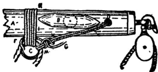
It is then passed through *d* round through the cringle *e*; through *d* again and through *e* again; then up over the gaff at *i* and *k*, down the other side and through *e* again, and so on up round the gaff four or five times; at the last, instead of going up over the gaff again, the earring is passed between the parts round the gaff as shown at *f*, round all the parts that were passed through *d*, as shown at *m*, and jammed by two half hitches *m* and *h*.
