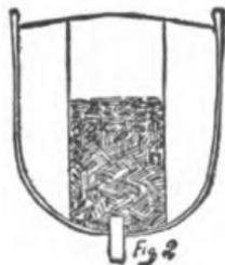
The vessel in this case would labor quite heavily on the slightest provocation and would not be so steady or so seaworthy as the one first mentioned, with the narrow bin or compartment extending to the upper deck.
