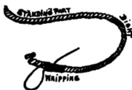
The ends of all ropes, whether belonging to the running or standing rigging, must be whipped with tarred roping twine or they will unravel. Take the rope in your left hand and lap the twine round it very tight a dozen times, taking care that the end lies under the first turns so as to secure it. Then make a loop with the twine and continue the lapping for four turns round the rope and the end of the twine, as shown above. Haul taut and cut off the end.
