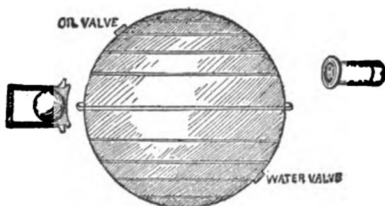
The specific gravity of oil will keep it in the upper part of the distributor, and the motion of the globe on the breaking waves or swell will insure the ejection of the oil through the graduated valve in any quantity."
