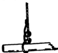
**TWO HALF HITCHES**—Pass the end of the rope round the standing part and bring it up through the bight. This makes a half hitch. Repeat the process and haul taut. If the knot is to bear a great strain, seize the end back with spunyarn to the standing part.
