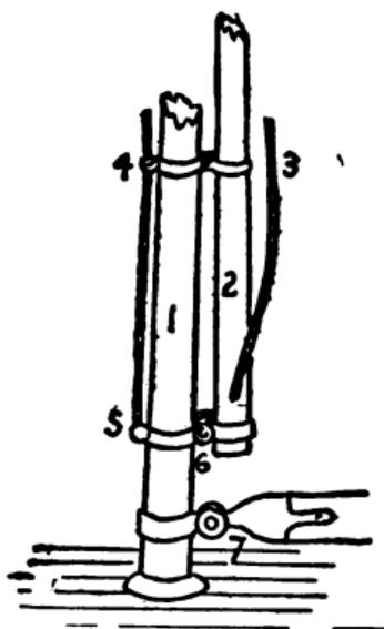
Detail of Sliding Gunter Rig, Fig. 6.
