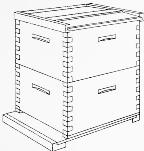
Fig. 5.—Eight-frame Langstroth Hive, Two Storey.
