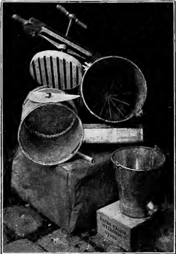
Fig. 7.—Metal Wax-press showing parts.
