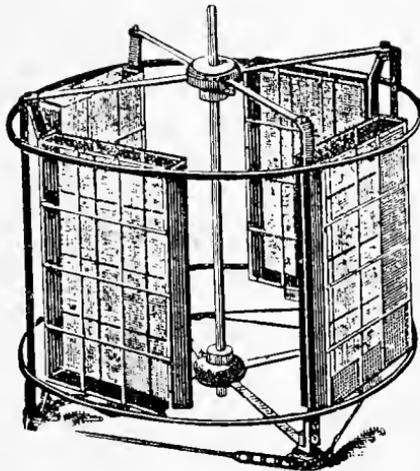
Fig. 3.—Reel of Four Comb Reversible Extractor.
