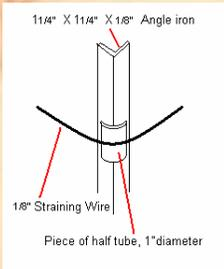
It is now important to tie the whole structure up with angle iron at all corners bound together with fencing wire and barrel tensioners (Turnbuckles). I have found it useful to insert half sections of steel tubing on the corners to ease the stretching process of the fencing wire (see the drawing left). If you enlarge the picture on the right, you will see 2 tensioners/turnbuckles on the left-hand side of the kiln, roughly in the middle.
