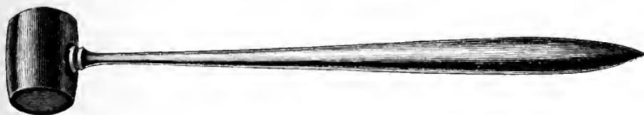
FIG. 121.—Hand mallet for condensing gold.
