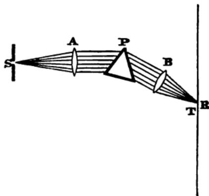
At  $s$  is a narrow slit, which is supposed to be perpendicular to the plane of the paper. Through this slit a thin line of light passes, and it is this thin line of light which is to be examined in the spectroscope. After passing through  $s$ , the light diverges until it falls upon an achromatic lens
