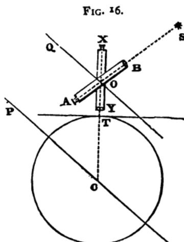
centre of the earth  $c$ . In the position  $A B$  the telescope is directed towards a star. The angle  $s o c$  represents the angle through which the telescope must be turned, in order to be moved from the star to the nadir. Hence the angle  $x o s$ , which is the zenith distance of the star, is known.
