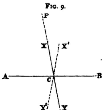
the intersection of the central vertical wire with the horizontal wire (fig. 8). Now, suppose the telescope to be lifted out of its bearings and replaced with the pivots reversed—*i.e.*, the pivot which was formerly to the east is now at the west—and let the telescope be again directed to the distant mark, then if
