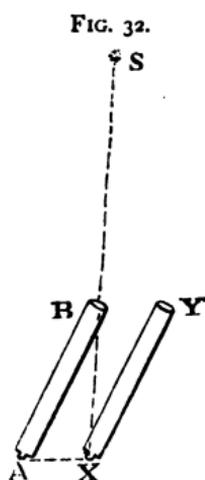
the telescope will move from the position marked *AB* to the position *XY* in the same time as the light from the star travels from *B* to *x*.
