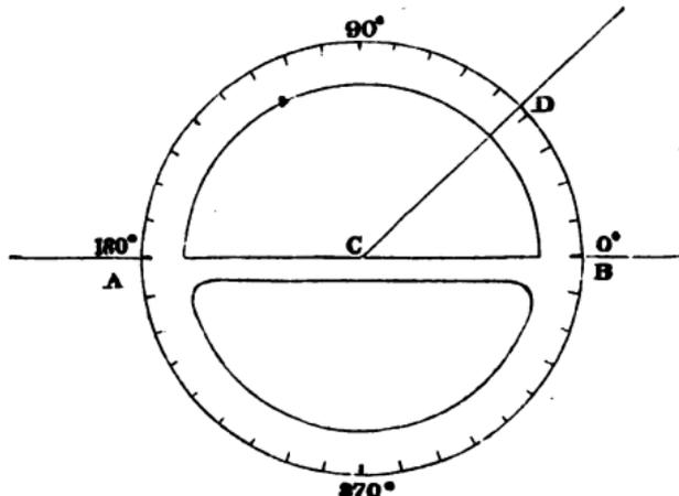
There is, however, no difficulty in finding at a glance the number appropriate to any intermediate division. To facilitate this operation the divisions  $5^\circ$ ,  $15^\circ$ ,  $25^\circ$ , which are situated half-way between each of the numbered divisions, are sometimes marked with a longer line, so that they can be instantly recognised.
