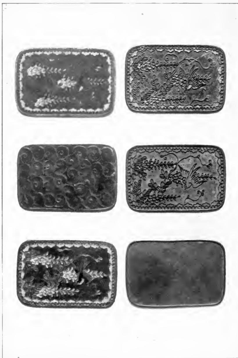
Fig. 140. Steps in process of "cloisonné" enameling.
