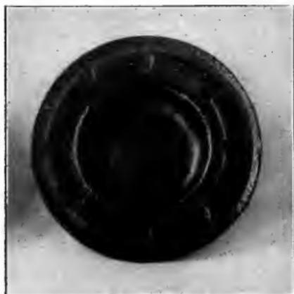
Fig. 129. Chased copper plate, showing an application of the method of beating down the background with the planisher chasing tools.
