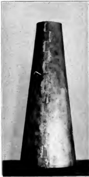
Fig. 123. "Cramped" seam vase ready for shaping.
