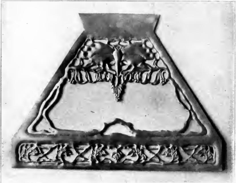
Fig. 76. Side of "dome" chased, and background cut out ready to bend in shape.
