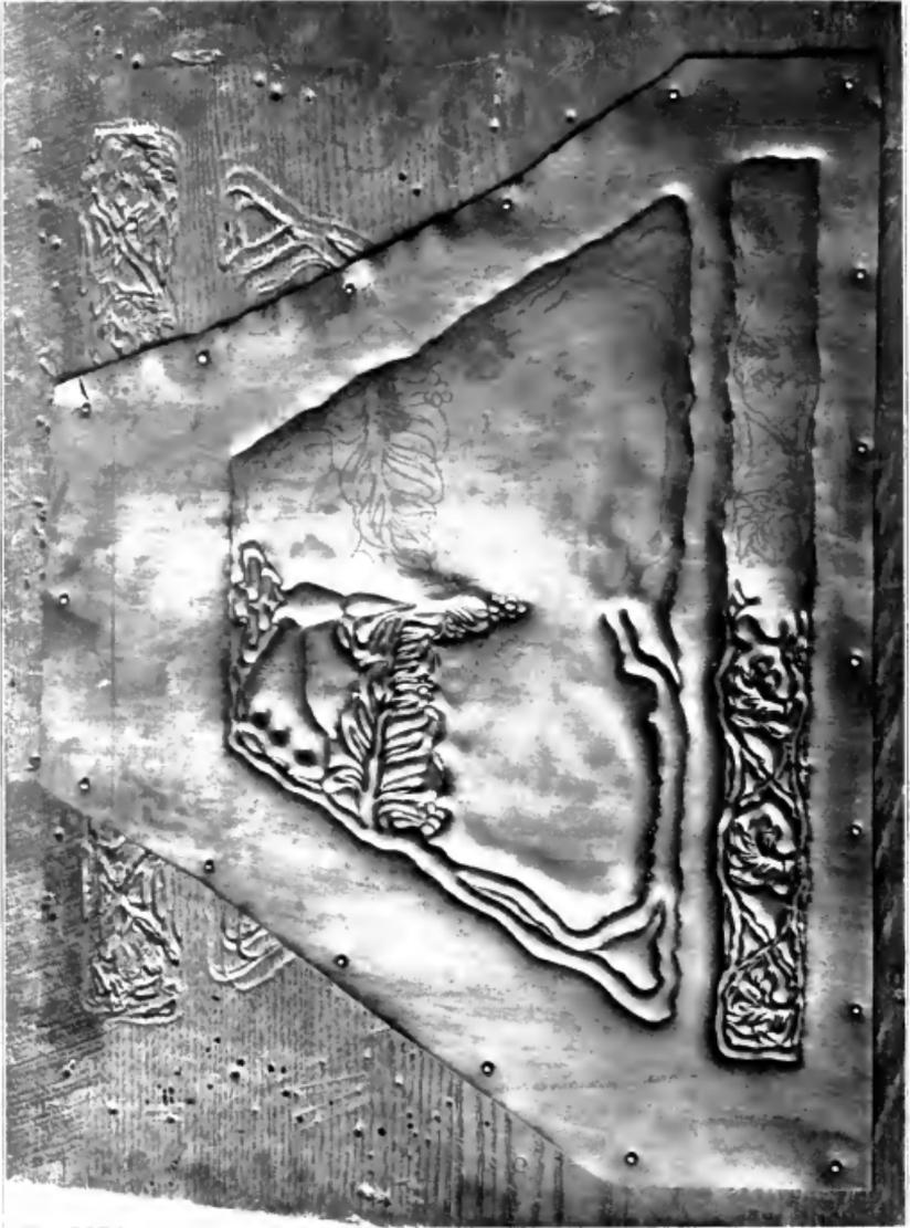
Fig. 74. One side of "dome" with design traced on, and one half "chased."
