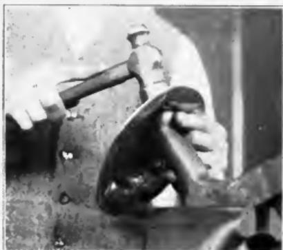
Fig. 65. Planishing the side of the plate.
