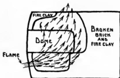
Fig. 149. Inside construction of home-made enameling muffle.
