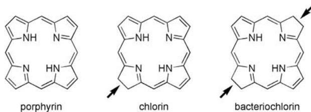
**Figure 11.7** The relationship between porphyrins, chlorins and bacteriochlorins
