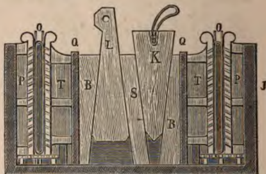
Fig. 37.—Wedge Press—Longitudinal Section of Lower Portion.
