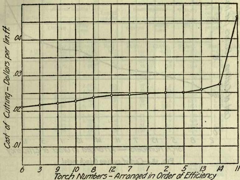
FIG. 36.—Cost of cutting 1/2-inch metal
