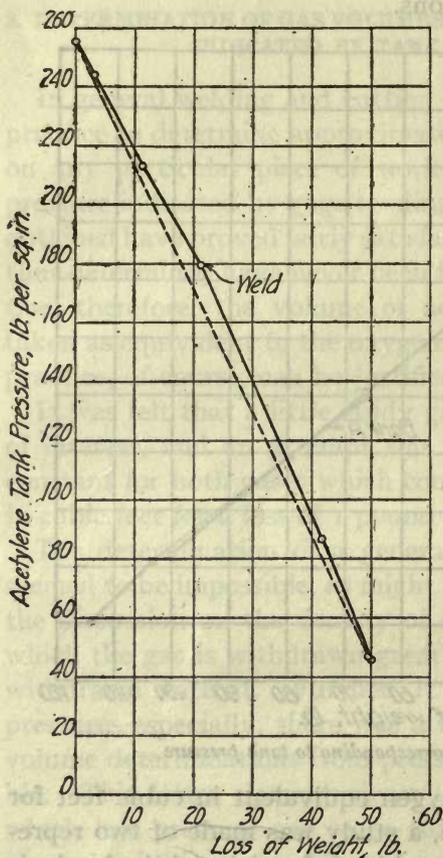
FIG. 15.—Loss of acetylene corresponding to gage pressure
