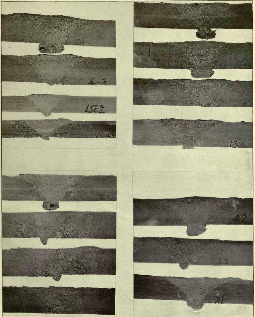
FIG. 71.—Etched sections through welds—Concluded
