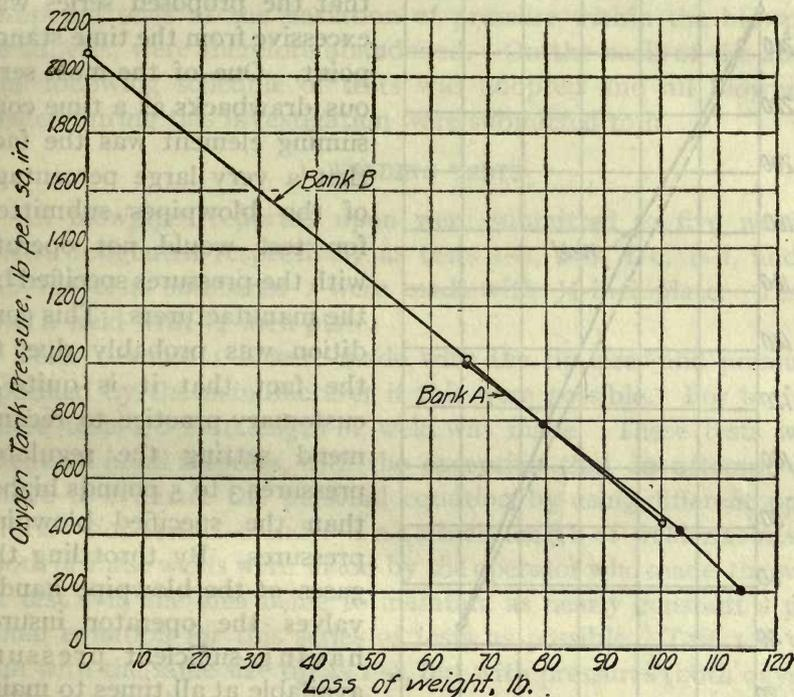
FIG. 14.—Loss of oxygen corresponding to tank pressure
