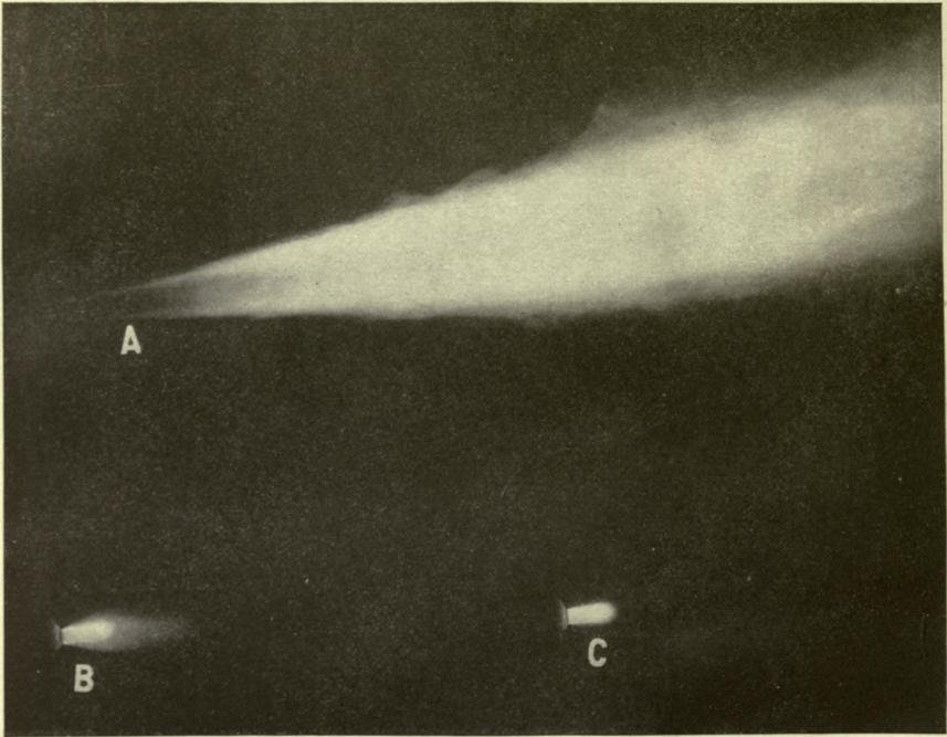
FIG. 64.—*Oxyacetylene flames*
