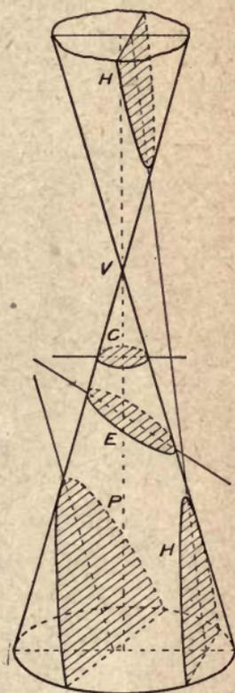
FIG. 88. — The conic sections.
