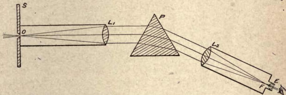
FIG. 139. — A spectroscope having only one prism.
