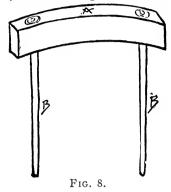
piece of wood (A) 4 inches in height, 2 feet long and about 4 inches thick, hollowed out so as to fit the circumference of the circle. Through this plank (A) pass rods of halfinch iron, B, B, sharpened at the bottom end. When needed for use these pins are driven into the ground until the inside face of the plank is just even with the circumference of the circle, making a firm obstacle, against which the putter can kick his forward
