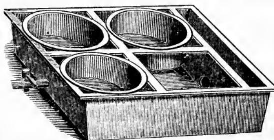
This is an instrument for testing the value and quality of milk. It will tell if milk has been skimmed, watered, or taken from a cow that has garget or any other disease that will affect the quality of the milk. It is simple in construction and operation, and is rapidly going into use in the best Butter and Cheese Factories in the country.
