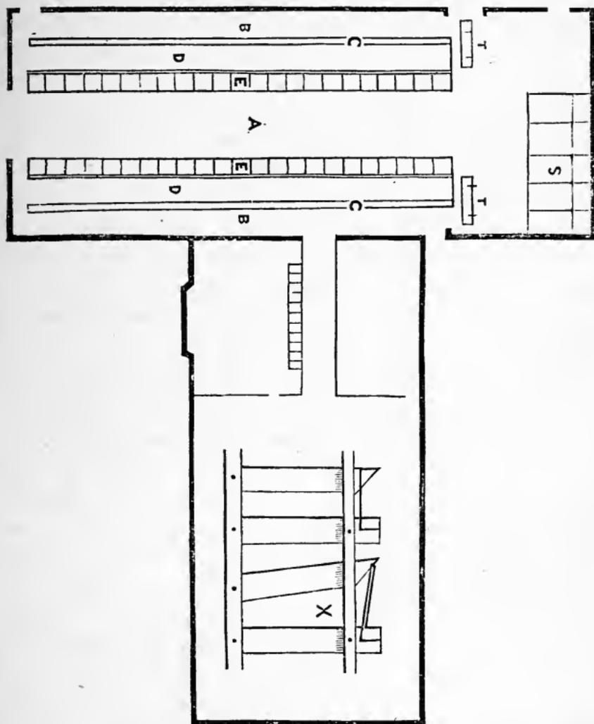
The mangers, E E, are two feet in the clear, with the bottoms raised four inches above the feet of the cow. A separate feed-box is made for each cow. It is formed by boarding up in front 16 or 18 inches, and separating their heads with a partition of two inch plank. The
