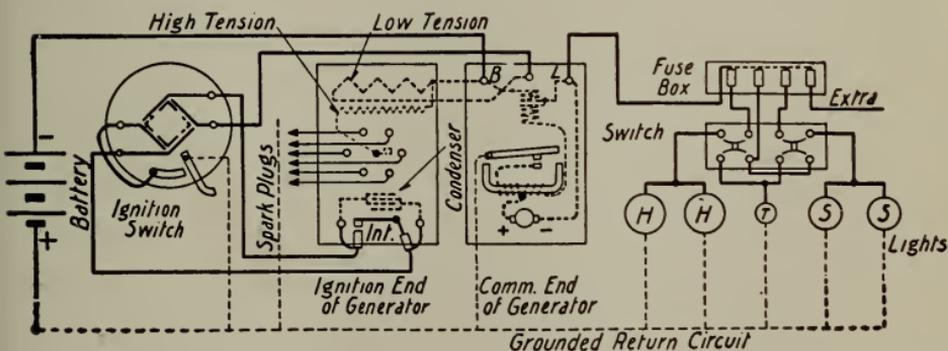
Fig. 296.—Lighting and ignition system.
