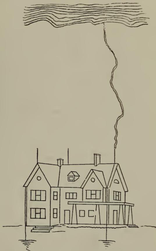
Fig. 37.—Charge equalized by lightning flash.
