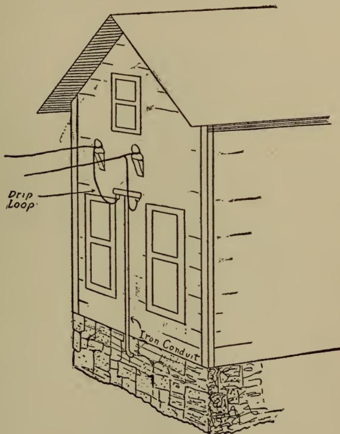
Fig. 276.—How wires are brought into house.
