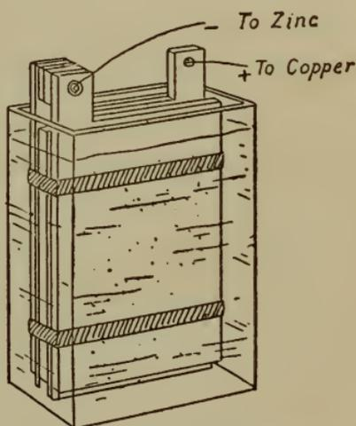
Fig. 63.—Storage cell assembled.
