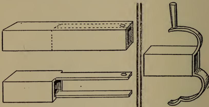
Fig. 241.—A slider that is easy to make.
