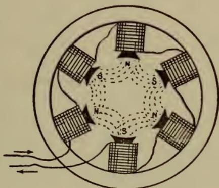
Fig. 143.—Six-pole field winding showing magnetic circuits.
