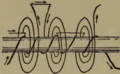
Fig. 103.—Diagram showing direction of coil windings.
