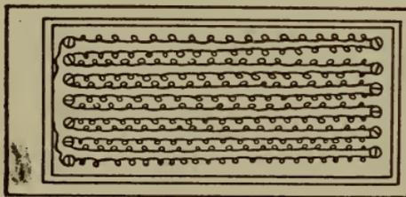
Fig. 121.—How the toaster is wired.
