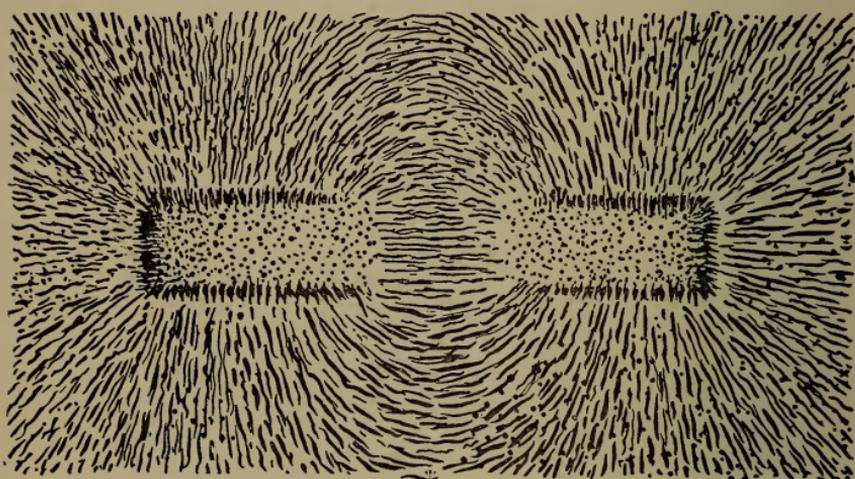
Fig. 10.—Magnetic field of bar magnet.
