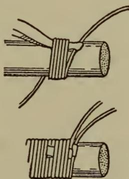
Fig. 98.—How wire is held in place.
