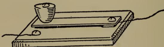
Fig. 138.—Switch for dark-room lamp.
