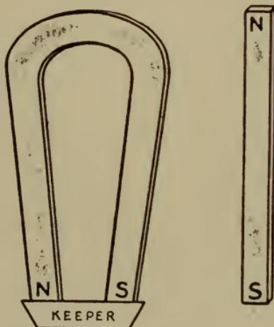
FIG. 3.—Horseshoe magnet and bar magnet.
