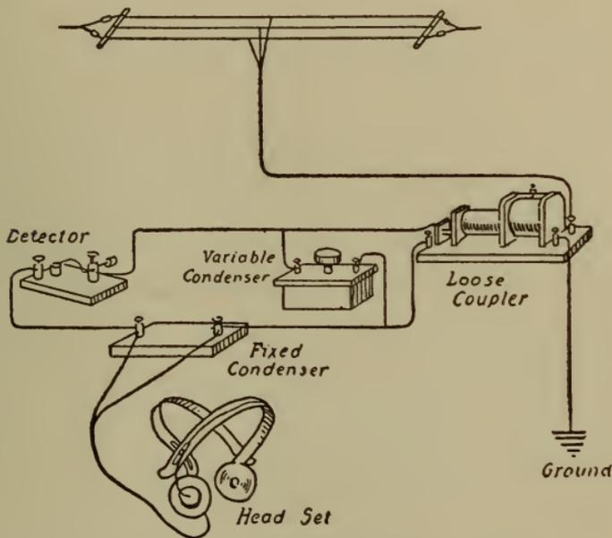
Fig. 227.—Tuned receiving set, loose coupled.
