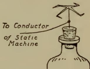
Fig. 31.—Static electric motor.
