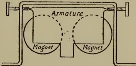
Fig. 189.—How relay armature is pivoted.
