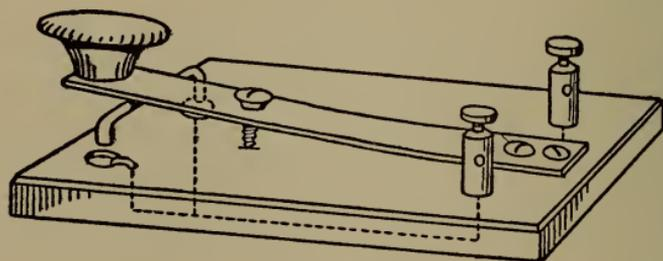
Fig. 250.—Sending key for heavy current.
