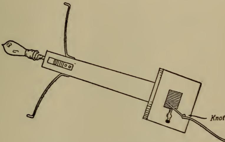
Fig. 303.—How cord runs to lamp.
