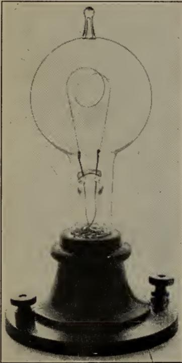
Fig. 128.—Edison's first electric lamp.
