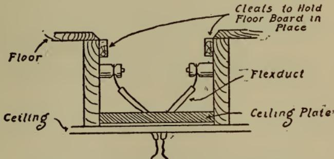
Fig. 272.—Ceiling plate in place at outlet.
