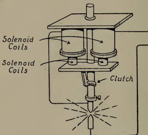
Fig. 125.—Principle of arc lamp.
