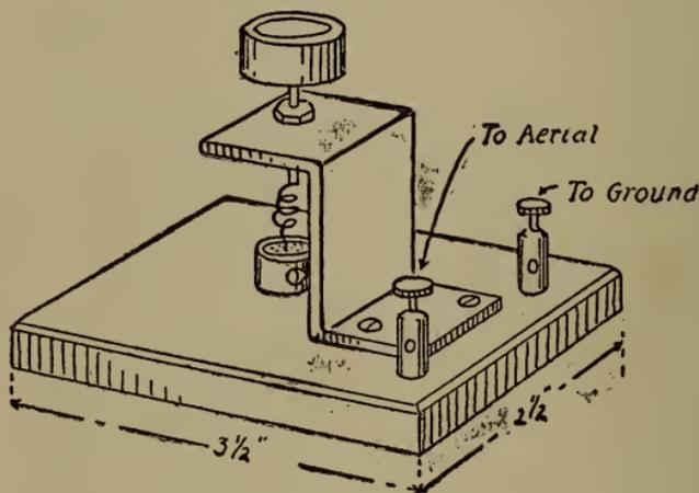
Fig. 237.—Silicon detector.
