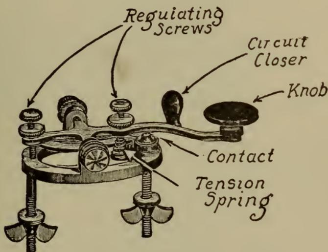
Fig. 173.—Standard type of key.
