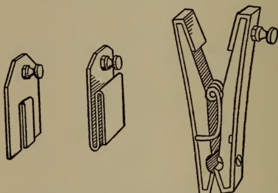
Fig. 253.—Easily made helix clips.
