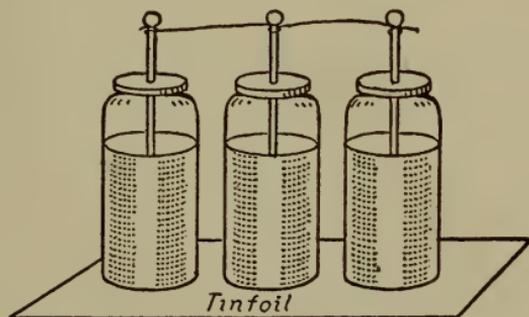
Fig. 29.—Parallel connection.
