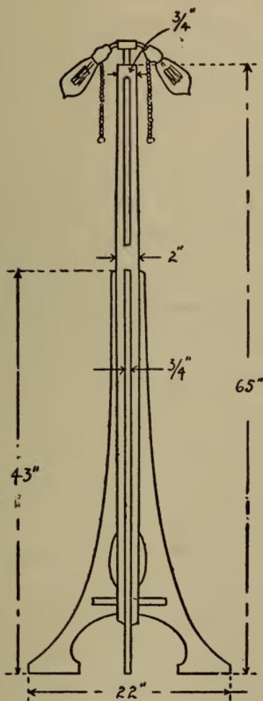
Fig. 312.—Dimensions of piano lamp.
