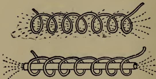
Fig. 72.—Coil without and with an iron core.
