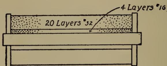
Fig. 217.—Induction-coil for microphone or telephone.
