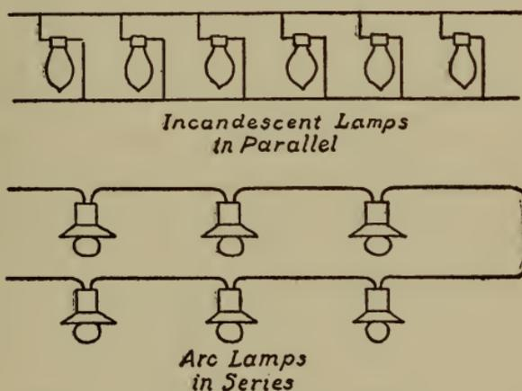
Fig. 67.—Series and parallel lighting circuits.
