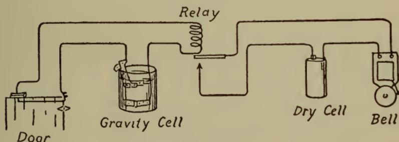
Fig. 89.—Wiring for burglar alarm.
