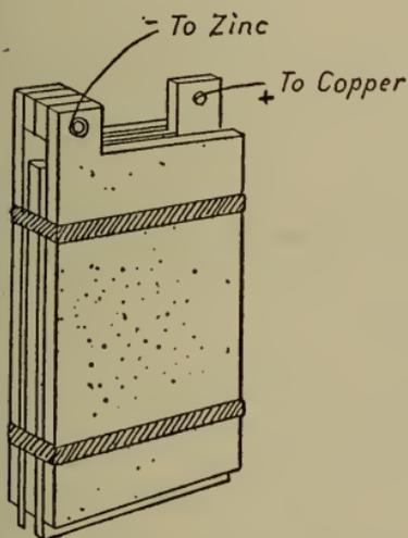
Fig. 62.—Lead plates completed, with separators between.
