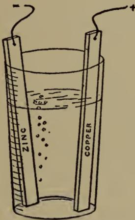
Fig. 42.—Cell when current is not flowing.
