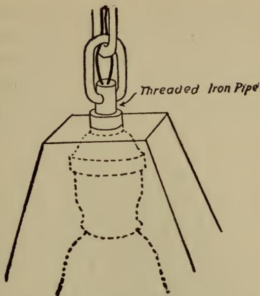
Fig. 307.—How shade is fastened to chain.
