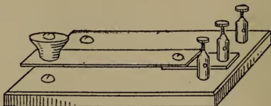
Fig. 186.—Two-way switch.
