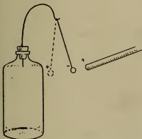
Fig. 23.—Pith-ball electroscope.
