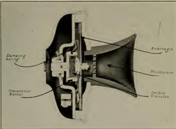
Fig. 196.—Parts of modern telephone transmitter.
