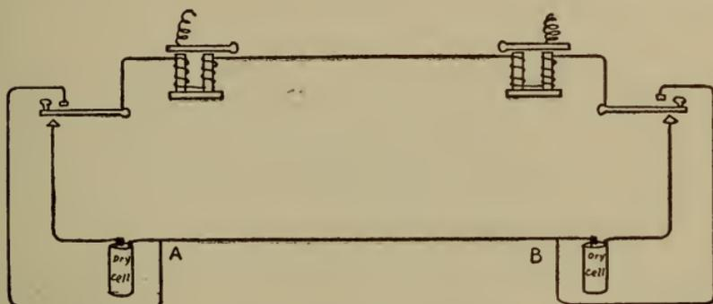
Fig. 181.—Circuit with two keys and two sounders.
