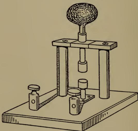
Fig. 258.—Vertical spark-gap.
