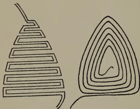
Fig. 114.—Heating elements for flat-irons.
