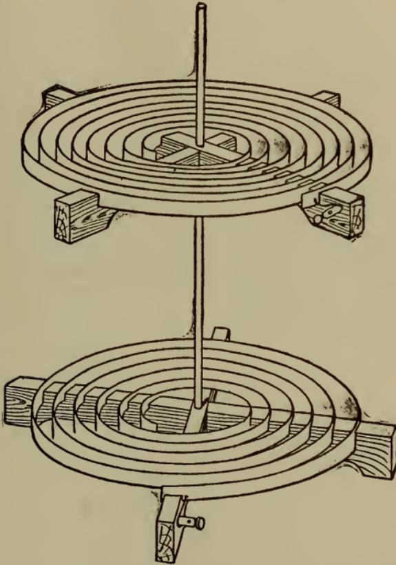
Fig. 252.—Oscillation transformer for closer tuning.
