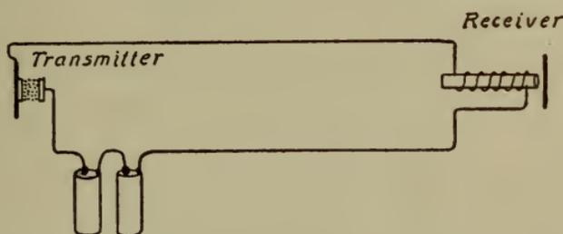
Fig. 195.—Simple circuit with microphone transmitter.
