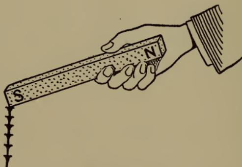
Fig. 13.—Magnetism by induction.
