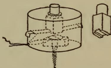
Fig. 84.—A push-button made from a pill box.
