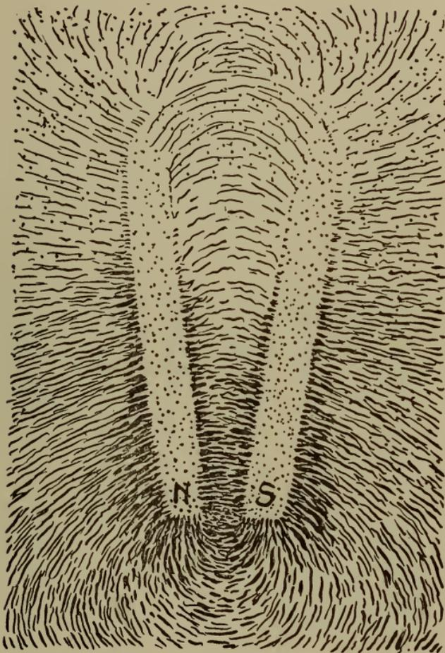
Fig. 11.—Magnetic field of horseshoe magnet.
