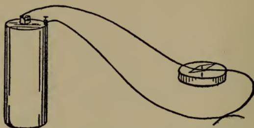
Fig. 69.—Current directs a magnet needle.
