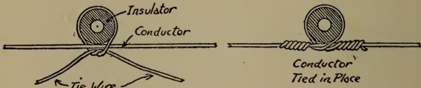
Fig. 271.—How to tie wire to knobs.
