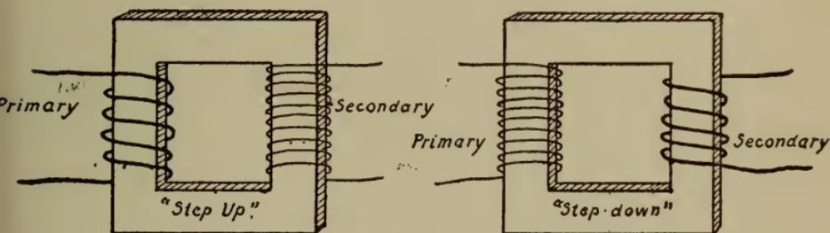
Fig. 149.—How transformers are wound.
