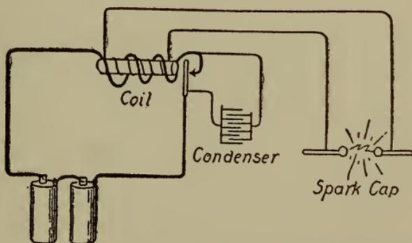
Fig. 108.—Connections for induction-coil and spark gap.
