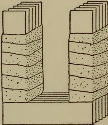
Fig. 154.—How sheet is cut for transformer.
