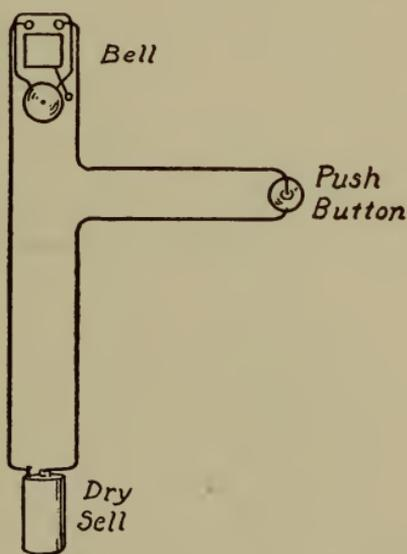
Fig. 74.—Simple electric bell circuit.
