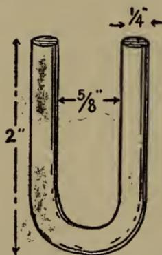
Fig. 75.—Magnet core for bell.
