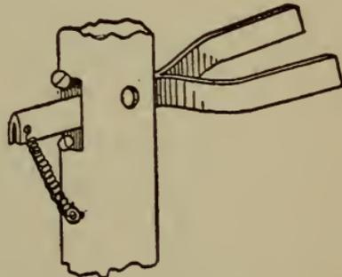
Fig. 208.—Detail of hook and connection.
