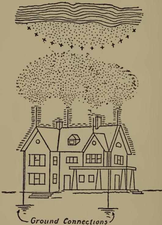
Fig. 36.—Field of static charge around a well-rodged house.
