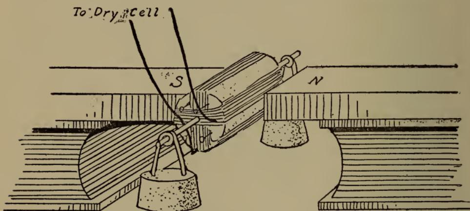
Fig. 166.—Complete "cork" motor.
