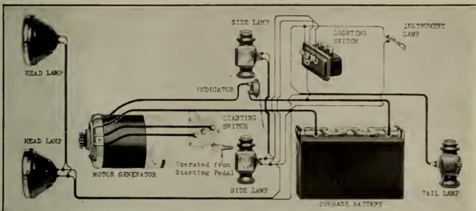
Fig. 295.—How an automobile is wired.
