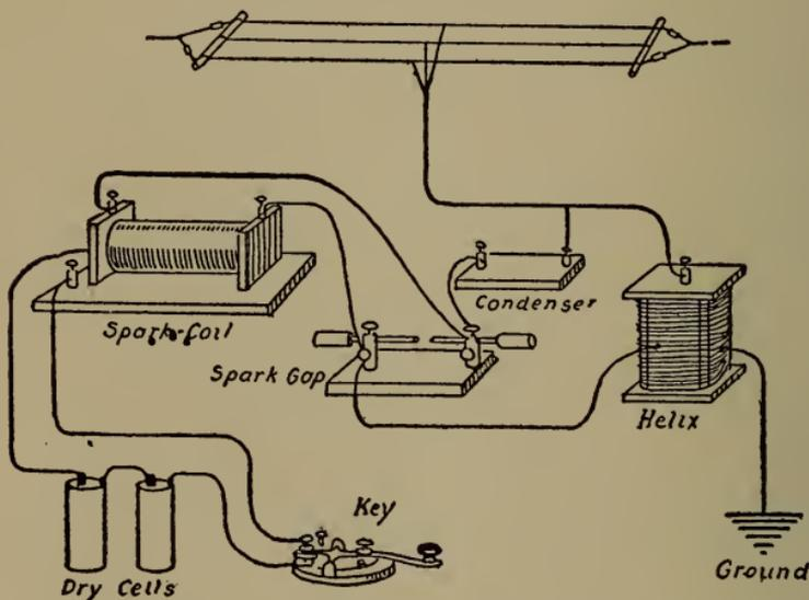
Fig. 226.—Tuned transmitting set, close coupled.
