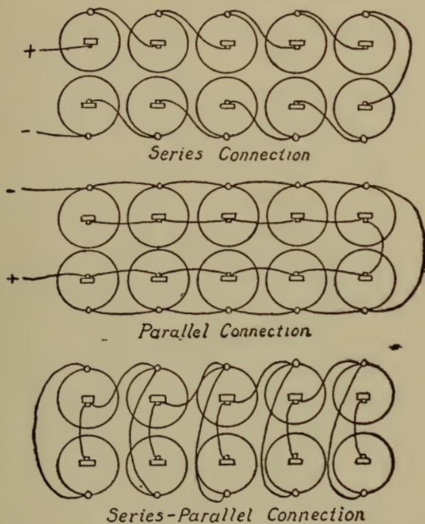
Fig. 58.—Connections for dry cells.
