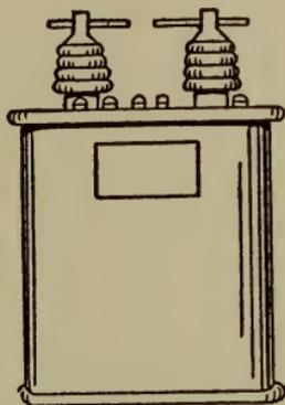
Fig. 256.—Transformer used for wireless.
