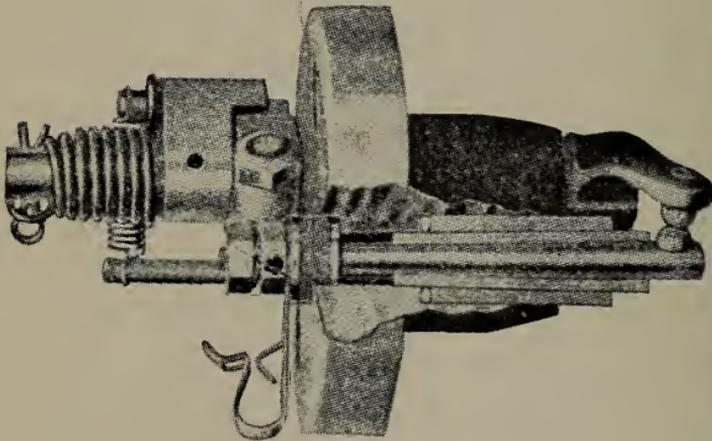
Fig. 287.—Make-and-break igniter.
