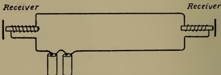
Fig. 194.—How Bell's first telephone was wired.
