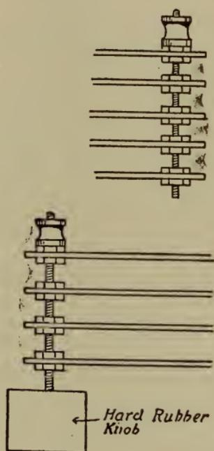
Fig. 247.—How plates are assembled.
