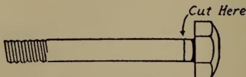
Fig. 85.—Bolt for magnet core.
