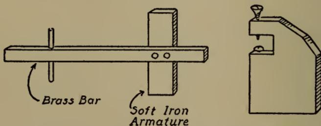
Fig. 184.—Armature and anvil of complete set.
