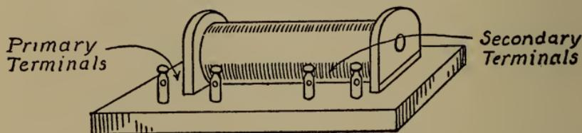
Fig. 218.—Finished induction-coil.
