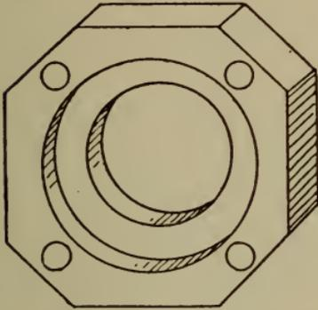
Fig. 205.—Front half of transmitter case.
