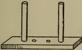
Fig. 178.—Field structure for telegraph sounder.
