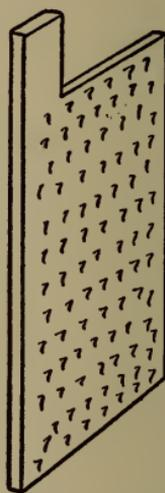
Fig. 61.—Plate prepared for red lead paste.
