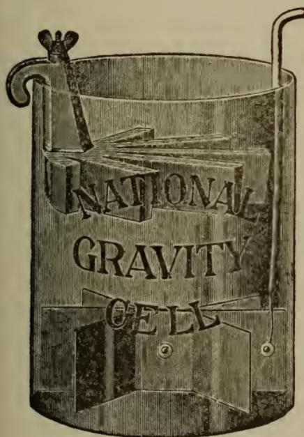
Fig. 46.—Gravity cell.
