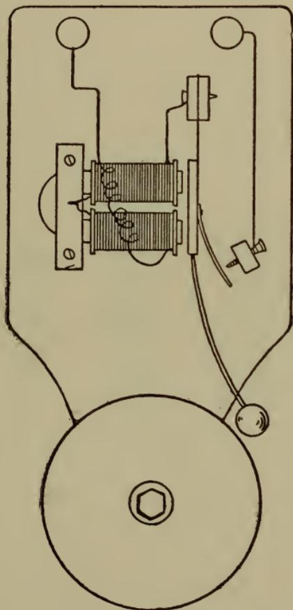
Fig. 80.—Inside of electric bell.
