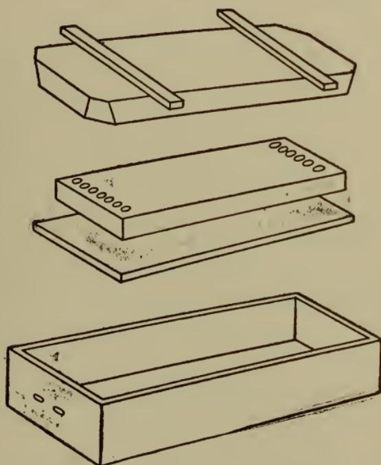
Fig. 119.—Mold for casting cement toaster base.
