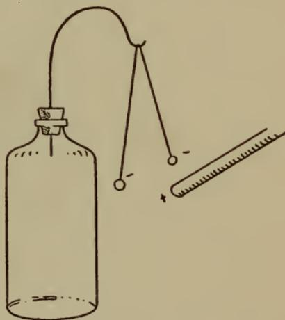
Fig. 24.—Electroscope with two pith balls.
