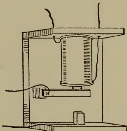
Fig. 86.—How alarm relay is wired.
