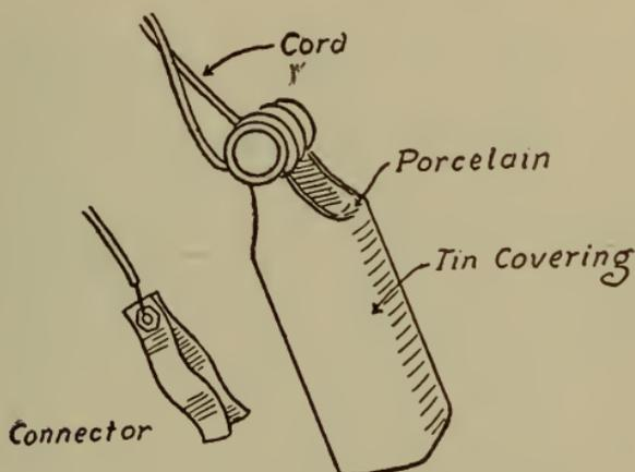
Fig. 115.—One style of flat-iron connector.
