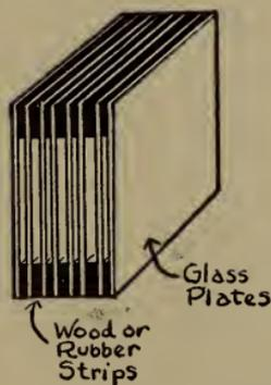
Fig. 245.—Glass plates assembled with separating strips between.
