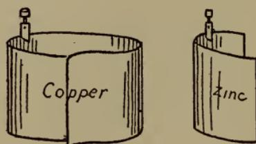
Fig. 50.—Copper electrode for Daniell cell and zinc for Leclanche cell.
