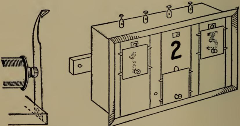
Fig. 91.—Catch for annunciator drop.
