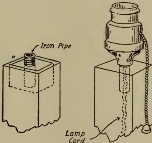
Fig. 301.—Mounting the socket on the standard.
