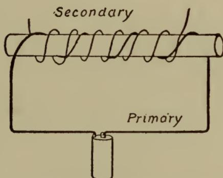
Fig. 96.—Connections of an induction-coil.
