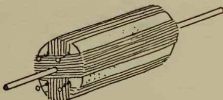
Fig. 165.—Cork armature of motor.
