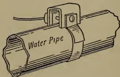
Fig. 187.—A convenient ground clamp for water pipes.
