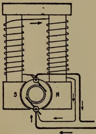
Fig. 144.—Shunt-wound generator.
