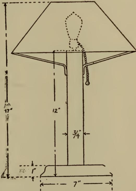
Fig. 305.—Dimensions of table lamp.
