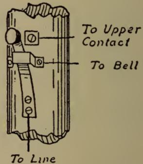
Fig. 210.—Detail of bell-ringing switch.
