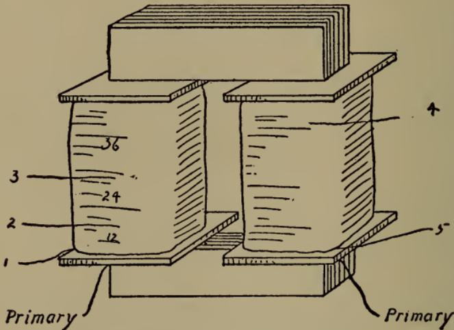
Fig. 157.—Transformer assembled.
