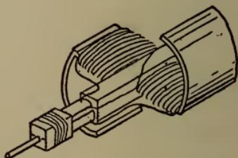
Fig. 171.—Complete armature.
