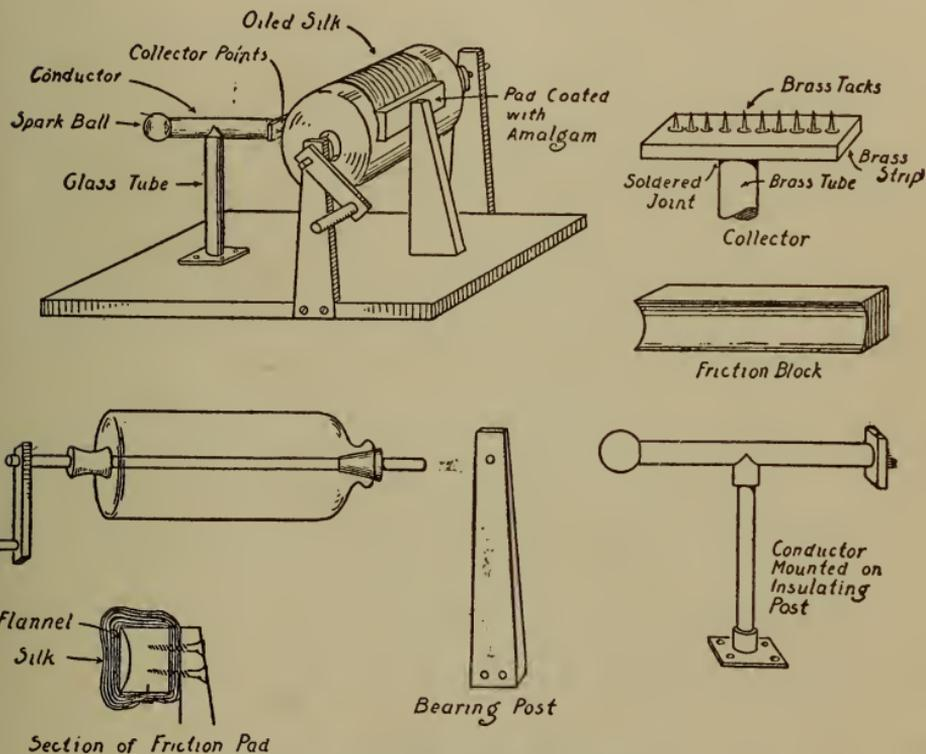
Fig. 27.—Cylinder electric machine.
