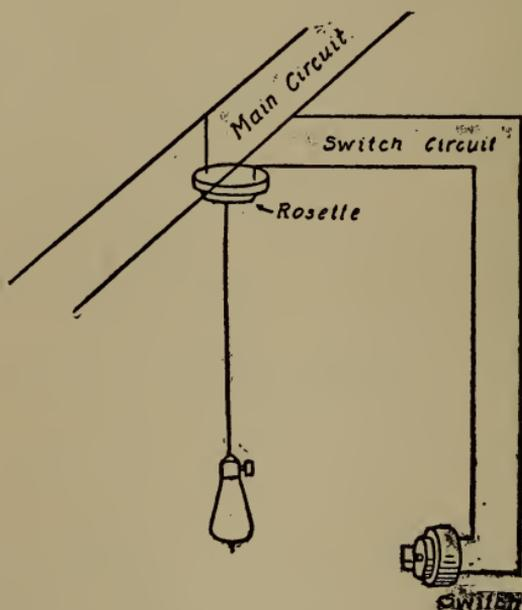
Fig. 273.—Connections for lamp and wall switch.
