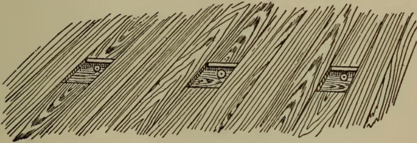
Fig. 268.—Knob work with pockets cut.
