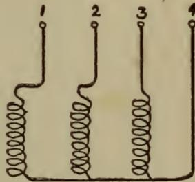
Fig. 94.—Annunciator connections.
