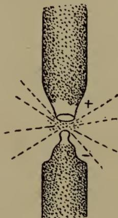
Fig. 123.—Direct current arc.
