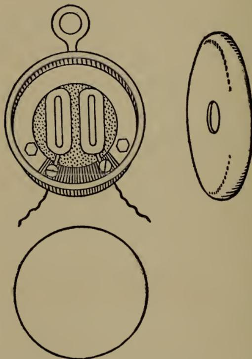
Fig. 214.—Parts of watch-case receiver.
