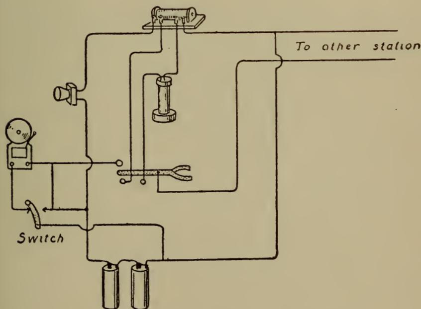
Fig. 220.—Telephone circuit with induction-coil.
