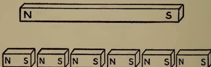
Fig. 15.—Many magnets could be made from one.
