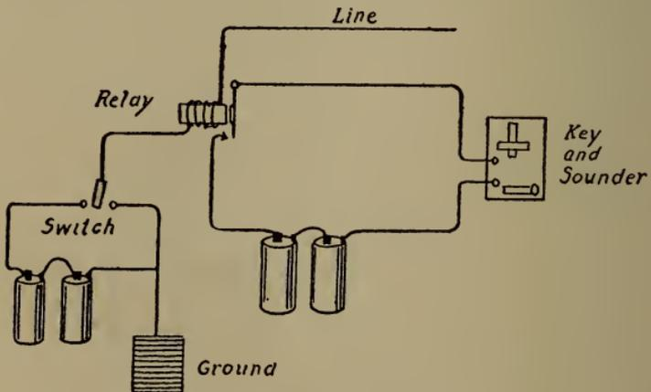
Fig. 191.—Connection for receiving with relay.
