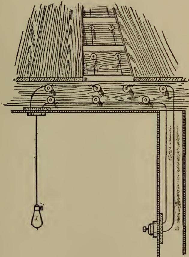
Fig. 274.—Lamp and wall switch installed.
