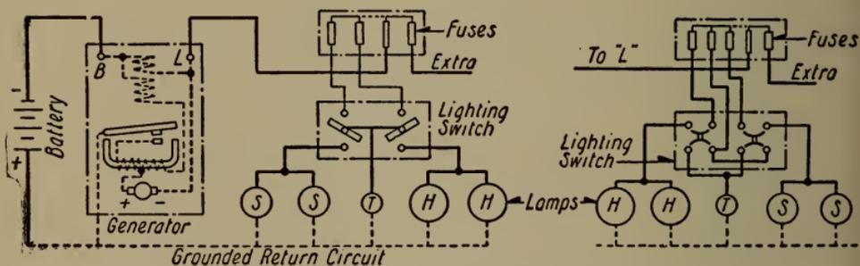
Fig. 294.—How automobile lights are wired.
