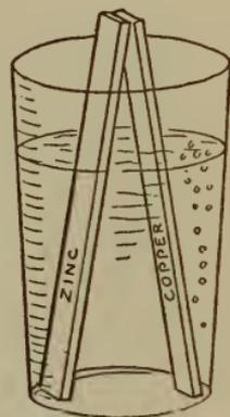
Fig. 41.—A simple zinc-copper cell.
