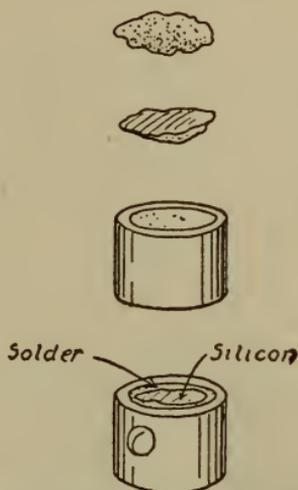
Fig. 238.—Cup of silicon detector.
