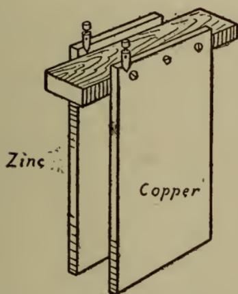
Fig. 54.—Mounting plate metal electrodes.
