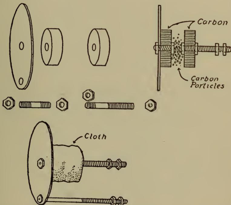
Fig. 203.—Parts and method of constructing telephone transmitter.
