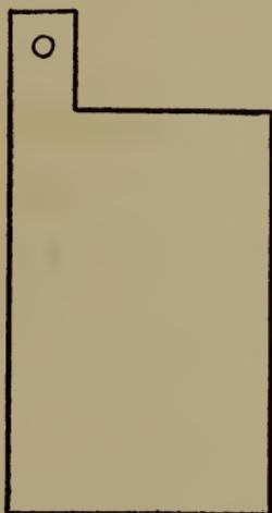
Fig. 60.—Lead sheet for battery plate.
