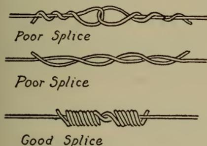
Fig. 83.—Wrong and right way of making splice.
