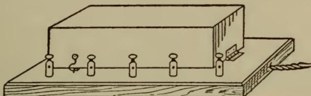
Fig. 161.—Toy transformer with cover in place.
