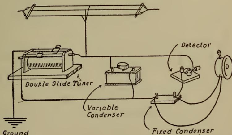
Fig. 225.—Receiving station arranged for tuning.
