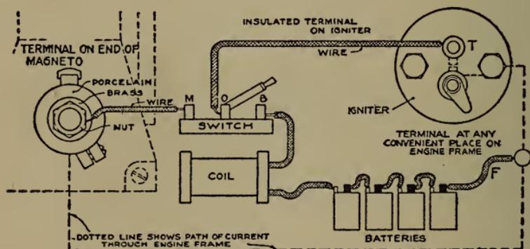
Fig. 291.—Wiring for both battery and magneto.
