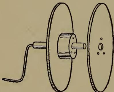
Fig. 99.—Section winder for induction-coil.
