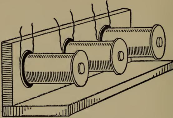
Fig. 90.—Magnets for annunciator.
