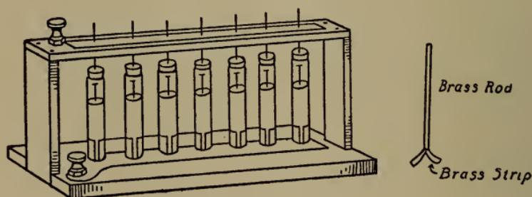
Fig. 255.—Test-tube condenser.
