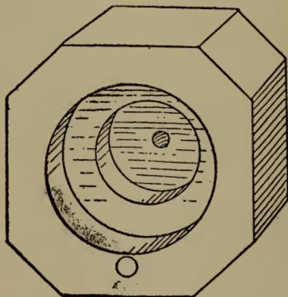
Fig. 204.—Back half of transmitter case.
