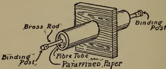
Fig. 234.—This lead-in is substantial and easily made.
