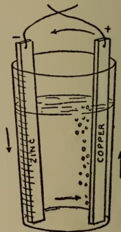
Fig. 43.—Cell when current is flowing.
