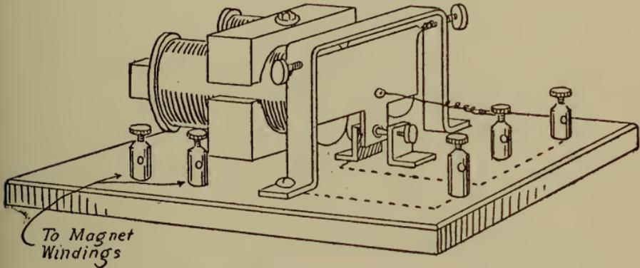
Fig. 188.—Telegraph relay.
