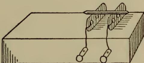
Fig. 215.—Microphone made from safety razor blades.
