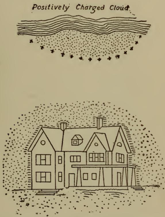
Fig. 35.—Field of static electricity around an unrodded house.
