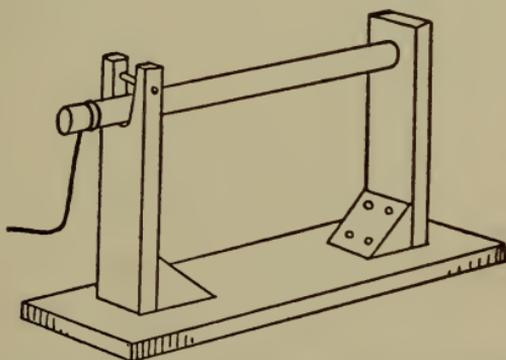
Fig. 77.—Windlass for winding wire on spools.
