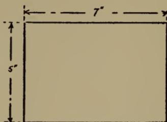
Fig. 244.—Glass plate for condenser.
