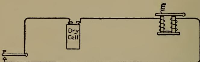
Fig. 176.—How key and sounder are wired.
