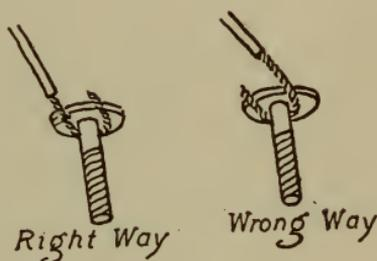
Fig. 118.—Right and wrong way of connecting wires.
