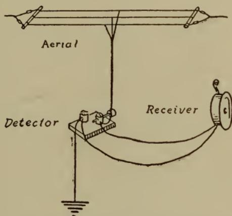
Fig. 223.—Simple receiving station.
