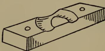
Fig. 79.—Block for holding magnet.
