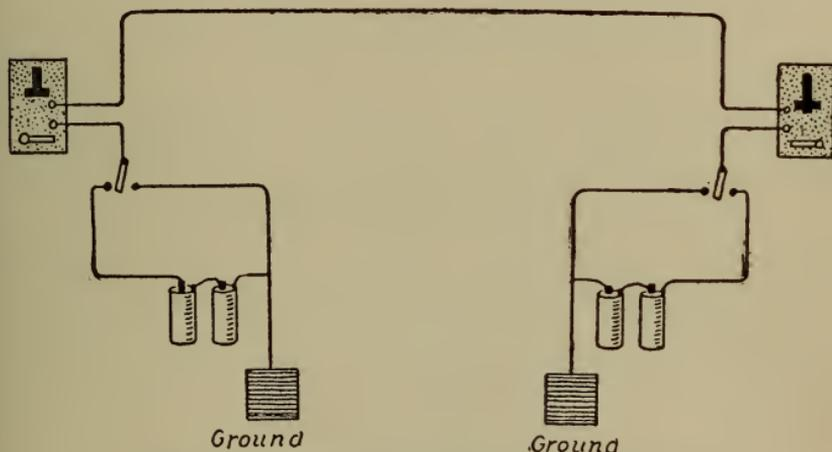
Fig. 185.—Circuit for two key and sounder sets.
