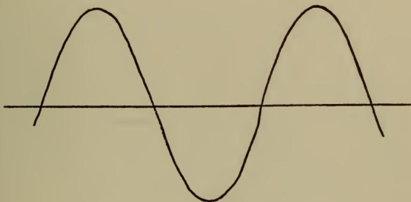
Fig. 148.—An alternating current wave.
