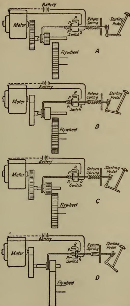
Fig. 297.—Electric starter operated with foot pedal.
