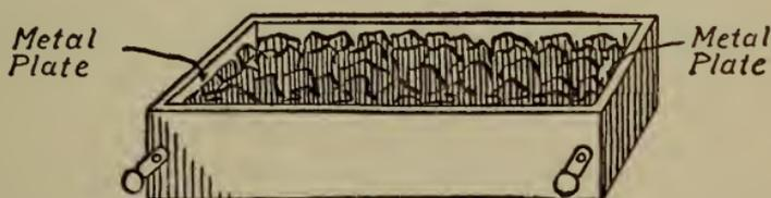
Fig. 216.—Multiple contact microphone made with broken coke.
