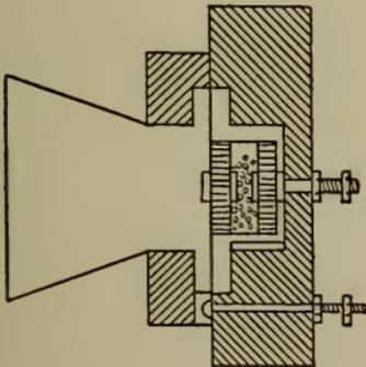
Fig. 207.—Section through assembled transmitter.
