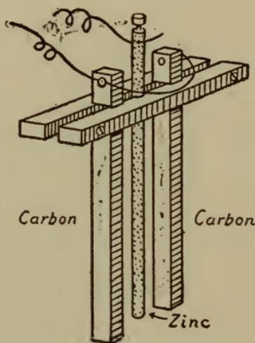
Fig. 55.—Mounting for carbons and zinc rod.
