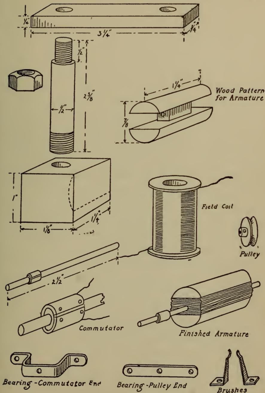
Fig. 150.—Parts of dynamo.
