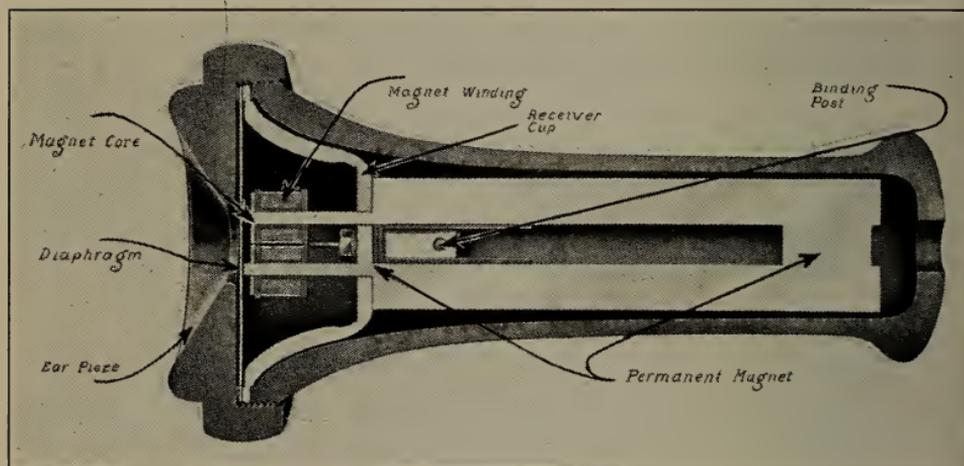
Fig. 197.—Parts of telephone receiver.
