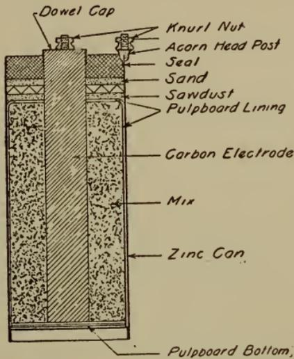
Fig. 49.—Inside of dry cell.
