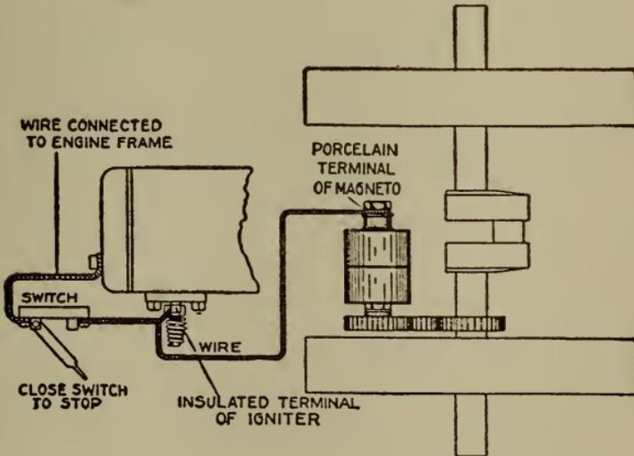
Fig. 290.—Connection for magneto with make-and-break ignition.
