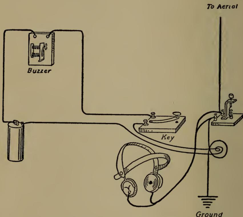
Fig. 259.—Buzzer connected to test detector adjustment.
