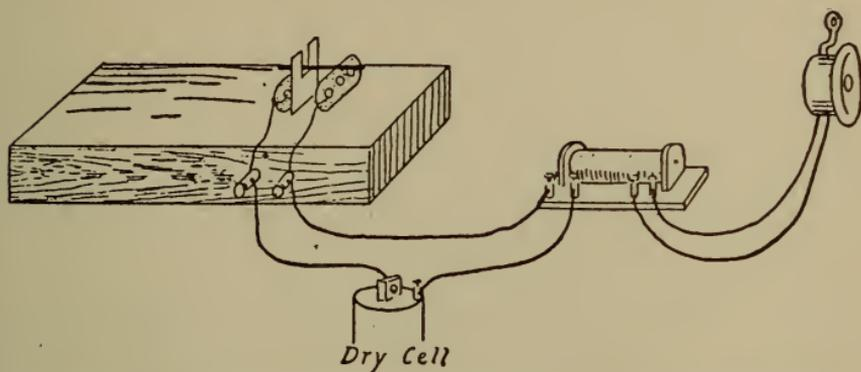
Fig. 219.—Connections of razor-blade microphone with induction-coil.
