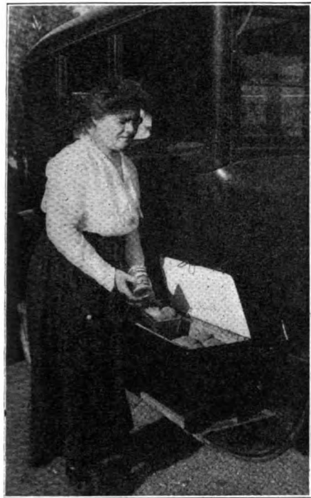
FIG. —THE "EATS" ARE COOKED IN THIS FIRELESS COOKER FROM THE HEAT THROWN OFF BY THE EXHAUST PIPE WITH WHICH IT IS CONNECTED
