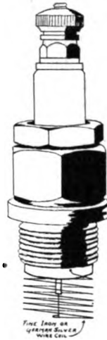
AN OLD SPARK PLUG AND A FEW INCHES OF FINE GER- MAN - SILVER WIRE ARE ALL THAT'S NEED- ED
