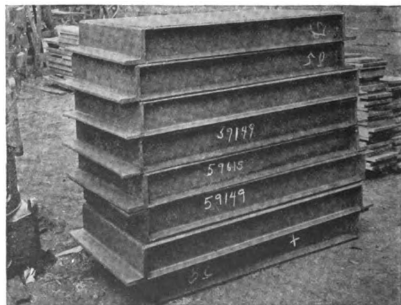
Fig. 115—Steel Machinery Bed-plates manufactured by use of the Arc Welder
