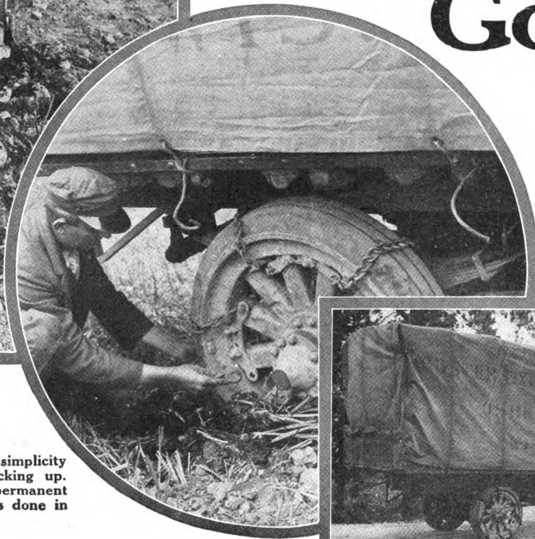
Note how the Giant Grip Chain bit into the ground and gave positive traction without any slippage.
