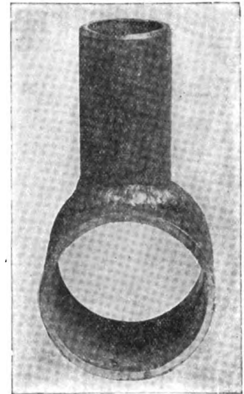
Fig. 118C. PIPE WELDING. See "Building Up Operation" for speed of work. The welded joint is stronger than the threaded joint. Steel or wrought iron pipe only may be welded.
