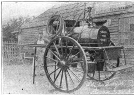
A Bush Fire Cart. An Australian bush fire is something of a proposition to combat and so the colonial government provides rather elaborate equipment. This picture shows Mr. T. H. Graham and a bush fire cart that he built from the ground up and is an excellent example of unusual work.
