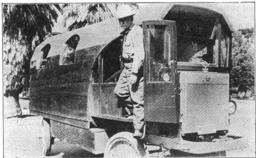
THE COMPLETED BODY WHICH WEIGHS 5,000 POUNDS IS CARRIED ON A FOUR WHEEL DRIVE TRUCK WHICH STEERS, DRIVES AND BRAKES ON ALL FOUR WHEELS
