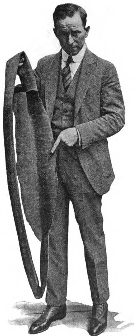
THINGS LIKE THIS HAPPEN JUST WHEN THEY'RE NOT WANTED TO. "PINCHED" INNER TUBES.
