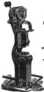
Hercules Patented Power Hammer. Weight of ram. 65 pounds.
