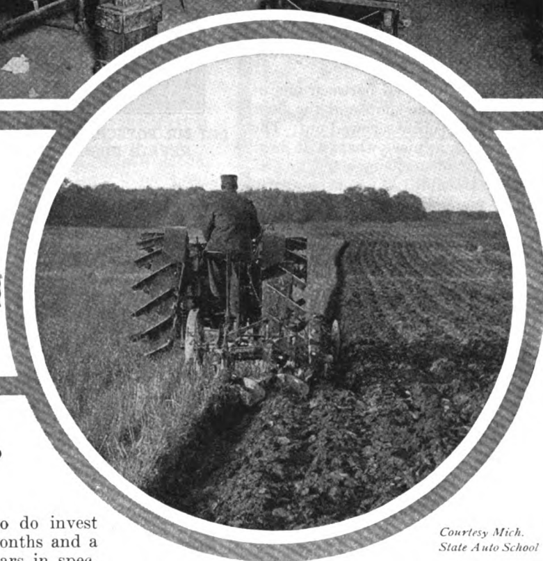
POWER PLANT OF TITAN 10-20 TRACTOR FIELD PRACTICE WITH TITAN TRACTOR AND THREE GANG PLOW
