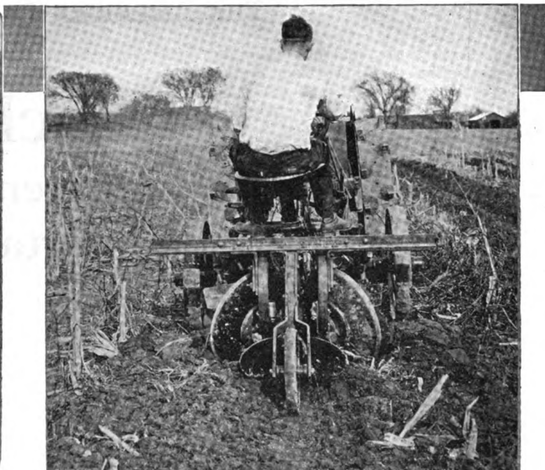
TRACTOR EQUIPPED FOR BREAKING UP SUGAR CANE STUBBLE.
