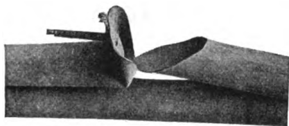
RIP CAUSED BY RUNNING ON FLAT TIRE.
