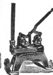
No. 4. American Tire and Axle Shrinker. Will shrink up to 4x1 inch round edge-tire, and axle up to 1 1/4 inch.
