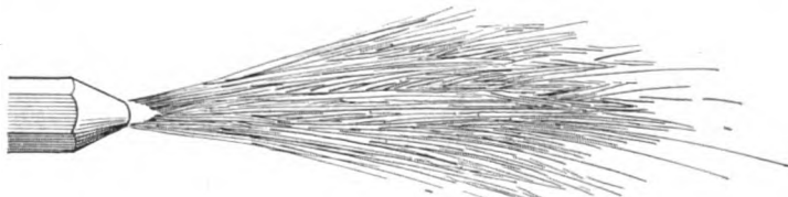
Too much oxygen in this flame, so it is termed an oxidizing one. Cone is shorter than in the above figure, more pointed and a different color, changing from the blue white to a darker blue. This flame is most easy to get and will ruin the weld.
