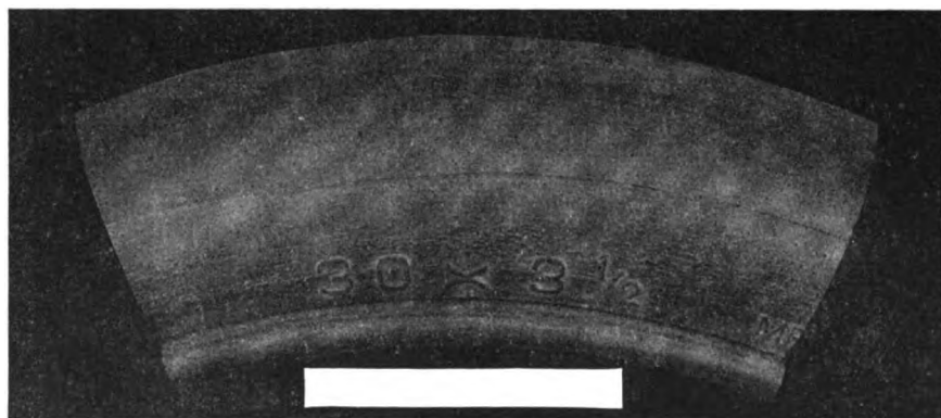
DETERIORATION:—CRACKED CONDITION OF RUBBER KNOWN AS "GUM CHECKING"
