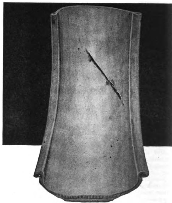
A fabric rupture which may have been started long before it was noticed. Caused by the breaking of a few threads of fabric resulting from a cut, severe bump, or bruise to the case. Internal pressure and weight on tire caused rupture to continue to break along bias of fabric
