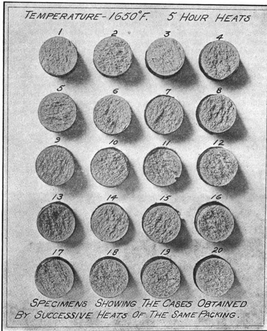
FIG. 5.—BROKEN SPECIMENS OF THE PIECES TREATED SHOWING THE CASE
