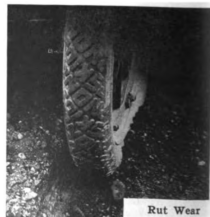
Abrasion by dirt and stones in making roadway
