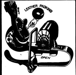
Placing the loop over the end of the cap and drawing the thumb lever back until it rests against the flat spring closes the coupler, keeps it closed, and takes up the wear of the leather packing.
