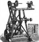
It is indispensable to blacks miths, wagon makers, wood workers and farmers. Consists of a two-cycle gasoline engine, running a rip saw, emery grinder, drilling and turning lathe and countershaft for running other machinery.
