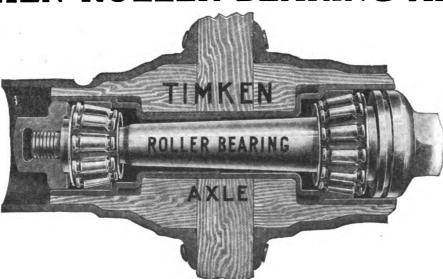
THE CAGE, made of stamped steel in one piece, insures perfect alignment, dispensing with the small nibs on the end of the rollers, reducing breakage under the severest strain to a minimum.
