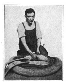
FIG. 1—INSERTING THE SHORT-STEMMED TIRE LUGS
