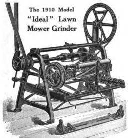
grinds the Reel Knives to fit the straight blade, even if the latter is bent and out of shape—something never done before, and the most important feature of Lawnmower sharpening. Has 5 in. ball bearing grinding wheel, ground and polished shaft, babbited bearings, twice as easy running as any other. Grinds either right or left hand Mowers perfectly in 15 minutes, without removing ratchets or wheels. We are the originators, and seven years' experience has shown us how to make them perfect.
