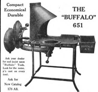
The heavy cast iron fire pan is mounted upon wrought iron legs rigidly braced. This produces a forge of great strength.
