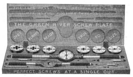
The dies are in two equal parts; the screws acting as a gauge, bring the dies *central* and thus *distribute the work equally* on the *four* cutting edges.
