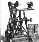
It is indispensable to blacks miths, wagon makers, wood workers and farmers. Consists of a two-cycle gasoline engine, running a rip saw, emery grinder, drilling and turning lathe and countershaft for running other machinery.
