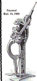
The only Calking Machine that with one pull of lever makes a heel calk complete, blunt or sharp, also makes double kink for the famous block calk, or sharpens side calk, with one pull of lever, welds blunt or sharp toe calks and forms toe clip with one pull of lever, also, has a shear to cut off either end of shoe.
