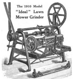
grinds the Reel Knives to fit the straight blade, even if the latter is bent and out of shape—something never done before, and the most important feature of Lawnmower sharpening. Has 5 in. ball-bearing grinding wheel, ground and polished shaft, babbited bearings, twice as easy running as any other. Grinds either right or left hand Mowers perfectly in 15 minutes, without removing ratchets or wheels. We see the originators, and seven years' experience has shown us how to make them perfect.
