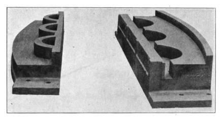
FIG. 1. FOR FORMING TANK SUPPORTS ON THE NEW STEEL CARS
