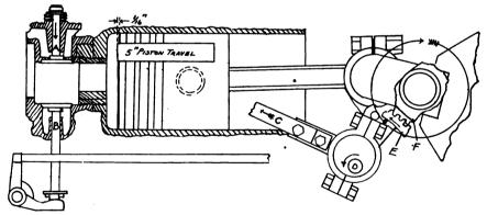
FIG. 1.—THE BEGINNING OF THE FIRST OR SUCTION STROKE
