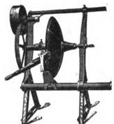
Can shear any part of edge to any bevel.
