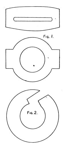
FIG. 1 AND 2.—FORGING RINGS AND LARGE NUTS
