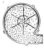
The outlet of the scroll shaped case is right in the path of the air currents, affording the easiest means of escape. All the air produced with each turn of the fan is delivered through the outlet. No air is carried past the opening and forced around the fan case a second time.
