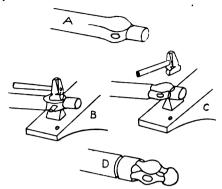
FIG. 1-SHOWING THE STEPS IN FORGING HAMMER
