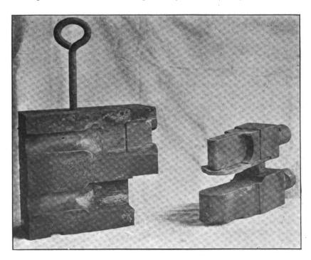
FIG. 4.—DIES AND PUNCHES THAT ARE USED FOR SCARFING AND WELDING
