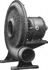
Efficient, because the scrollshaped fan case increases gradually in size as it approaches the discharge outlet, and the fan is built up with tapered, enclosed sides; allowing no churning of the air inside. Our blast gate gives perfect regulation. Write for particulars.
