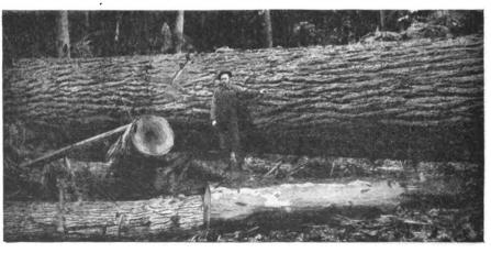
STEEL WEDGES ARE USED TO KEEP THE SAW FROM BINDING
