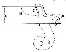
FIG. 4.—HOW TO FORGE A HAMMER
