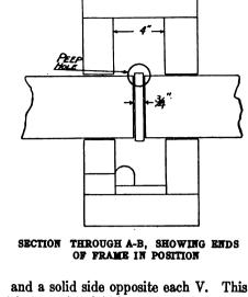
and a solid side opposite each V. This throws the laid-in pieces about six inches apart. This weld will elongate evenly when being reduced, and will not slip or shear, as the ordinary lap or V-weld will.
