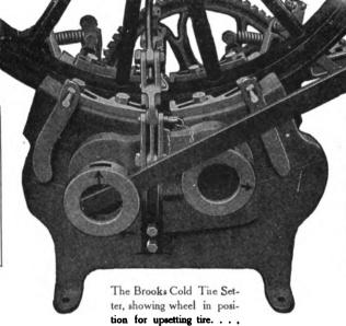
The Brooks sets the tire cold. No burnt surfaces to wear away. No steam and watersoaked felloes to shrink or split and loosen the tire. Simple, cheap, durable.
