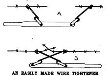
seven or eight inches apart. Then make two small clevises, like small plow clevises in shape, and bolt one to each hole in the bar so they will work freely. Then make two grabs for the barb wire of 3-inch round iron (horse rake teeth make good ones) about eight inches long when finished, with a large eye in the end connecting them to the clevises. To tighten wire, place grabs on wire, as shown at A, take hold of handle and
