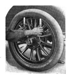
FIG. 1—ALLOW ALL AIR TO ESCAPE FROM TIRE TUBE
