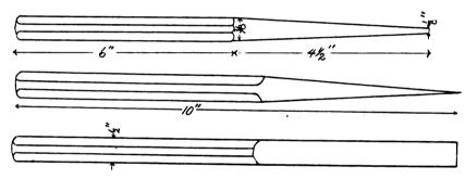
FIGS. 4 AND 5-A SLENDER PUNCH AND ALSO A COLD CHISEL ARE NEEDED
