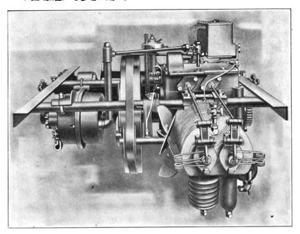
FIG. 2.—A FRONT VIEW OF THE INTERNATIONAL AUTO ENGINE
