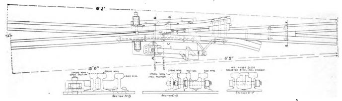
FIG. 4.—SHOWING PLANS AND SECTIONS OF SPRING RAIL FROG
