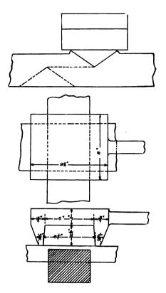
SHOWING CHANNEL TOOL AND METHOD OF USING WHEN WELDING
