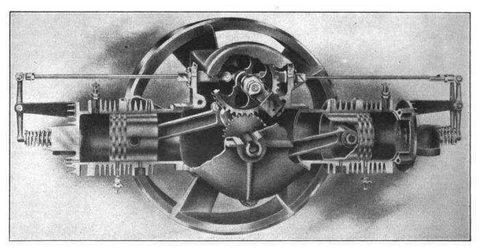
FIG. 2—THE BLACK MOTOR AND PARTS, SHOWING PARTS OF INTERIOR MECHANISM
