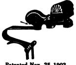
Patented Nov. 25, 1902 Patented June 11, 1907 The spring is pivoted at the front so that it can be turned out of the way of the wrench while clipping Coupling to the axle.
