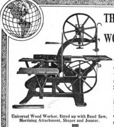
Universal Wood Worker, fitted up with Band Saw, Mortising Attachment, Shaper and Jointer.
