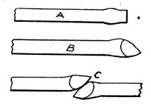
FIG. 8.—THE HALVES ARE THEN WELDED
