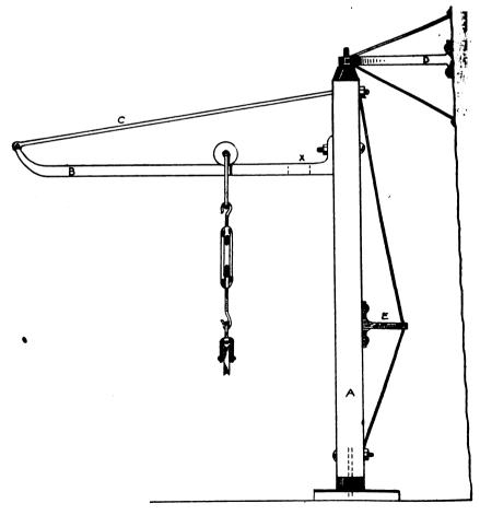
AN BASILY MADE CRANE FOR HANDLING HEAVY WORK
