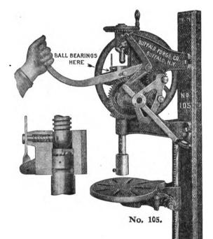
Ball Bearings Placed at the Point of Highest Speed.
