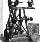
It is indispensable to blacks miths, wagon makers, wood workers and farmers. Consists of a two-cycle, gasoline engine, running a rip saw, emery grinder, drilling and turning lathe, and countershaft for running other machinery. Self contained, compact and portable. Weight, 165 lbs. \$55 complete,
