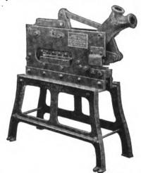
The frame is of armor plate, working parts of drop-forged steel, carefully machined and fitted. Knives and punches are of crucible steel, accurately fitted. The compound leverage gives ease of operation.
