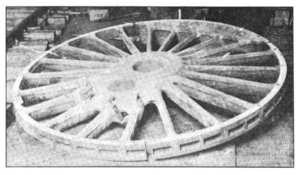
FIG. 2-FOUR OR FIVE SPOKES CAN BE WELDED AT ONE TIME
