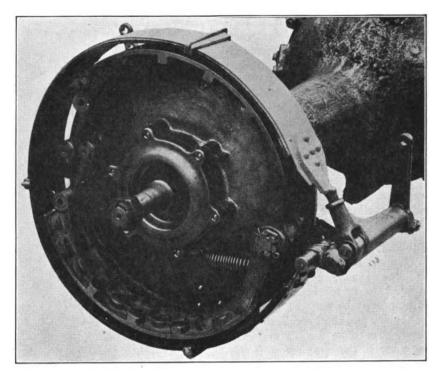
FIG. 5. BRAKE DRUM SHOWING BOTH INTERNAL AND EXTERNAL BRAKES
