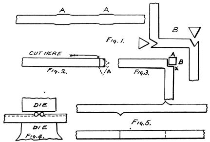
THERE ARE SEVERAL METHODS OF FORGING CRANK AXLES
