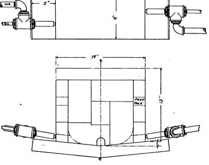
TOP VIEW AND AN END VIEW OF FRAME WELDING FURNACE
