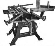
Universal Wood Worker, fitted up with the Single End Tenoning Attachment, with traveling table and hold down lever.
