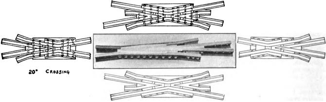
FIG. 5. SINGLE-RAIL BOLTED PLATE CROSSING WITH EASERS, ALSO A MANGANESE HARD CENTER FROG
