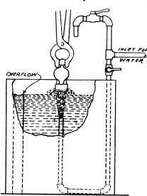
FIG. 2-THE BATH USED TO TEMPER A HAND HAMMER
