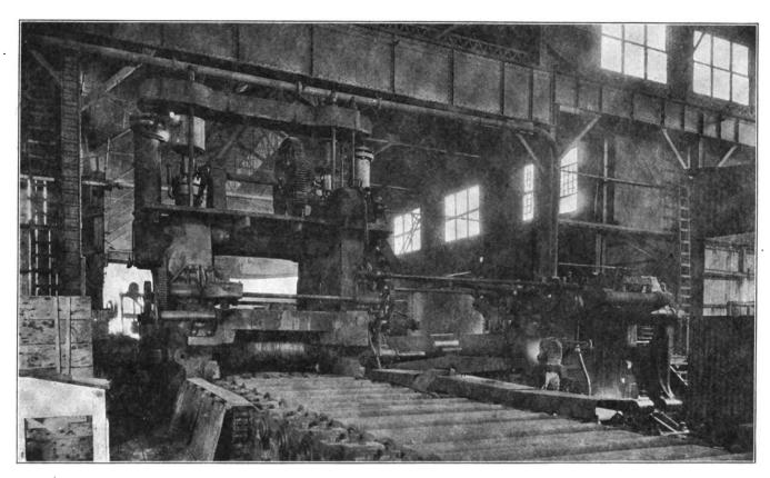
ONE OF THE ROLLERS WHICH CONVERTS INGOTS INTO PLATES
