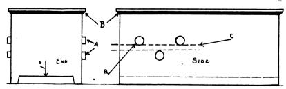
FIG. 1. - A PROPERLY CONSTRUCTED BOX FOR CASEHARDENING
