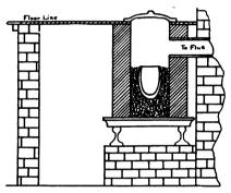
FIG. 6. SECTIONAL VIEW OF BRASS FURNACE
