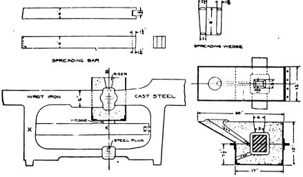
FIG. 1-BROKEN ENGINE FRAMES ARE QUICKLY REPAIRED WITH THERMIT
