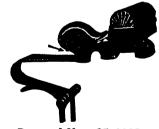
Patented Nov. 25, 1902 Patented June 11, 1907 The spring is pivoted at the front so that it can be turned out of the way of the wrench while clipping Coupling to the axle.
