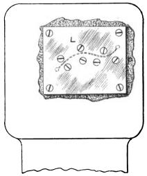
FIG. 1-REPAIRING A CRACKED CYLINDER
