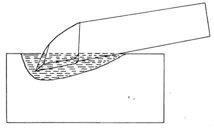
FIG. 7.—THE CORRECT METHOD OF DIPPING A SIDE TOOL
