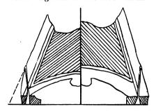
FIGS. 1 AND 2, SHOWING HALF CROSS SEC-TIONS OF CORRECTLY AND INCOR-RECTLY SHOD FOOT
