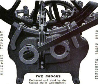
Fourth - The Draw-heads are constructed with lateral movement, so that they may always be in alignment with the tire, thus overcoming the chance of bending the tire edgewise.
