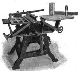
Universal Wood Worker, showing the Mortising Attachment and 27" band saw.
