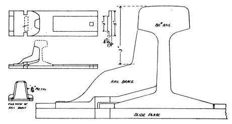
FIG. 2.—SOLID ROLLED SWITCH SLIDE AND MALLEABLE IRON BRACE
