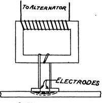
FIG. 3—FOR ANNEALING SPOTS IN ARMOR PLATE
