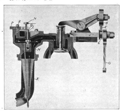
FIG. 5.-A SECTIONAL VIEW OF THE CADILLAC CARBURETOR
