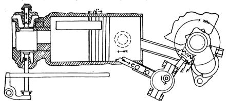
FIG. 2.—THE BEGINNING OF THE SECOND OR COMPRESSION STROKE
