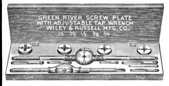
No. 1124. ¼ to ¾ inch. Stock 22 in. long. 5 sizes, ¼-20, ¾-16, ½-12, %-11, ¾-10, Taps, Dies and Guides, and Adjustable Tap Wrench, No. 58.
