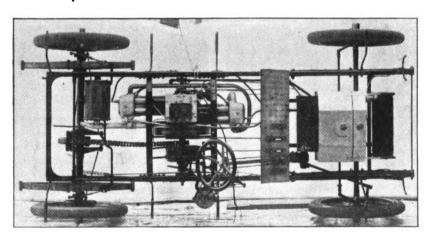
FIG. 6—ALL PARTS ARE NOW ACCESSIBLE. CHASSIS OF A REO CAR
