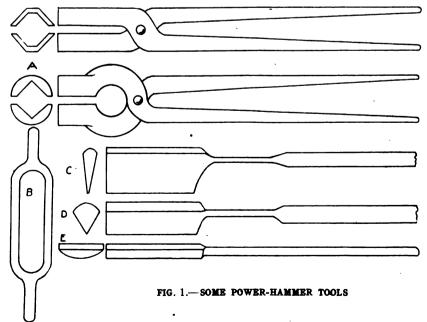
cutting and nicking under the power hammer. When used for this purpose take but a section of the file and use it in connection with have the spring in one piece, as at B. In making the swage at A the lower part is made to fit the bottom dies of the hammer very snugly. The top part
