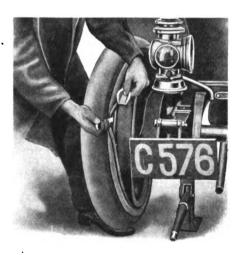
FIG. 6-PUT LUGS IN FROM THE BACK
