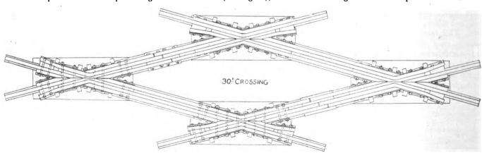
FIGS. 6 AND 7.—THREE-RAIL BOLTED PLATE CROSSING WITH ROLLED STEEL THROAT-BLOCKS
