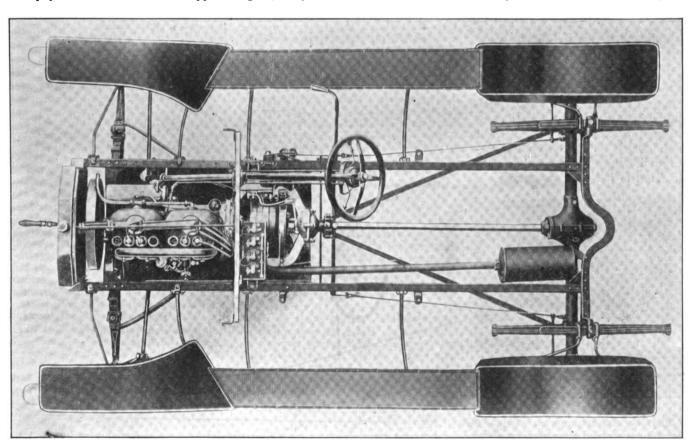
FIG. 3.—A TOP VIEW OF THE FORD CHASSIS USED FOR THE MODEL S ROADSTER
