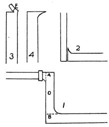
FORGING CRANK AXLES
