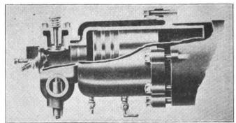
FIG. 3.—SHOWING WATER JACKET OF MOTOR CYLINDER
