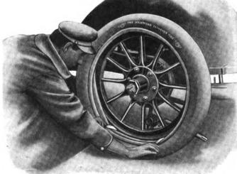
FIG. 2-START TO REPLACE TIRE WITH A CLEAN RIM
