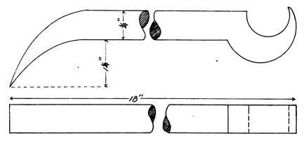
FIG. 3-A HANDY TOOL FOR PULLING KEYS
