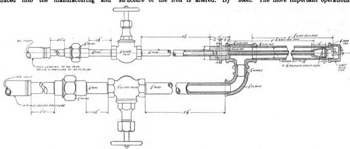
FIG. 5.—DETAIL AND PARTIAL SECTIONAL VIEW OF THE BURNER WITH ALL DIMENSIONS AND INSTRUCTIONS FOR MAKING
