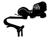
Patented Nov. 25, 1902 Patented June 11, 1907 The spring is pivoted at the front so that it can be turned out of the way of the wrench while clipping Coupling to the axle.
