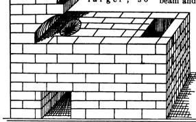
FIG. 1.—THE BASE OF THE CHIMNEY SHOULD EXTEND THE FULL WIDTH OF THE FORGE
