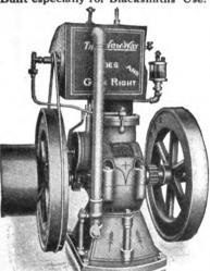
Look at the other engines first. Note the multitude of rods, springs and triggers described as simple. Remember that the water tank (always left out of the cut) has to be filled and emptied every winter day. To forget it once may mean a ruined engine. Remember that water-cooled engines all have packed cylinder heads. Packing leaks and blows out. Inevitable trouble and loss of power sometime.
