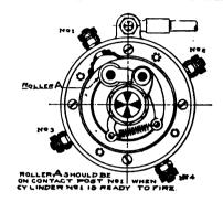
FIG. 1—DIAGRAM SHOWING METHOD OF SETTING COMMUTATOR
