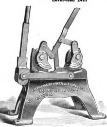
American Tire and Axle Shrinker. Will shrink up to 4 x 1 inches round edge tire, and axles up to 11/4 inches.
