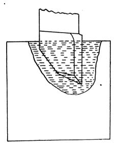
FIG. 6.—DON'T DIP THE TOOL IN THIS MANNER
