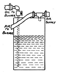
FIG. 6.—METHOD OF PIPING THROUGH OIL TANK
