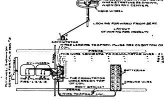
DIAGRAM OF WIRING FOR SPLITDORF COIL
