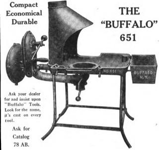
The heavy cast iron fire pan is mounted upon wrought iron legs rigidly braced. This produces a forge of great strength. Equipped with the "Buffalo 200 Silent Blower" placed at right angles to the front of the forge. The hand falls naturally upon the crank. At the same time, it keeps the face away from the fire. A convenience appreciated by the careful smith.
