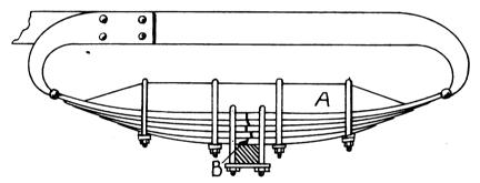
FIG. 2-A TEMPORARY REPAIR UNTIL A NEW SPRING IS PROCURED
