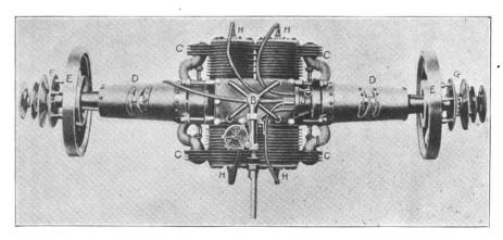
FIG. 3-THE HOLSMAN MOTOR AND PARTS
