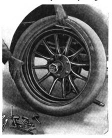
FIG. 3—BEGIN AT VALVE HOLE TO REPLACE TIRE
