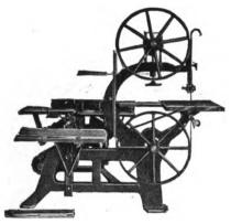
Universal Wood Worker, fitted up with Band Saw,
