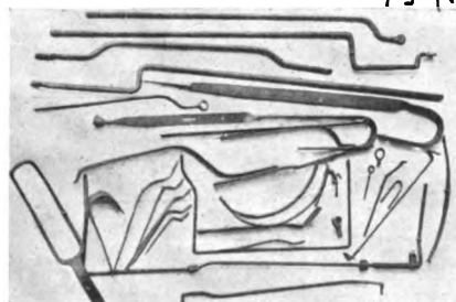
FIG. 2—SOME OF THE BENT SHAPES TURNED OUT BY THIS FORMER
