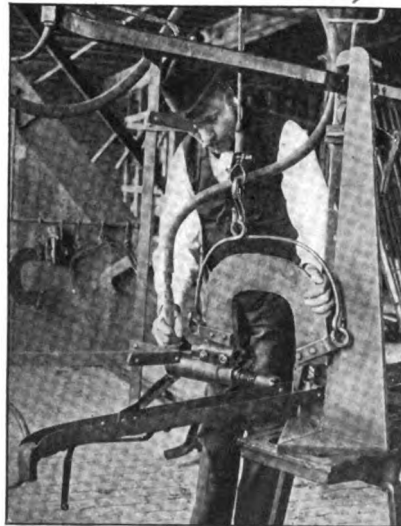
FIG. 7.—SHOWING A YOKE HAMMER IN OPERATION
