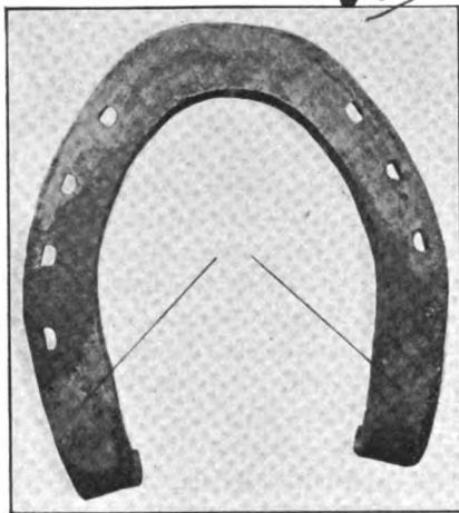
FIG. 1.--THE SHOE HAS A GROOVE WORN IN BOTH BRANCHES
