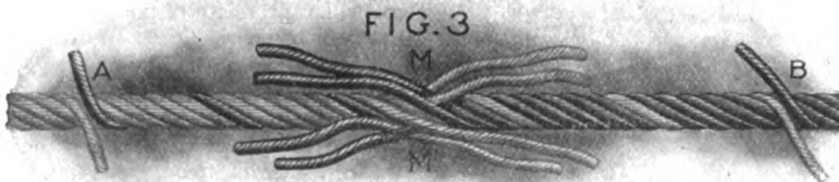
ONE STRAND AT A TIME IS UNLAI D AND REPLACED BY ONE FROM THE OPPOSITE END
