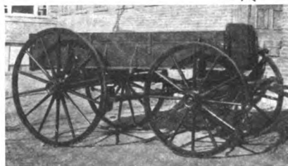
FIG. 6—A TWO-HORSE FARM WAGON BUILT FROM THE ROUGH TIMBER AND IRON
