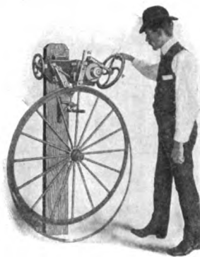
Fig. 2. DRAWING UP THE TIRE.
