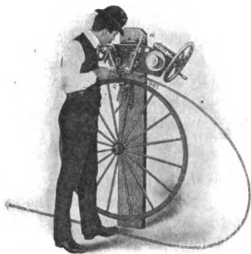
Fig. 1. A RUBBER TIRE SETTER. WHEEL IN PERPENDICULAR POSITION.
