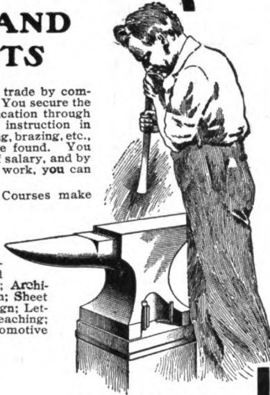
UPSETTING BY RAMMING. (From Shop Practice, copyrighted.)
