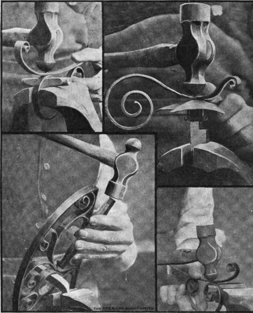
Fig. 22. TWO FORMS OF RIVET BLOCKS IN USE.
