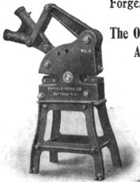
Buffalo Punch, Shear and Bar Cutter
