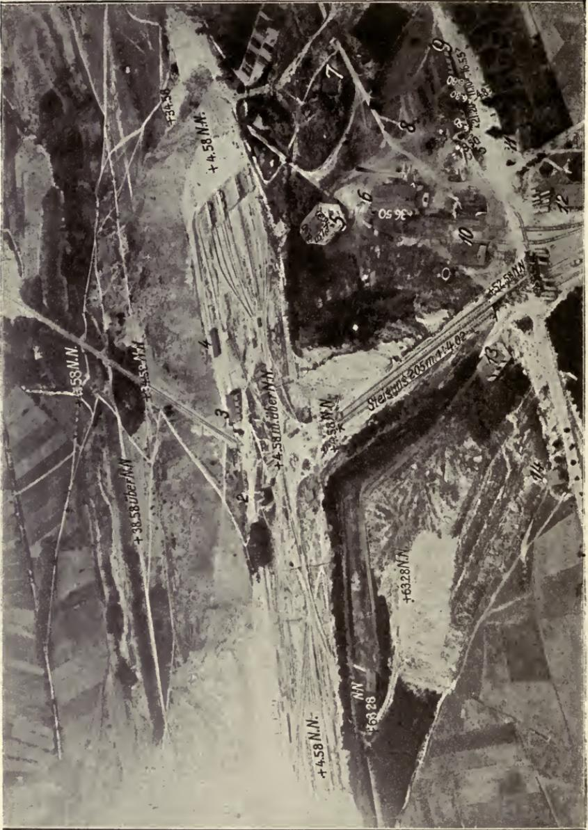
FIG. 207.—Chalkpits near Rüdersdorf. The figures denote the heights above the datum level. (über N.N. = above the datum level. Steigung 205 m, 1 : 4.02 = ascent of 1 in 4.02 over a distance of 670 ft.)
