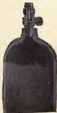
FIG. 107.—Section through steel cylinder.
