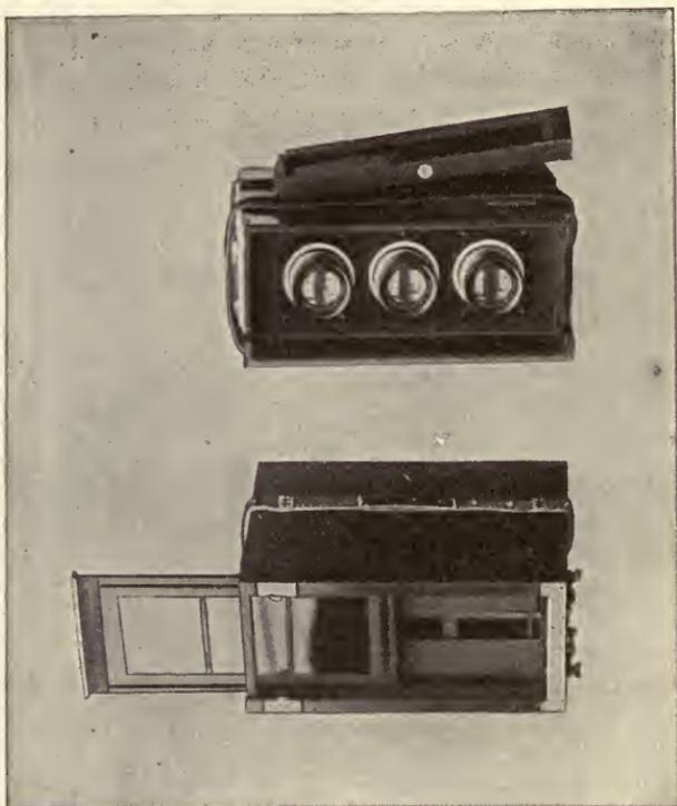
FIG. 213.—Miethe's camera for three-colour photography in a balloon.
