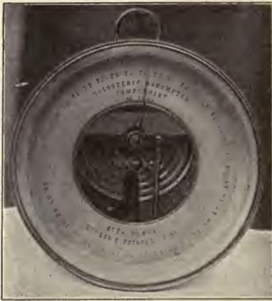
Fig. 118.—Aneroid barometer.
