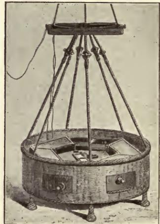
FIG. 216.—Panoramic apparatus for a balloon without observers.
