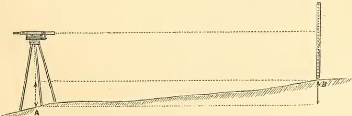
points, as A, in Fig. 346. Measure the height of the level line above the point. Then direct this line to a rod held on the other
