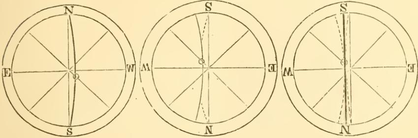
as is shown by Fig. 138, in which the former position of the needle is indicated by a dotted line.\* Now bend the needle, as in Fig. 139, till it cuts divisions midway between those cut by it in its present and in its former position. This makes it certain that the needle is straight, or that its two ends and its center lie in the same straight line.
