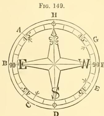
181. We can now understand why W. is on the right hand of the compass-box and E. on the left. Let the direction from the center of the compass to the point B in the figure be required, and suppose the sights in the first place to be pointing in the direction of the needle, S. N., and the north sight to be ahead.
