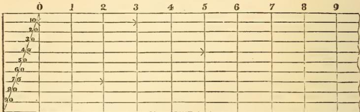
In the fifth figure, the scale of 5 chains to 1 inch is subdivided diagonally to only every quarter-chain, or 25 links. The distance
