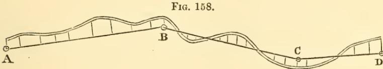
line running in the general average direction of the brook, such as A B in the figure. Measure this line, taking offsets to the various bends of the brook, as explained in Art. 97. Then set the compass at B, and take a back-sight to A, and, if they agree, take a fore-sight to C, and proceed as before, noting particularly the points where the line crosses the brook.
