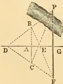
116. *Second Method.* At any convenient point, as A of the given line, erect a perpendicular of any convenient length, as AB, and mark a point C on the given line in the line of P and B. Measure CA, CB, and CP. Then the distance from C to the foot of the perpendicular, i. e.,  $CD = \frac{CA \times CP}{CB}$ .
