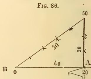
The above numbers are the most easily remembered, but the longer the lines measured the better; and nearly the whole chain may be used; thus: Fix down the 36th link from one end at  $A$ , and the 4th link from the same end on the line at  $B$ . Fix the other end of the chain also at  $B$ . Take the 40th-link mark from this last end, and draw the chain tight, and this mark will be in the perpendicular desired. The sides of the triangle formed by the chain will be 24, 32, and 40.
