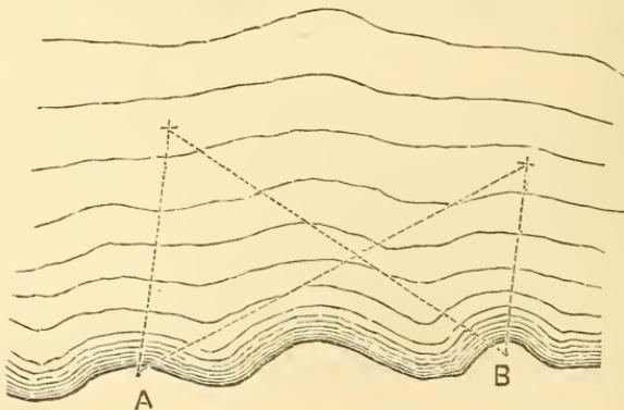
A B, and the angles which the lines of sight make with it would then be known, and its place would be fixed by angular co-ordinates. Two observers are necessary.
