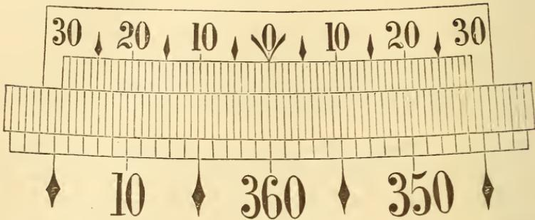
the left-hand vernier is to be read, as in Art. 312; but when the degrees are counted to the right, from the 360° line, the right-hand vernier is to be used.
