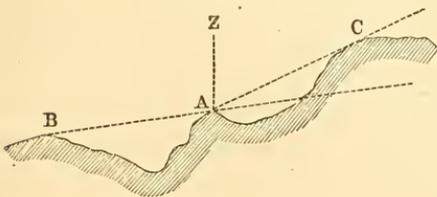
\* To determine at a station A, whether its signal can be seen from B, projected against the sky or not, measure the vertical angles BAZ and ZAC. If their sum equals or exceeds  $180^\circ$ , A will be thus seen from B. If not, the signal at A must be raised till this sum equals  $180^\circ$ .
