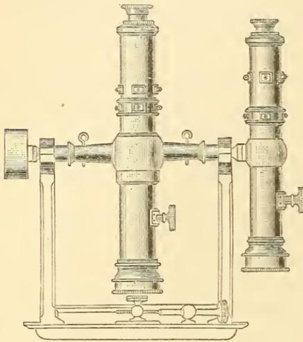
be easily read by lamp-light, and that the marking should be very distinct, on account of the imperfect light available. Again, the instrument should not be too heavy, as there is often difficult climbing to be done over fallen rock and other mine *débris*. If the instrument be easily detached from its tripod, it will often be found a convenience, as thereby the load may be lightened and the instrument itself more carefully carried and more fully protected.
