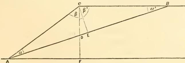
line. Mark two points equally distant from the eye. Measure, by the preceding method, the angles  $\beta$  and  $\beta'$ , which CA and CB make with the vertical CD. Then will half the difference of these angles equal the angle which the slope makes with the horizon.
