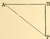
With the transit, set it at any point of the given line, as A, and observe the angle between this line and a line thence to the given point, P. Then set at P, sight to the
