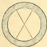
Usually, one cross-hair is horizontal, and the other vertical, as in Fig. 203, but sometimes they are arranged as in Fig. 205, which is thought to enable the object to be bisected with more precision. A horizontal hair is sometimes added.
