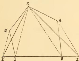
When the figure has many angles, they should not be numbered consecutively all the way around, but, after the numbers have gone around as far as the angle where it is intended to have the vertex of the final triangle, the numbers should be continued from the other angle of the base, as is shown in Fig. 50. In it only the intersections are marked.
