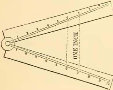
ends L in English instruments, and consists of two lines running from the center to the ends of the scale, and each divided into ten equal parts, each of which is again subdivided into ten, so that each leg of the scale contains 100 equal parts. To illustrate its use, suppose that a scale of 7 chains to 1 inch is required.
