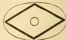
the cross-hair may be above or below the middle of the target by its full thickness, as magnified by the eye-piece of the telescope without the error being perceptible. The next three, Figs. 380,
