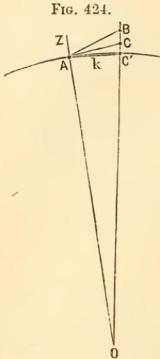
A correction for the curvature of the earth must therefore be made. It may be done in two ways: either by calculating  $CC'$ , and adding it to  $BC$ , obtained by formula [1], or by calculating the angle  $CA C'$ , adding it to  $BAC$ , and then applying the formula [1] to the angle  $BAC'$ .
