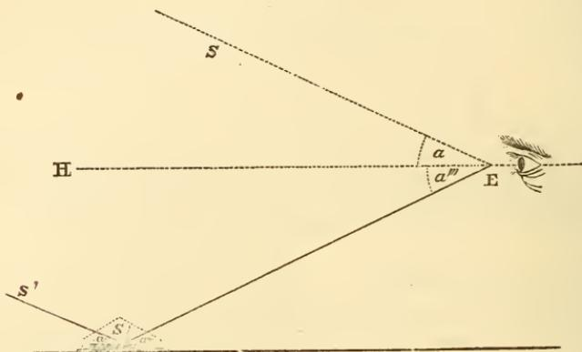
which strike respectively the index-glass and the artificial horizon, are parallel; i. e.; S and S', Fig. 527, are the same point.
