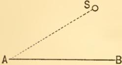
Thus, in Fig. 3, if we know the angle BAS to be a third of a right angle, and AS to be one inch, the point S is determined;
