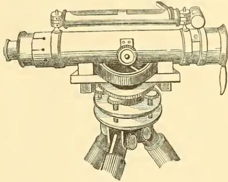
**527. Lenoir's Level.** In this, the telescope carries, at each end, a steel block, whose upper and lower faces are made perfectly parallel. They are placed on a brass circle, which is made level by reversing a level placed upon the upper surface of the steel blocks.
