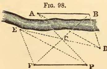
**125. Second Method.** Set a stake at any point C in the line of A P, and another at any convenient place, as at D. Through P set out a parallel to A D, intersecting C D in E. Through E set out a parallel to D B, intersecting C B in F. The line P F will be the parallel required.
