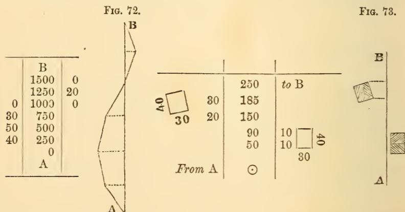
The plat and field-notes of the position of two houses, determined by offsets, are given above on a scale of two chains to one inch :
