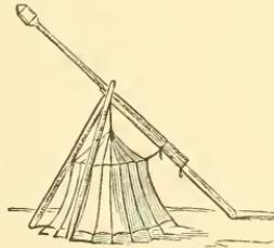
with stones ; and Fig. 507 shows it with the staff turned aside, to make room for the theodolite and its protecting tent. The heights of these signals varied between fifteen and eighty feet.
