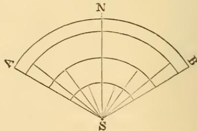
touches the arc at another point, B. Bisect the arc AB at N. Draw SN, and it will be the true meridian, or north and south line required.
