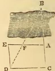
of A E and D B. Measure A F and E F. Then is  $AB = \frac{AC \times AF}{EF}$ ; or  $CB = \frac{AC \times CD}{EF}$ .
