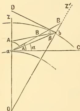
Signals are erected at each point, and from *a* the angle  $B a C = A$  is observed; and from *b* the angle  $A b D = B$ . The heights of the signals above the instrument at *a* and *b* are *h* and *h'*. The distance between the signals is *k*.
