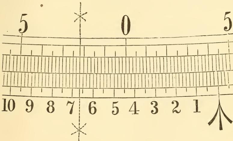
reading must be made as explained in the last article. Thus, in the figure, the reading on the arc from the zero of the limb to the zero of the vernier is  $4^{\circ} 20'$ , and something more, and the reading of the vernier from 10 toward the right, where the lines coincide, is  $3' 20''$  (or it is  $10' - 6' 40'' = 3' 20''$ ), and the entire reading is therefore  $4^{\circ} 23' 20''$ .
