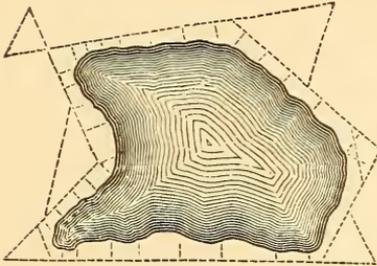
such as a pond, swamp, forest, block of houses, etc., as appears from the figure, in which external bounding lines are taken at will and measured, and tied by "tie-lines" measured between these lines, prolonged when necessary, while offsets
