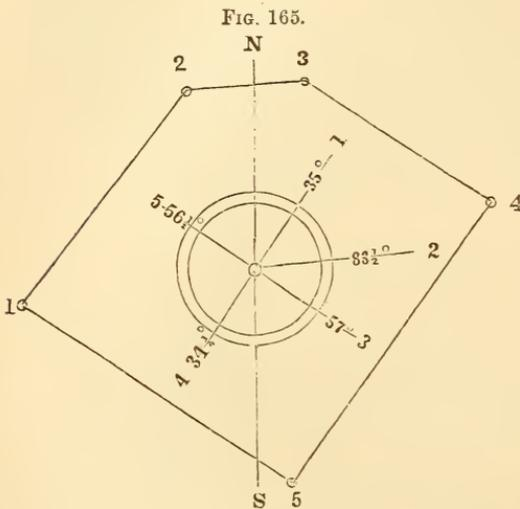
it must be attached to a square board so that the N and S line of the compass-box may be parallel to two opposite edges of the board. This is placed on the paper, and the box is turned till the needle points as it did when the first bearing was taken. Then a line drawn by one edge of the board will be in a
