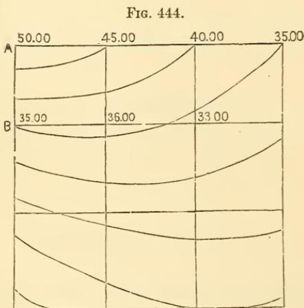
**627. Interpolating with the Sector.** This is one of the easiest ways. The problem is: having given on a plat two points of known height, to interpolate between them a point of any desired intermediate height.
