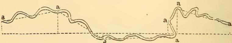
When offsets from lines measured around a field are taken inside of these bounding lines, they are sometimes distinguished as *insets*.
