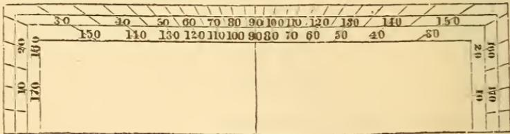
semicircular one is preferable. The objection to the rectangular protractor is that the division corresponding to a degree is very unequal on different parts of the scale, being usually two or three times as great at its ends as at its middle.
