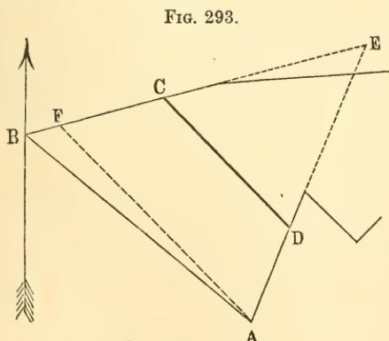
On the ground or plat produce the two converging sides to meet at some point  $E$ . Calculate the content of the triangle  $ABE$ . Measure the side  $AE$ . From  $ABE$  subtract the area to be cut off, and the remainder will be the content of
