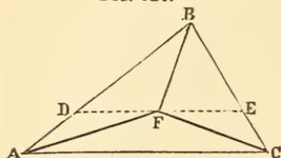
be found. On any side, as  $AB$ , take  $AD = \frac{1}{3} AB$ . From  $D$  draw  $DE$  parallel to  $AC$ . The middle,  $F$ , of  $DE$ , is the point required.
