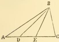
Suppose that a triangular field,  $ABC$ , had to be divided among five men, two of them to have a quarter each, and three of them each a sixth. Divide  $AC$  into two equal parts, one of these again into two equal parts, and the other one into three equal parts. Run the lines from the four points thus obtained to the angle  $B$ .
