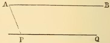
**360.** *To trace a line through a given point parallel to an inaccessible line.* Let  $C$  be the given point and  $AB$  the inaccessible line. Find the angle  $CAB$ , as in Art. 381. Set the instrument at  $C$ , direct it to  $A$ , and then turn it so as to make an angle with  $CA$  equal to the supplement of
