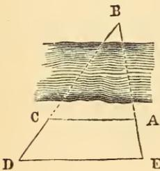
152. **By Parallels.** From A measure AC in any convenient direction. From a point D, in the line of BC, measure a line parallel to CA, to a point E in the line of AB. Measure also AE.
