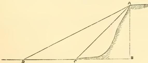
*When the base is inaccessible:* Make  $C = 45^\circ$ , and  $D = 26^\circ 34'$ . Then  $CD = AB$ . So, too, if  $C = 26^\circ 34'$ , and  $D = 18^\circ 26'$ .
