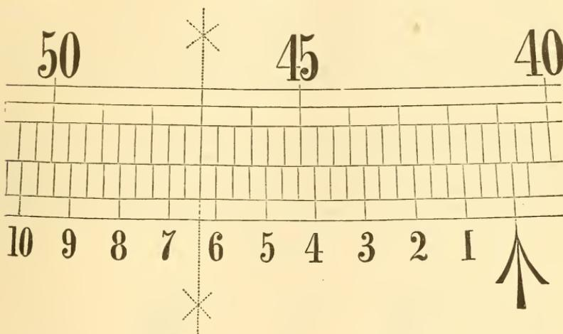
40 spaces on the vernier (numbered to whole minutes) are equal to  $13^\circ 40'$  on the limb—i. e., to 41 spaces, each of  $20'$ .
