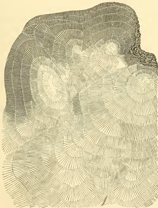
steeper than 45° are represented by short, heavy lines, parallel to the contour-lines, as shown in the upper right-hand corner of Fig. 455—a hill drawn by Lehmann's method.
