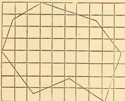
number of squares which fall within the plat represent so many square chains; and the triangles and trapezoids which fall outside of these may then be calculated and added to the entire square chains which have been counted.
