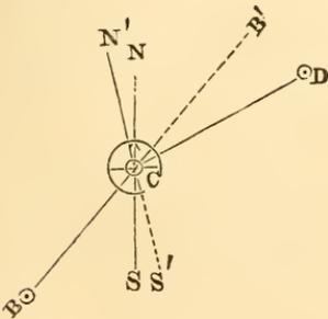
tion must be at C, and the forward bearing must be corrected by the difference just found between the fore- and back-sights, adding or subtracting it, according to circumstances. An easy method is to draw a figure for the case, as in Fig. 153. In it, suppose the true bearing of BC, as given by a fore-sight from B to C, to be N. 40° E., but that there is local attraction
