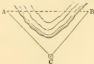
**374. By Triangulation.** Let  $AB$  be the inaccessible distance. From any point,  $C$ , from which both  $A$  and  $B$  are accessible, measure  $CA$ ,  $CB$ , and the angle  $ACB$ . Then in the triangle  $ABC$  two sides and the included angle are known to find the side  $AB$ .\*
