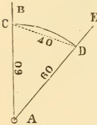
To lay off an angle with this scale, as, for example, to draw a line making at A an angle of  $40^\circ$  with AB, take, in the dividers, the distances from 0 to 60 on the scale of chords; with this for radius and A for center, describe an indefinite arc CD. Take the distance from 0 to 40 on the same scale, and set it off on the arc as a chord from C to some point D. Join AD and prolong it. BAE is the angle required.
