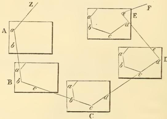
table have one, will facilitate this. Then sight forward from C to D, and fix  $CD$ ,  $cd$  on the plat, as  $bc$  was fixed. Set up at D, make  $dc$  coincide with  $DC$ , and proceed as before. The figure shows the lines drawn at each successive station. The table drawn at A shows how the survey might be commenced there.
