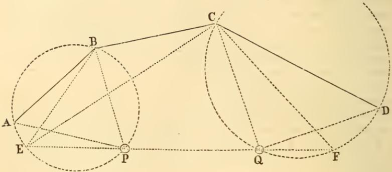
$EB$  and  $BC$ , and the angle  $EBC = ABC - ABE$ ; whence  $EC$  and the angle  $ECB$  are found. In the triangle  $ECF$  are known  $EC$ ,  $FC$ , and the angle  $ECF = BCD - ECB - FCD$ ; whence we find  $EF$ , and the angles  $CEF$  and  $CFE$ .
