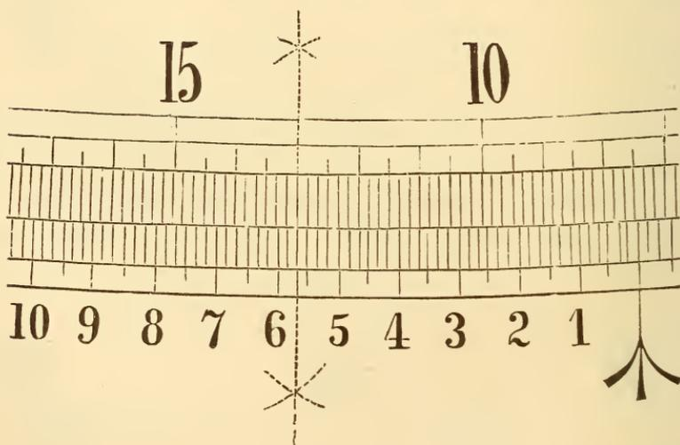
**316. Reading backward.** When an index carrying a vernier is moved backward, or in a contrary direction to that in which the numbers on the circle run, if we wish to read the space which it has passed over in this direction from the zero-point, the vernier must be read backward (i. e., the highest number be called 0), or its actual reading must be subtracted from the value of the smallest space on the circle. The reason is plain ; for, since the vernier
