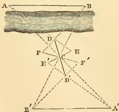
Take any convenient point, as  $C$ . Set stakes at two other points,  $D$  and  $D'$ , in the same line, and at equal distances from  $C$ . Take a point  $E$ , in the line of  $AD$ ; measure from it to  $C$ , and onward till  $CE' = CE$ . Take a point  $F$  in the line of  $BD$ ; measure from it to  $C$ , and onward till  $CF' = CF$ . Range out the lines  $AC$  and  $E'D'$ , and set a stake at their intersection,  $A'$ . Range out the
