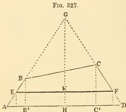
of the triangle  $ADG$ . Then  $GK = GH \sqrt{\left(\frac{ma + na'}{(m+n)a}\right)}$ . Having measured this length of  $GK$  from  $G$  on  $GH$ , set off at  $K$  a perpendicular to  $GK$ , and it will be the required line of division.
