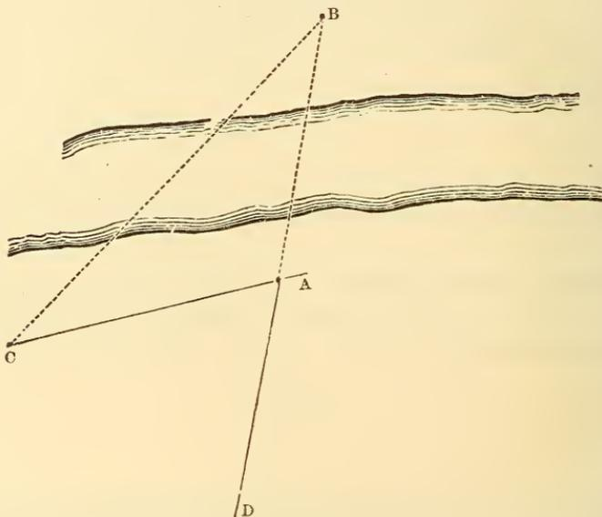
set to half that angle, looking at  $A$  directly, and  $B$  by reflection, till you come to some point,  $C$ , at which they coincide. Then is  $C A = A B$ .
