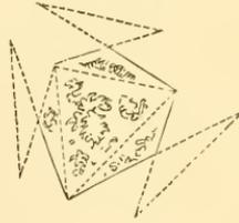
The method of this article may be employed for a figure of six sides, as shown in Fig. 61 (in which the dotted lines within the wooded field have their lengths determined by the triangles formed outside of it), but not for figures of a greater number of sides.
