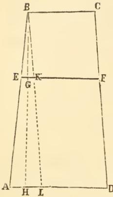
$$EF = \sqrt{\left(\frac{m \times AD^2 + n \times BC^2}{m + n}\right)}.$$
