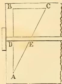
be half the original scale. Divide the outermost arc into three equal parts, and draw a line from A to one of the points of division, as D. Then *each* arc will be divided into parts, one of which is twice the other. Take any distance on the original scale, and find by trial which of the arcs on the right-hand side of the figure it corresponds to. The other part of that arc will be half of it, as desired.
