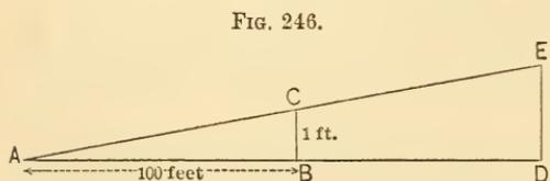
for one revolution of the gradienter-screw, was 4.27 feet, the distance at which the rod was held was 427 feet.
