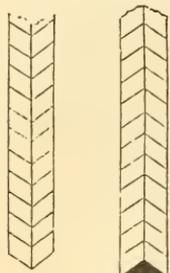
**530. Target.** This is a plate of iron or brass, attached to the rod in such a way that it may be moved up and down the rod and clamped in any position. The face of the target should be painted of such a pattern that, when sighting to it, it may be very precisely bisected by the horizontal cross-hair. Some of the many varieties are given in Figs. 377-385.
