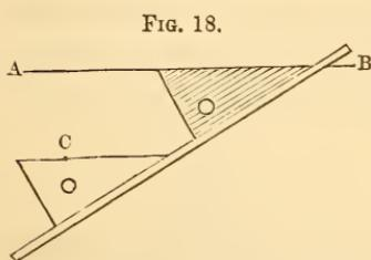
be the line to which a parallel is to be drawn, and C the point through which it must pass. Place one side of the triangle against the line, and place the ruler against another side of the triangle. Hold the ruler firm and immovable, and slide the triangle along it till the side of the triangle which had coincided with the given line passes through the given point. This side will then be parallel to that given line, and a line drawn by it will be the line required.
