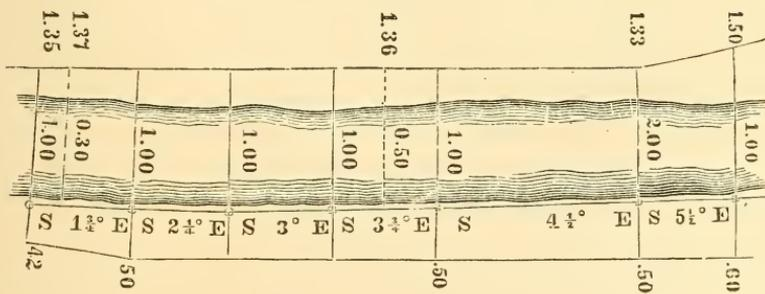
rection of the length of the canal were made. The *bearings* refer to the magnetic meridian at the time of the survey. The *lengths* of the several portions are inserted at the *end* of each in chains and links. The *offsets* at each station are represented by red lines drawn across the canal in such a direction as to bisect the angles
