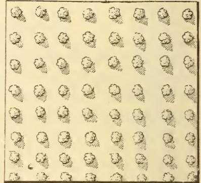
utter violation of the principles of mapping in horizontal projection, though it may be defended as a pure convention. *Orchards* are represented by trees arranged in rows (Fig. 459). *Bushes* may be drawn like trees, but smaller. Fig. 460 represents trees and bushes intermingled.
