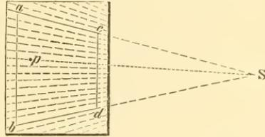
Divide  $ab$  and  $cd$  into the same number of equal parts. The table is then prepared. Now let there be a station,  $P, p$  on the table, at which the table is to be oriented. Set the table, so that  $p$  is over  $P$ , apply the edge of the ruler to  $p$ , and turn it till this edge cuts  $cd$  in the division corresponding to that in which it cuts  $ab$ . Then turn the table till the sights point to  $S$ , and the table will be oriented.
