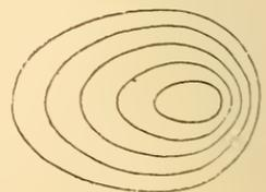
right cone would thus be represented by a series of concentric circles, as in Fig. 439; an oblique cone, by circles not concentric, but nearer to each other on the steep side than on the other, as in Fig. 440; and by a half-egg, somewhat as in Fig. 441.
