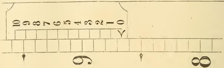
vernier has moved up two hundredths of an inch ; and so for other numbers. If the position of the vernier be as in this figure, the line marked 7 on the vernier corresponding with some line on the scale, the zero-line of the vernier is seven hundredths of an inch above the division of the scale next below this zero-line. If this division be, as in the figure, 8 inches and 6 tenths, the reading will be 8.67 inches.\*
