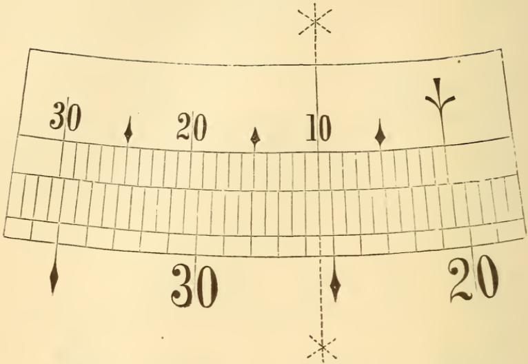
If 15 spaces on the vernier are equal to 16 on the circle, each space on the vernier will be  $= \frac{16 \times 30'}{15} = 32'$ , and the vernier will therefore read to 2'.
