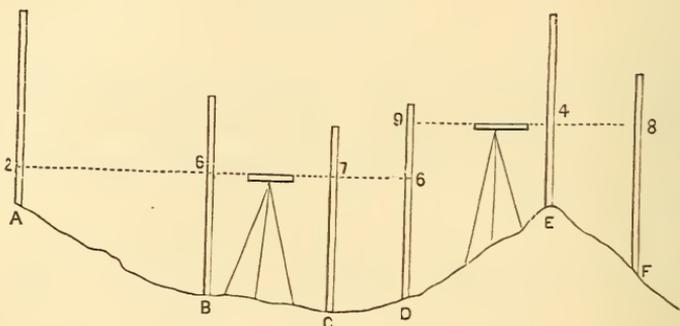
preceding one, but with only two settings of the instrument. D is the turning-point :
