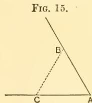
sponding to it gives the angle required. Otherwise, since the chord of any angle equals twice the sine of half the angle, we have this rule: Divide half the tie-line by the measured distance, find in a table of natural sines the angle corresponding to the quotient, and multiply this angle by two, to get the angle desired.
