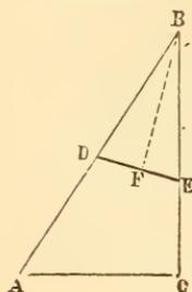
From B set off BD and BE each equal to  $\sqrt{\left( \frac{2 BDE}{\sin. B} \right)}$ . The line DE thus obtained will be perpendicular to the line, BF, which bisects the angle B. The length of DE =  $\frac{\sqrt{(2 \cdot DBE \cdot \sin. B)}}{\cos. \frac{1}{2} B}$ .
