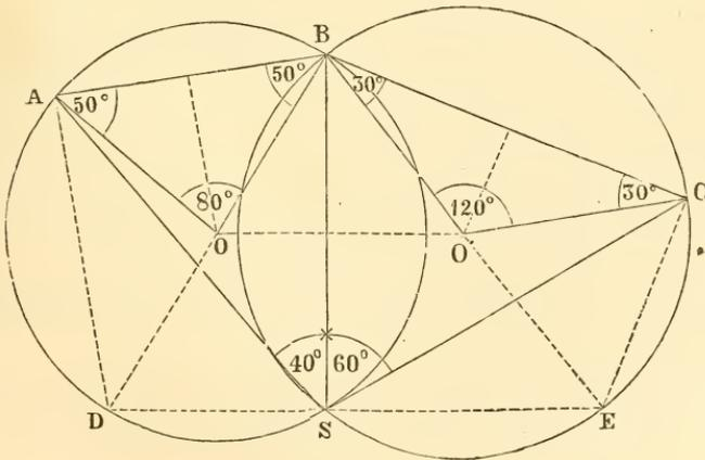
measured. To fix this point, S, on the plat containing A, B, and C, draw lines from A and B, making angles with AB each equal
