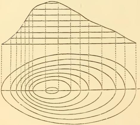
to be drawn as they would be seen from above, or horizontally projected on the map, as in Fig. 438. These are "contour-lines."
