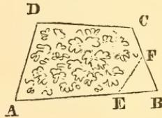
To plat this field, construct the triangle BEF, as in Art. 82. Produce the sides BE and BF, till they become respectively equal to BA and BC, as measured on the ground. Then, with A and C as centers, and with radii respectively equal to AD and CD, describe arcs, whose intersection will be D, the remaining corner of the field.
