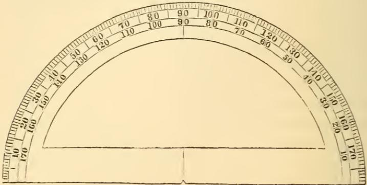
extending beyond its circumference, so that a line can be at once drawn by it when it is set to the desired angle. A Vernier scale is sometimes added to it to increase its precision.
