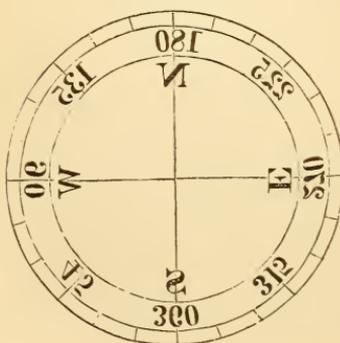
card are reversed or written upside down, as in the figure (in which only every fifteenth degree is marked), because they are again reversed by the prism.
