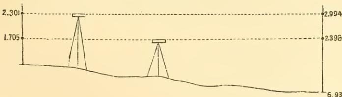
to set near to it, and sight to a rod held on it, and use this reading instead of the measured height of the cross-hairs.
