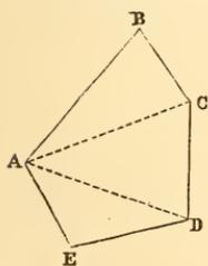
Thus, take any polygon, such as the five-sided one in the figure. Express the angle which the directions of any two sides, as A B, C D, make with each other, thus  $(A B \wedge C D)$ . Then will the content of that polygon be, as below :
