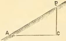
$\frac{BC}{AC}$ ; which is the tangent of the angle  $BAC$ . The English and Americans use the ratio of the base to the height—i. e.,  $\frac{AC}{BC}$ ,
