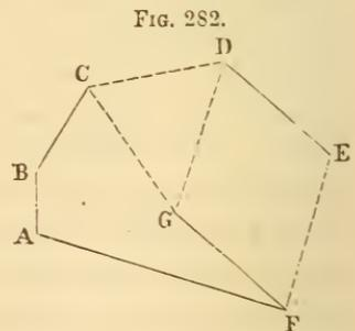
angle in which the three sides are given to determine the angles and thence the required bearings.
