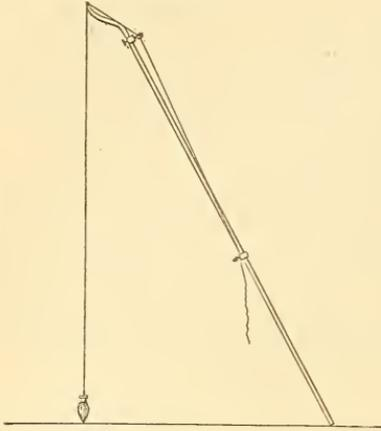
hole, about one eighth of an inch in diameter, in the center of a painted +, or a circle about six inches in diameter. Fig. 559 shows a very convenient device for marking the stations, and plumbing down from them when the roof is high. It is made of light gas-pipe, about half an inch in diameter, and of any convenient length. At one end is a drill; the other end is bent about three inches out of line, and tapered at the end to fit
