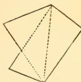
from one corner to the other corners; from a point in one of the sides to the corners; from a point inside of the figure to the corners; and from various corners to other corners. The last method is usually the best. The lines ought to be drawn so as to make the triangles as nearly equilateral as possible.
