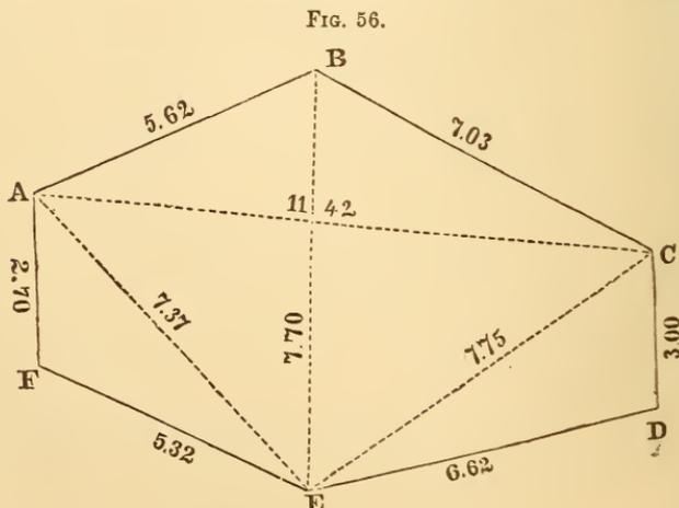
enough to divide the field into triangles, of which there will always be two less than the number of sides. Choose such diagonals as will divide the field into triangles as nearly equilateral as possible. Measure also one or more diagonals for "proof-lines." It is well for the surveyor himself to place stakes in advance at all the corners of the field, as he can then select the best mode of division.
