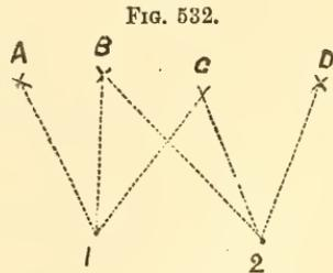
When the shore is inaccessible, a base-line must be measured on the water, and points on the shore fixed by angles from its ends, as in Art. 729.
