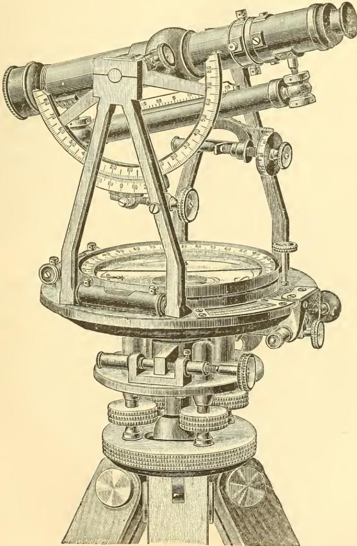
Attached to the right-hand standard is the "Gradienter" (shown in detail in Fig. 245).
