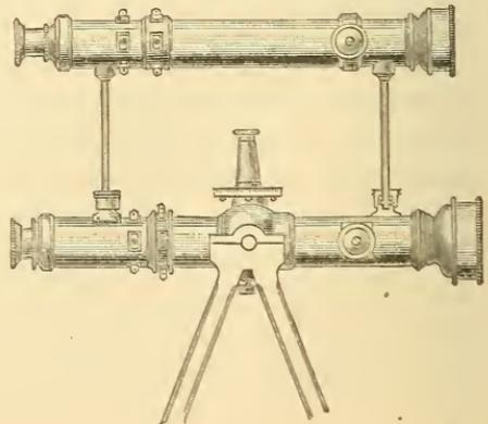
transit an extra telescope is attached on one side, as shown in Fig. 561, and is balanced by a weight on the opposite side. The advantage of this form is, that sights may be taken vertically up or down, as is sometimes necessary in connecting the underground surveys with those on the surface.
