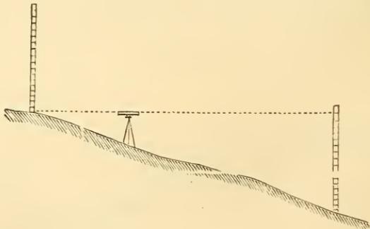
slopes so steep that the rod is too near the level to be read. If this be impossible, keep notes of the lengths of the sights to the turning-points, backward and forward, and as soon as possible take
