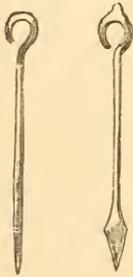
On irregular ground, two stout stakes, about six feet long, are needed to put the forward chain-man in line, and to enable whichever of the two is lowest to raise his end of the chain in a truly vertical line, and to strain the chain straight.
