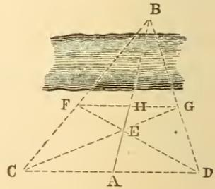
**158. To an Inaccessible Line.** The shortest distance,  $CD$ , from a given point,  $C$ , to an inaccessible straight line  $AB$ , is required. From  $C$  let fall a perpendicular to  $AB$ , by the method of Art. 119. Then set a stake at any point,  $E$ , on the line  $AC$ ; set a second,  $F$ , at the intersection of  $EB$  and  $CD$ ; a third,  $G$ , at the intersection of  $AF$  and  $CB$ ; and a fourth,  $H$ , at the intersection of  $EG$  and  $CD$ .
