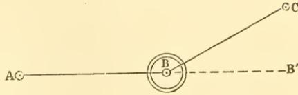
To measure it with the *Transit*, set the instrument at B, direct the telescope to A, and then turn it over. It will now point in the direction of AB produced, or to  $B'$ , if the second adjustment has been performed. Note the reading. Then direct the telescope to C. Note the new reading, and their difference will be the required angle of deflection,  $B'BC$ .
