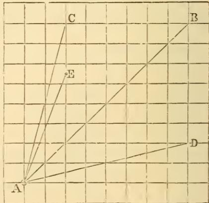
which the line AC is the hypotenuse, is 4 to 1, the line AC makes an angle of  $14^\circ$  with the meridian. The line AD, the hypotenuse of an equal triangle which has its long side lying east and west, makes likewise an angle of  $14^\circ$  with that side, and therefore makes an angle of  $76^\circ$  with the meridian.
