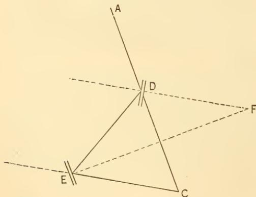
desired angle equal to twice the angle which the mirrors make with each other.
