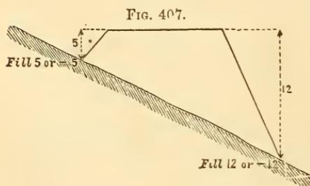
intended outside edges—i. e., where their slopes will meet the surface of the ground ; and the height which the ground at those points is above or below the required height or depth of the top or bottom of the finished work, is marked on
