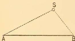
Thus, in Fig. 4, the point  $S$  is determined by being in the intersection of the two lines  $AS$  and  $BS$ , which make respectively angles of a half and of a third of a right angle with the line  $AB$ , which is one inch long ; for the place of the point could be found, if lost, by drawing from  $A$  and  $B$  lines making with  $AB$  the known angles.
