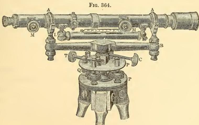
wyes by tapering pins, so that the telescope can be clamped in any position. The milled-headed screws at M and M are used to move
