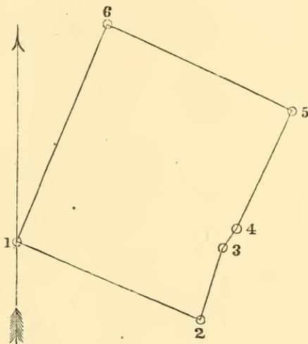
**258. Mascheroni's Theorem.** *The surface of any polygon is equal to half the sum of the products of its sides (omitting any one side) taken two and two, into the sines of the angles which those sides make with each other.*
