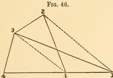
Draw a line from the first to the third angle of the figure. From the second angle draw a parallel to the line just drawn, cutting the produced side in a point 1'. From the point 1' draw a line to the third angle. A triangle (1'—3—4 in the figure) will thus be
