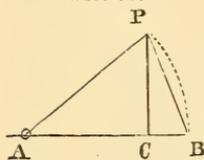
from the given point P, to some point, as A, of the given line. Hold the end of the distance at A, and swing round the other end of the chain from P, so as to set off the same distance along the given line from A to some point B. Measure BP. Then will the distance BC from B to the foot of the desired perpendicular
