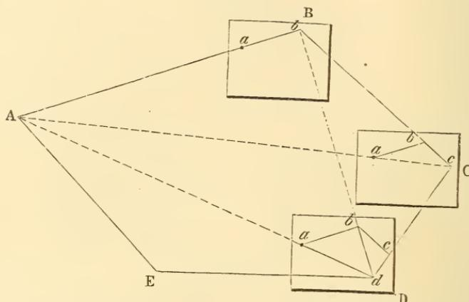
the point in which the edge of the ruler cuts the line drawn from B will be the point *c* on the table. Next sight to D, and draw an indefinite line. Set up at D, and make the line last drawn point to C. Then fix the needle at *a* or *b*, and by the alidade, as at the last station, get a new line back from either of them, to cut the last-drawn line at a point which will be *d*. So proceed as far as desired.
