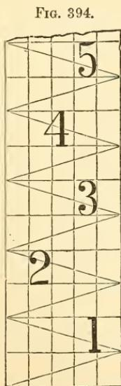
each 0·02 foot high, so that it reads to hundredths, and less by estimation. This is based on the power the eye has in bisecting angles.
