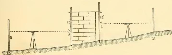
wall, and this B. S. and F. S. had been really taken. Set up the instrument beyond the wall, take a B. S. to this peg, and go on as usual.
