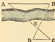
intersection of  $CA$  and  $DB$ , and measure  $CE$ . Then is  $AB = \frac{CD \times (AC - CE)}{CE}$ .
