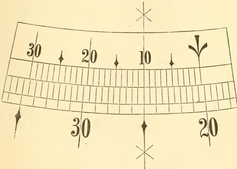
In Fig. 222, the reading is  $20^\circ 40'$ , the index being at a point beyond  $20^\circ 3'$ , and the additional space being shown by the vernier to be  $10'$ .
