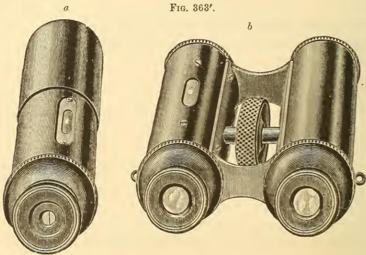
glass, and containing in addition thereto a reflecting prism, cross-wire, and small spirit-level, the last being shown in the open part of the tube.
