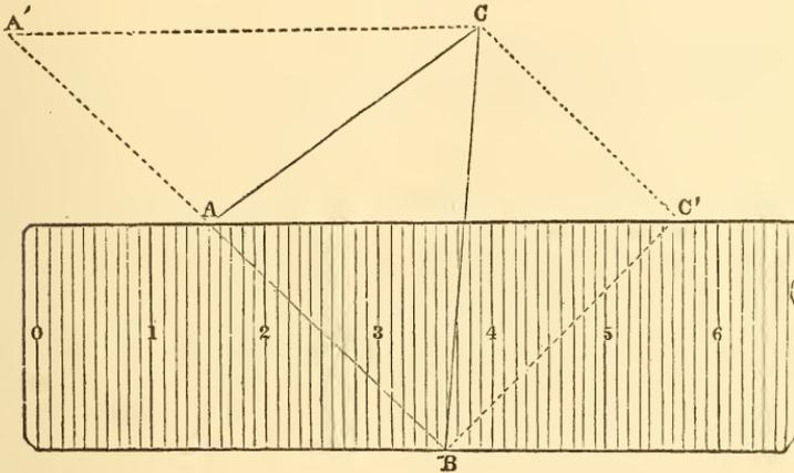
number of divisions on the scale, from the point to which the division A on the scale has arrived, to the third corner of the triangle—express the area of the triangle A B C in square chains.
