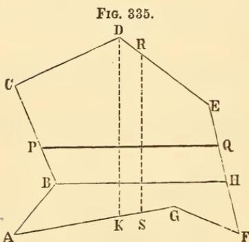
be a given polygon, and B H the direction parallel to which is to be drawn a line P Q, dividing the polygon into two parts in any desired ratio =  $m : n$ . The area P C D E Q =  $\frac{m}{m+n} \cdot A B C D E F G$ .
