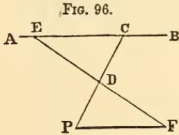
**122. Second Method.** Measure from P to any point, as C of the given line, and put a mark at the middle point D of that line. From any point, as E of the given line, measure a line to the point D, and continue it till  $DF = DE$ . Then will the line PF be parallel to AB.
