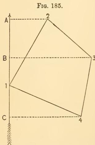
The expressions are simplified by dividing the proposed polygon into two parts by a diagonal, and computing the area of each part separately, making the diagonal the side omitted.
