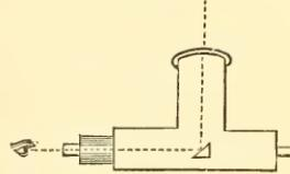
In the telescope is placed a small mirror, or reflector, or (what is still better) a triangular prism of glass, at an angle of  $45^\circ$  to the line of sight. Thus the observer can keep his eye at the same place at any inclination of the telescope.
