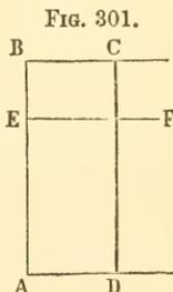
*Demonstration.* Let  $a$  = value per acre of one portion of the land, and  $b$  that of the other portion. Let  $x$  = the width required,  $BC$  or  $AD$ . Then the value of  $BCFE = a \times \frac{x \times BE}{10}$ , and the value of  $ADFE = b \times \frac{x \times AE}{10}$ .
