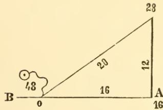
111. *Second Method.* Hold one end of the chain at A and fix the other end at a point B, taken at will. Swing the chain around B as a center, till it again meets the line at C. Then carry the same end around (the other end remaining at B) till it comes in the line of CB at D. AD is the perpendicular required.
