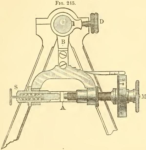
is clamped to the axis by the screw D. M is the micrometer-screw. A is a lip projecting from a plate fastened to the standards.
