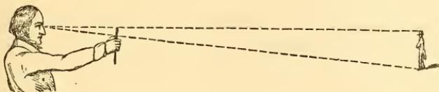
measured with accuracy) of 100, 500, 1,000 feet, etc. To apply this, when a man is seen at any unknown distance, hold up the pencil at arm's length, making the top of it come in the line from the eye to his head, and placing the thumb-nail in the line from the eye to his feet, as in Fig. 16. The pencil having been previously graduated by the method above explained, the portion of it now intercepted between these two lines will indicate the corresponding distance.
