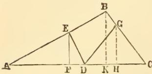
The altitudes, EF and GH, of the parts ADE and DCG, will be obtained by dividing  $\frac{1}{2}$  ABC, by half of the respective bases AD and DC.
