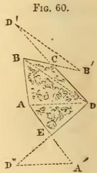
their length, forming two new triangles, as shown by the dotted lines, and measure the sides  $B'D'$  and  $A'D''$ . The three sides of each of these triangles will thus be known, and also the three sides of the triangle  $BAD$ , since  $AD = A'D''$ , and  $BD = B'D'$ .
