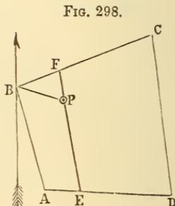
*Example.* A field is bounded thus : N.  $14^\circ$  W., 15.20 ; N.  $70\frac{1}{2}^\circ$  E., 20.43 ; S.  $6^\circ$  E., 22.79 ; N.  $86\frac{1}{2}^\circ$  W., 18.00. A spring within it bears from the second corner S.  $75^\circ$  E., 7.90. It is required to cut off 10 acres from the west side of the field by a straight fence through the spring. How far will it be from the first corner to the point at which the division-fence meets the fourth side ? *Ans.* 4.6357 chains.
