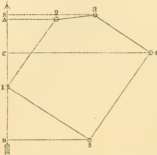
perpendicularly, set off the departure, 155 links.\* This gives the point 2. Join 1...2. From 1 again, set off, upward, 236 links, to B, and from B, to the right, perpendicularly, set off 283 links, which will fix the point 3. Join 2...3; and so proceed, setting off north latitudes along the meridian upward, and south latitudes along it downward; east
