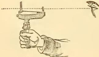
end, through which can be seen a hair which covers, on the circle, the number of the degrees of the angle of inclination, or of the horizontal angle.
