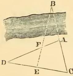
ments of  $DA$  and  $EB$ . Measure  $AC$ ,  $CE$ ,  $ED$ ,  $DF$ , and  $FA$ . Then is  $AB = \frac{AC \times AF \times DE}{CE \times DF - AF \times DE}$ .
