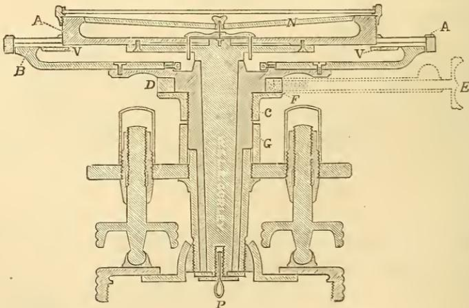
as is usual, are placed near the north and south points of the compass-circle, so that the observer can read the vernier without stepping to the side of the instrument. The slow motion, both of the upper and lower plate, is given by one tangent-screw. In each
