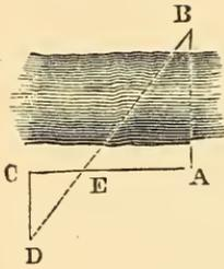
lar, CD. Find a point, E, in the line of AC and BD. Measure AE and EC. Then is  $AB = \frac{AE \times CD}{CE}$ .
