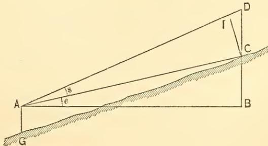
sit; G the point over which it is set; C where the rod is held; A B a horizontal line through the axis of the telescope; A C the distance from the horizontal axis of the telescope to the foot of the rod; and C D the distance, on a vertical rod, passed over by the horizontal cross-hair for one revolution of the gradienter-screw. Let C F be perpendicular to A C, and D B to A B.
