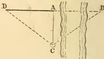
**378. By Triangulation.** Measure a distance  $AC$ , about equal to  $AB$ . Measure the angles at  $A$  and  $C$ . Then, in the triangle  $ABC$ , two angles and the included side are known, to find another side,  $AB = \frac{AC \sin. ACB}{\sin. ABC}$ .
