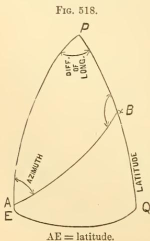
When the triangle sides do not exceed fifteen miles, the geodetic latitudes, longitudes, and azimuths required are computed as follows :
