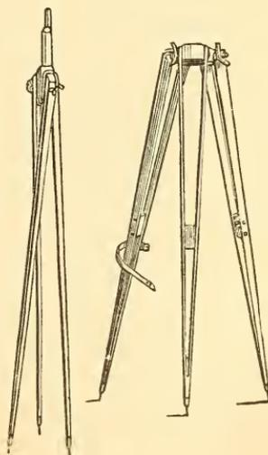
The joints by which the instrument is connected with the tripod are also various. Fig. 144 is the "ball-and-socket joint," most usual in this country. It takes its name from the ball in which terminates the covered spindle which enters a corresponding cavity under the compass-plate and the socket in which this ball turns. It admits of motion in any direction, and can be tightened or loosened by turning the upper half of the hollow piece inclosing
