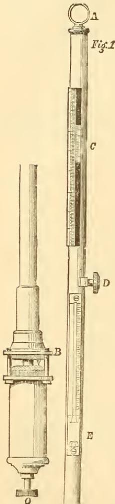
Fig. 436 is a cistern barometer.\* This consists of a column of mercury, contained in a glass tube, whose lower end is placed in a cistern of mercury. The tube is covered with a brass case, terminating at the top in a ring, A, for suspension, and at the bottom in a flange, B, to which the cistern is attached.
