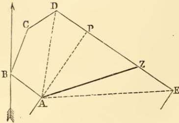
side of it the required line will end, by drawing or running "guess-lines" from the given point to various angles, and roughly measuring the content thus parted off. If, as in the figure, A being the given point, the guess-line AD parts off less than the required content, and
