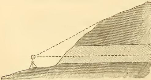
If the line has to be prolonged by setting the instrument farther on, the second adjustment is important.
