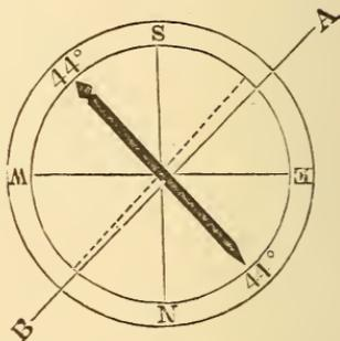
the other end of the sights to be directed to the same object. Suppose that the needle would have pointed to  $45^\circ$  if the line of sight had passed through the center; the needle will now point to  $44^\circ$ , the error being doubled by the reversion, and the true reading being the mean.
