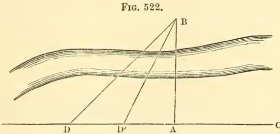
longed, looking by direct vision at  $C$ , until you arrive at some point,  $D$ , from which  $B$  is seen by reflection to coincide with  $C$ . Then is  $A D = A B$ .
