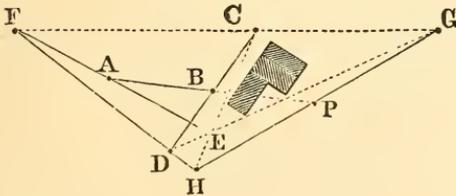
Range out  $FD$  and  $CE$  to intersect in  $H$ . Measure  $GH$ . Its middle point,  $P$ , is the required point in the line of  $AB$  prolonged. The unavoidable acute intersections in this construction are objectionable.
