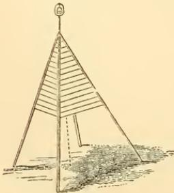
Three or four timbers framed into a pyramid, as in Fig. 504, with a long mast projecting above, fulfill the first and last conditions. The mast may be made vertical by directing two theodolites to it, and adjusting it so that their telescopes follow it up and down, their lines of sight being at right angles to each other. Guy ropes may be used to keep it vertical.
