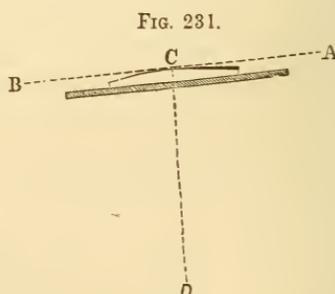
the plate turns. For, let  $AB$  represent this plane, seen edgewise, and  $CD$  the center line of the vertical axis, which is here drawn as making an acute angle with this plane on the right-hand side. The first figure represents the bubble brought to the center of the tube. The second figure represents the plate turned half around. The center line of the axis is supposed to remain unmoved. The
