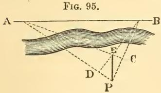
This method will apply when only two points of the line are visible.
