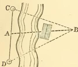
**380. To find the Distance from a Given Point to an Inaccessible Line.** In Fig. 254, Art. 358, the required distance is CE. The operations therein directed give the line CA and the angle CAB, or CAE. The required distance  $CE = CA \cdot \sin. CAE$ .
