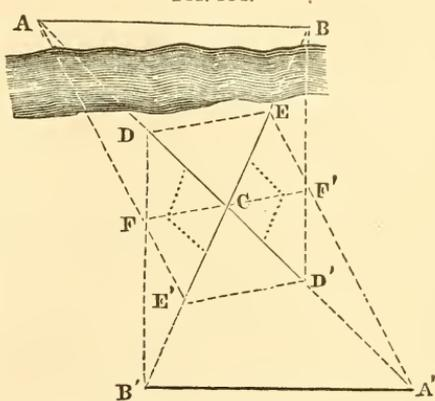
Range out the lines BE' and DF, and set a stake at their intersection B'. Measure A'B', and it will be equal to the desired distance AB.
