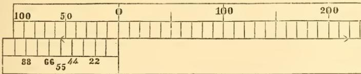
eleven hundredths, or a tenth and a hundredth, and the first division on the short, or vernier scale, will overlap, or be longer than the first division on the long scale, by just *one* hundredth of an inch; the second division will overlap *two* hundredths, and so on. The principle will be more fully developed in treating of "Verniers."
