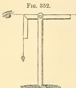
**501. Reflecting Levels.** In these, the perpendicular to the direction of gravity is not an actual line, but an imaginary reflected line.
