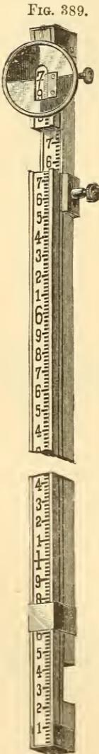
**533. The Boston Rod (Fig. 388).** This is usually in two parts, like the New York rod. The target is rectangular, and is fastened to one of the pieces near its extremity. For heights less than six feet, the rod is held with the target-end down, and the target is moved up by sliding up the piece which carries it. For heights above six feet, the rod is turned end for end, bringing the target-end up, and then sliding up the piece which carries the target.
