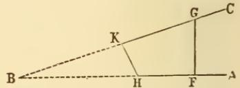
**412. To part off any Figure.** If the field be very irregularly shaped, find by trial any line which will part off a little less than the required area. This trial-line will represent  $HK$  in the preceding figure, and the problem is reduced to parting off, according to the required condition, a *quadrilateral*, comprised between the trial-line, two sides of the field, and the required line, and containing the difference between the required content and that parted off by the trial-line.
