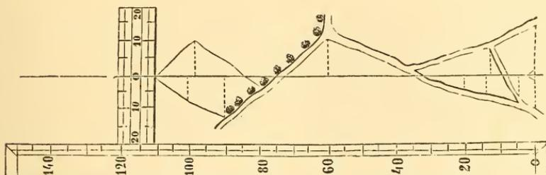
will be greatly facilitated. The points thus obtained are joined by straight lines, and a miniature copy of the curved line is thus obtained; all the operations of the platting being merely repetitions of the measurements made on the ground.
