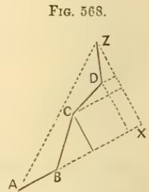
$\tan. Z A X = \frac{X Z}{A X}$ , and the length of A Z =  $\sqrt{A X^2 + X Z^2}$ ; or  $A X \div \cos. X A Z$ .
