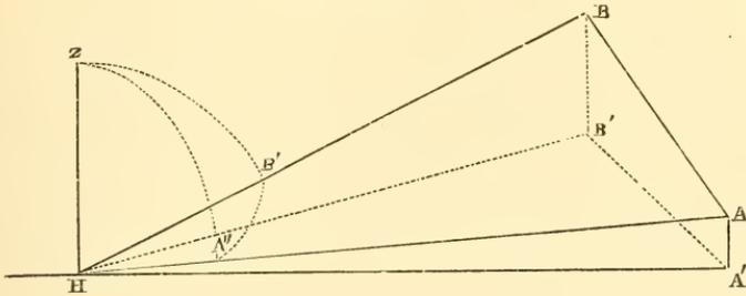
planes,  $AHA'$  and  $BHB'$ , and the oblique plane  $AHB$ , cut this sphere in arcs of great circles,  $ZA''$ ,  $ZB''$ , and  $A'B''$ , thus forming a spherical triangle,  $A'ZB''$ , in which  $A'B'' = h$  measures the observed angle ;  $ZA'' = Z$  measures the zenith-distance of the point  $A$  ; and  $ZB'' = Z'$  measures the zenith-distance of the point  $B$ .
