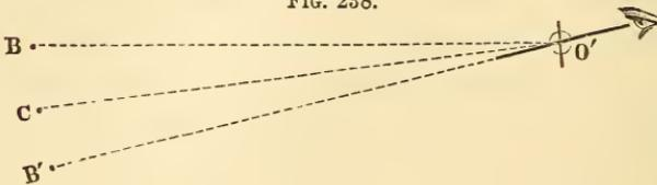
If not, the apparent error is double the real error, as appears from the figures, the obtuse angle  $O$  coming to  $O'$ , and the desired perpendicular line falling at  $C$  midway between  $B$  and  $B'$ . The rectification may be made as before; or, in some large instruments, in which the telescope is supported on  $Y$ s, by moving one of the  $Y$ s laterally.
