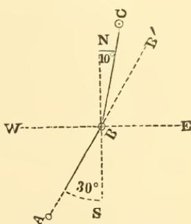
tract the sum of the bearings from  $180^{\circ}$ . *Ex.:* If AB bears N.  $30^{\circ}$  E. and BC bears S.  $40^{\circ}$  E., the angle CBB' is  $110^{\circ}$ .
