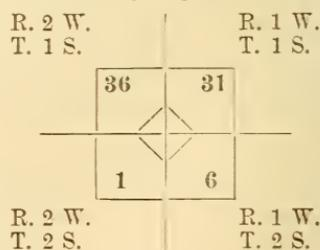
“These marks are to be distinctly and neatly chiseled into the wood, at least the eighth of an inch deep; and to be also marked with *red chalk*. The *number* of the *sections* which they respectively *face* will also be marked on the township post.
