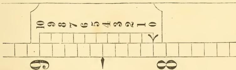
made by setting off on it nine tenths of an inch, and dividing that length into ten equal parts. Each space on the vernier is therefore equal to a tenth of nine tenths of an inch, or to nine hundredths of an inch, and is consequently one hundredth of an inch shorter than one of the divisions of the original scale. The first space of the vernier will therefore fall short of, or be overlapped by, the first
