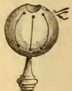
two pairs of plain "Sights," each shaped as in the figure, placed at the ends of two bars at right angles to each other. The slit, and the opening with a hair stretched from its top to its bottom, are respectively at the top of one sight and at the bottom of the opposite sight.\* This is used in the same manner as the preceding form, but is less portable, and more liable to get out of order.
