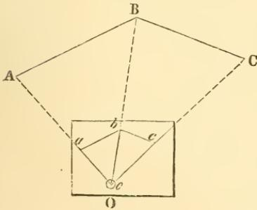
station,  $A$  on the ground. Draw a line by the ruler. The desired point is somewhere in this line. Make the ruler pass through another point,  $b$  on the table, and make the sights point to  $B$  on the ground. Draw a second line, and its intersection with the first will be the point desired. Using  $C$  in the same way would give a third line to prove the work. This operation may be used as a
