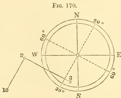
course required, its proper length being set off on it from 1 to 2. Now, suppose the bearing from 2 to be  $S. 60^{\circ} E.$  Draw through 2 a line parallel to the line passing through the center of the circle and through the opposite points  $S. 60^{\circ} E.$  and  $N. 60^{\circ} W.,$  and it will be the line desired. On it set off the proper length from 2 to 3, and so proceed.
