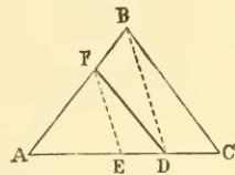
The point  $F$  will be most easily obtained on the ground by the proportion  $AD : AB :: AE = \frac{1}{2} AC : AF$ .
