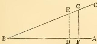
When the field is given on the ground, or on a plat, at any point, as  $D$ , of the given side  $A B$ , set out a "guess-line,"  $D E$ , perpendicular to  $A B$ , and calculate the content of  $D E B$ . Then the required distance
