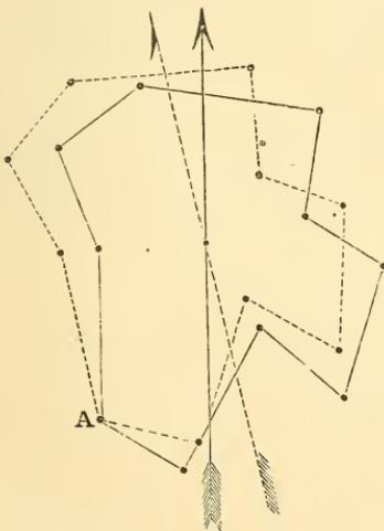
**282. To run out Old Lines.** To succeed in retracing old lines, proper allowance must be made for the change in the variation
