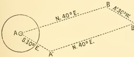
*Second Method.* Set, by repeated trials, two transits on opposite sides of the shaft, so that they shall at the same time point to one
