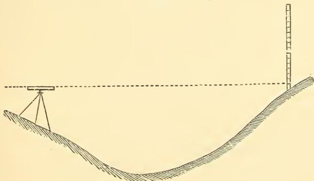
**552.** When the rod is a little too low, raise it alongside of a stake, or the body, and put the top of the rod "right"; then measure down from the bottom of the rod, and add it to its length.
