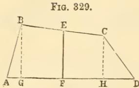
Taking away the triangle  $ABG$ , the remainder,  $GBEF$ , will be to the rest of the figure in a known ratio, and the position of  $EF$ , parallel to  $BG$ , will be found as in the last article.
