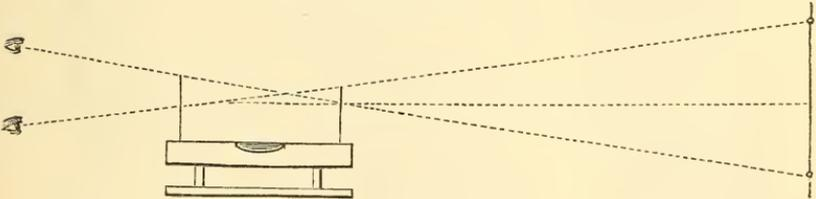
Bring the bubble to the center of the tube and make a mark, in the line of sight, as far off as can be seen. Then turn the level end for end, and sight again. If the bubble remains in the same place, "all right." If not, rectify it by altering the sights, or by altering the marks for the bubble to come to, bringing the bubble half-way back, and trying it again.
