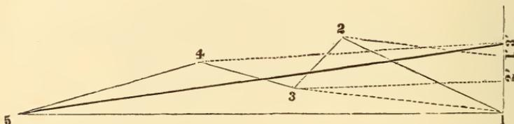
the method given in Art. 76, by which the irregular figure 1...2...3...4...5 is reduced to the equivalent triangle 1...5...3', and the straight line 5...3' therefore parts off the same quantity of land on either side as did the crooked one. The distance from 1 to 3', as found on the plat, can then be set out on the ground and the straight fence be then ranged from 3' to 5.
