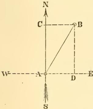
given line, of which the length AB, and the bearing (or angle, B A C, which it makes with the magnetic meridian), are known. It is required to find the differences of latitude and of longitude between its two extremities A and B—that is, to find A C and C B; or, what is the same thing, B D and D A.
