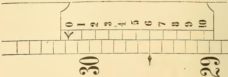
parts, each of which is therefore one tenth of eleven tenths of an inch—i. e., eleven hundredths of an inch, or a tenth and a hundredth. Each space of the vernier therefore overlaps a space on the scale by one hundredth of an inch. The manner of reading this vernier is the same as in the last one, except that the numbers run in a reverse direction. The reading of the figure is 30·16.
