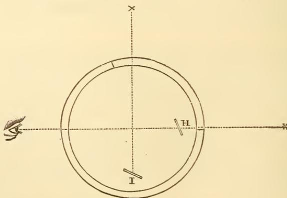
**707. The Optical Square (Fig. 521).** This is a box containing two mirrors, fixed at an angle of  $45^\circ$  to each other, and therefore
