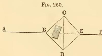
may be done when no means of measuring any distance can be obtained. Let  $AB$  be the line to be prolonged. Set the instrument at  $B$  and deflect angles of  $45^\circ$  in the directions  $C$  and  $D$ . Set at some point,  $C$ , on one of these lines and
