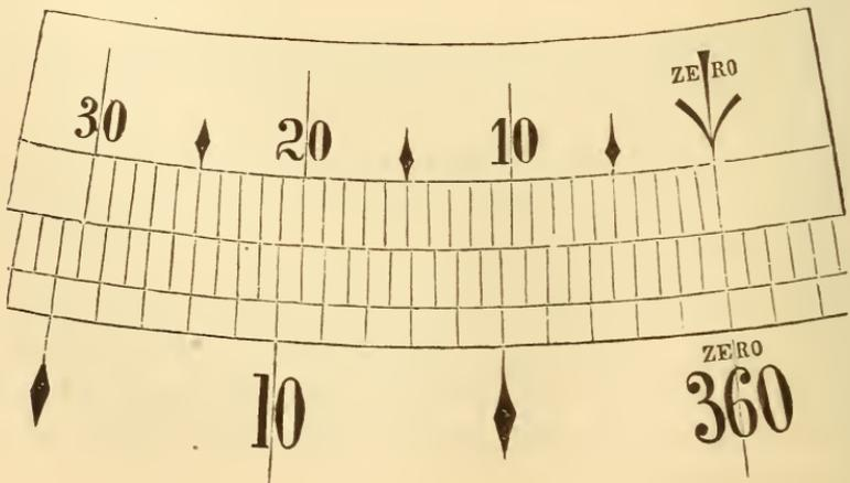
Suppose 30 spaces on the vernier to be equal to 29 on the circle. Each space on the vernier will be  $= \frac{29 \times 30'}{30} = 29'$ , and will therefore be less than a space of the circle by  $1'$ , to which the vernier will then read.
