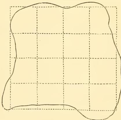
**624. On a Single Hill.** Proceed thus: From its top, range lines down the hill, in various directions, and take their bearings. Set stakes on them at each change of slope, and note the heights and distances of these stakes from the starting-point, and plat their places. The contour-lines are then put in as in Art. 626.
