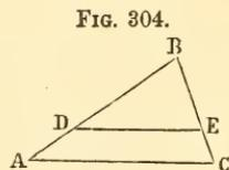
Generally, to divide the triangle into two parts, B D E and A C E D, which shall have to each other a ratio  $= m : n$ , we have  $B D = A B \sqrt{\frac{m}{m+n}}$ .
