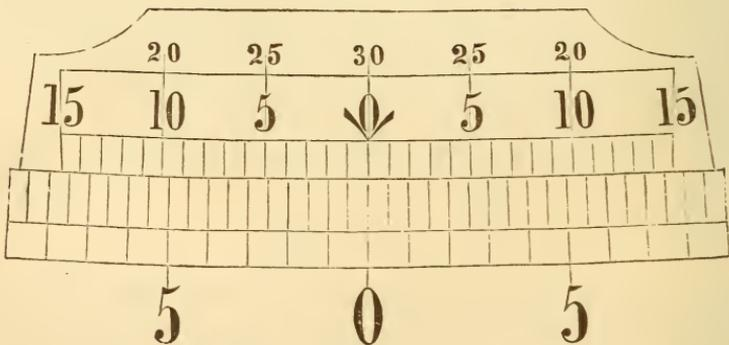
divided to half-degrees, and the vernier reads to minutes, 30 parts on it being equal to 31 on the limb. But the vernier is only half as long as in the previous case, going only to 15', the upper figures on one half being a sort of continuation of the lower figures on the other half. Thus, in moving the index to the right, read the *lower* figures on the left-hand vernier (it being retrograde)
