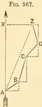
When the compass is used, calculate the latitude and departure of each of the courses, A B, B C, etc. The algebraic sum of their latitudes will be equal to A X, and the algebraic sum of their departures will be equal to X Z. Then is  $\tan. Z A X = \frac{X Z}{A X}$ ; that
