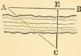
angle  $CAB$  by the method of Art. 381. Set the instrument at  $C$ , sight to  $A$ , and turn an angle  $= 90 - CAB$ . It will then point in the direction of the required perpendicular,  $CE$ .
