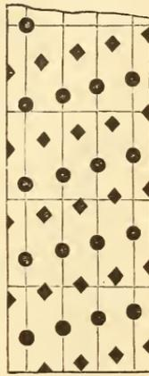
*Pemberton's Rod* (Fig. 396). This is on the principle of nine verniers placed side by side. It reads to hundredths, which are given by counting up from the dot which the hair bisects, to the dot in the same vertical line which is bisected by one of the horizontal lines which mark the tenths. The inventor claims that it can be read nine times as far as Gravatt's.
