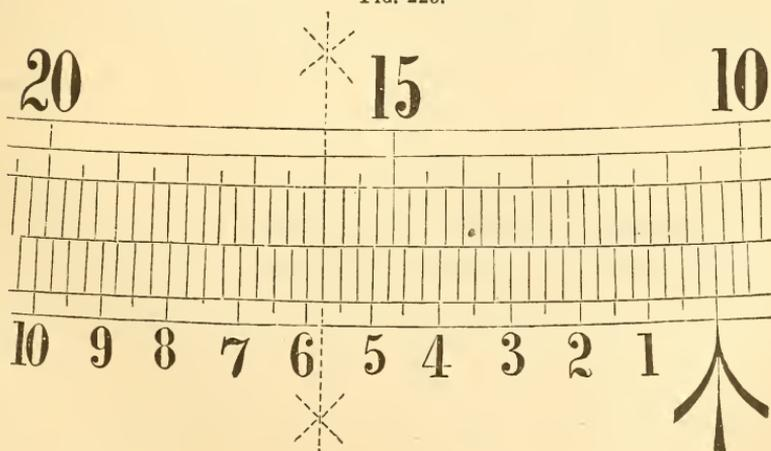
therefore read to  $20' - 19' 40'' = 20''$ . Fig. 224 shows such an arrangement. The reading in that position would be  $40^\circ 46' 20''$ .
