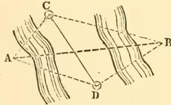
**382. Problem.** To measure an inaccessible distance, AB, when a point, C, in its line can be obtained. Set the instrument at a point, D, from which A, B, and C can be seen, and measure the angles CDA and ADB. Measure also the
