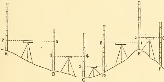
is placed in the column of "Rise"; when it is less, their difference is a "Fall." The following table represents the same observations as the last figure, and their careful comparison will explain any obscurities in either :
