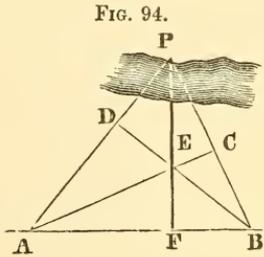
**Problem 7.** To let fall a perpendicular from a given point to an inaccessible line.
