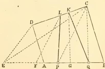
to it. Join C P, and from F draw F L parallel to it. Join P L and Q K, and they will be the division-lines required.
