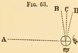
Then turn its head a quarter of the way around, so that the second slit, looked through, points to A. Then see if the other slit covers B again, as it will if correct. If it does not do so, but sights
