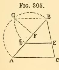
This may be constructed thus: Describe a semicircle on A B as a diameter. From B set off  $B F = \frac{m}{m+n} \cdot B A$ . At F erect a perpendicular meeting the semicircle at G. Set off B G from B to D. D is the starting-point of the division-
