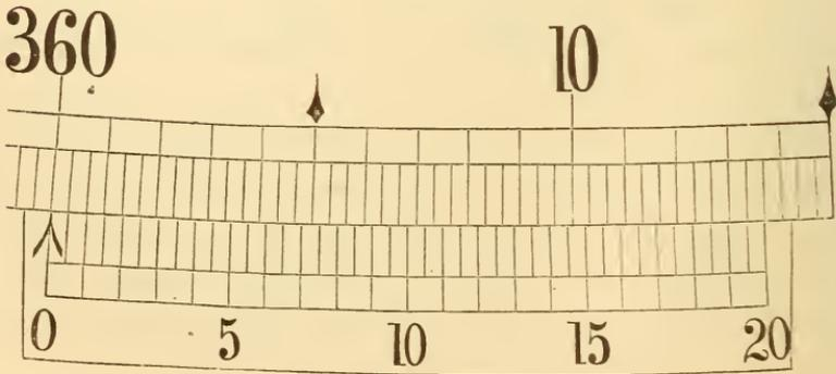
space on the vernier will be  $= \frac{41 \times 20'}{40} = 20\frac{1}{2}'$ , and the vernier will therefore read to  $20\frac{1}{2}' - 20' = 30''$ . It will be retrograde. In Fig. 223 the reading is  $360^\circ$ , or  $0^\circ$ ; and it will be seen that the
