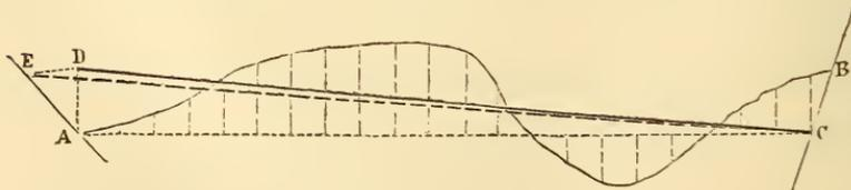
ning a guess-line, A C, Fig. 303, across the bends of the fence which crooks from A to B, measuring offsets to the bends on each
