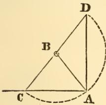
**Problem 3.** *To erect a perpendicular to an inaccessible line, at a given point of it.*
