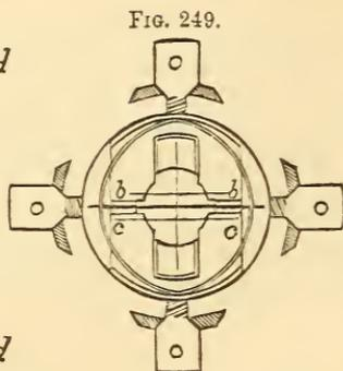
of the rod will be intercepted between the stadia wires, and that the greater the distance at which the rod is held, the longer will be the space on the rod intercepted by the stadia wires.
