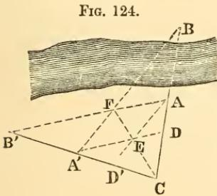
**156. By Transversals.** Set a stake, C, in the alinement of B A; a second, D, at any convenient point; a third, E, in the line CD; and a fourth, F, at the intersection of the aline-
