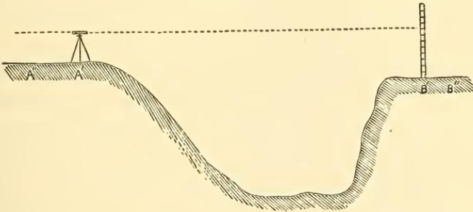
reading. The difference of the reading and of the height of the cross-hairs gives a difference of height of A and B. Then set up at B, and observe to A, similarly. A new difference of height is obtained. The mean of these two is the correct one.
