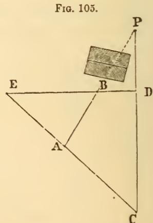
the line of EA; in which case the new distances, CA and CD, will alone require to be measured.
