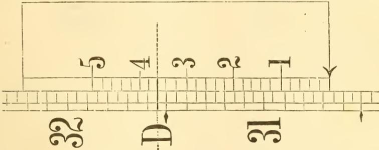
nier, and divided into 25 equal parts, each of which is therefore  $= \frac{24 \times .05}{25} = .048$  inch, and is shorter than a division of the scale by  $.050 - .048 = .002$ , or two thousandths of an inch, a twenty-fifth part of a division on the scale, to which minuteness the vernier can therefore read. The reading in the figure is  $30.686$  ( $30.65$  by the scale and  $.036$  by the vernier), the dotted line marked D showing where the coincidence takes place.
