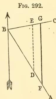
**415. To part off a Quadrilateral.** Let it be required to part off, by a line running in a given direction, a quadrilateral from a field in which are given the side  $AB$ , and the directions of the two other sides running from  $A$  and from  $B$ .
