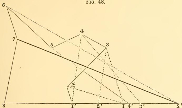
75. *General Rule.* When the given figure has many sides, with angles sometimes salient and sometimes re-entering, the operations of reduction are very liable to errors if the draughtsman attempts to reason out each step. All difficulties, however, will be removed by the following *General Rule*:
