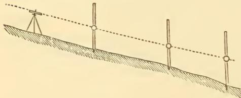
For example, suppose the horizontal distance from A to B is 1,200 feet, and that B is 16·8 feet higher than A. The rise per hundred feet from A is 1·4 foot. Beginning at A, set stakes at every hundred feet, so that the top of each one is 1·4 foot higher than the preceding one.
