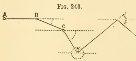
cessive portions of a line (such as a road, the boundaries of a farm, etc.), so as to read off on the instrument, at each station, the angle which each line makes—not with the pre-
