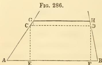
**409.** When the field is given by bearings, deduce from them the angles at  $A$  and  $B$ . The required sides will then be given by these formulas :
