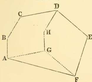
and bearing can be found as in Case 1. Then the triangle  $AGF$  may be treated like the triangle  $AEF$  in the last article, to obtain the length of  $AG = CD$ , and the bearing of  $FA$ .
