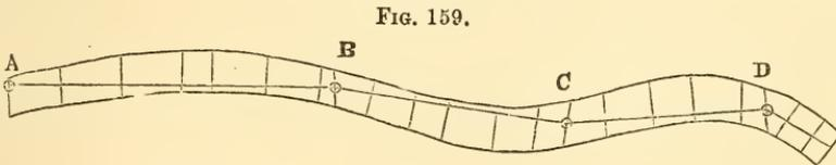
which can be most conveniently measured in the road, and measure offsets on each side to the outside of the road.
