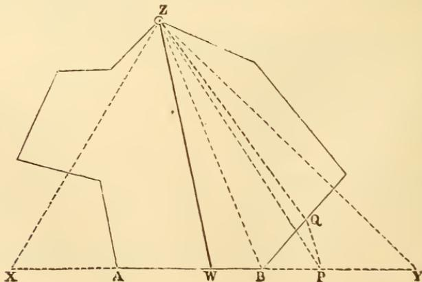
**451. By Lines starting from an Angle.** Produce one side,  $AB$ , of the given polygon, both ways, and reduce the polygon to a single equivalent triangle,  $XYZ$ . Then divide the base,  $XY$ , in the required ratio, as at  $W$ , and draw  $ZW$ , which will be the division-line desired. In this figure the polygon is divided into two equivalent parts.
