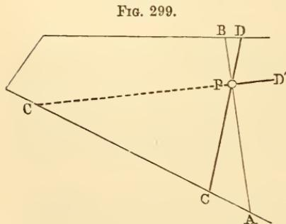
a field a certain area by a line passing through a given point  $P$  within the field. Run a guess-line  $AB$  through  $P$ . Calculate the area which it parts off. Call the difference between it and the required area =  $d$ . Let  $CD$  be the desired line of division, and let  $P$  represent the angle,  $APC$  or  $BPD$ , which it makes with the given line. Obtain the angles  $PAC = A$ , and  $PBD = B$ , either by measurement, or by de-
