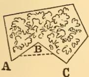
If any angle of the field is re-entering, as at B in the figure, measure a tie-line across the salient angle A B C.
