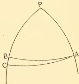
To find the distance C B, when the latitude of the starting-point A, and the distance A C are known.
