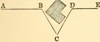
$60^\circ$  from CD prolonged, and the new direction will be in the line of AB prolonged. This method requires the measurement of one angle less than the preceding.
