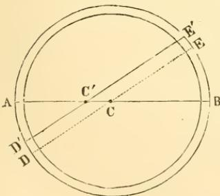
error of *eccentricity*, arising from the center of the axis which carries the upper circle (and with which it and its index-pointers
