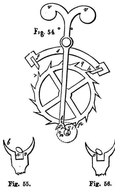
This latter construction will be seen to only differ from that previously described in the number of teeth that are included between the impulse and locking pallets; the action is identically the same as in the first escapement in 1791, and neither of these two varieties can be considered an improvement on it; in both the main causes of irregularity of the Robin escapement are retained as we shall proceed to show.
