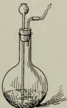
Fig. 35.—Marsh's test for arsenic.
